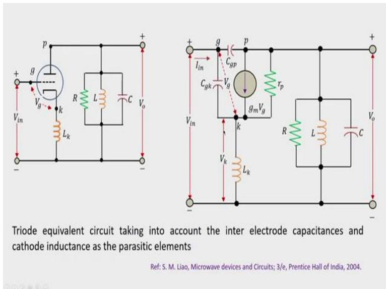
Now, if we analyze this circuit, we can write first of all  $C_{gp}$  the capacitance between gate and plate. This is much less compared to  $C_{gk}$ , the capacitance between grid and cathode. And also  $\omega L_k$  the reactance provided by this parasitic inductance is much less compared to  $1/\omega C_{gk}$ . So these are true for practical vacuum tubes when operated at higher frequencies.
