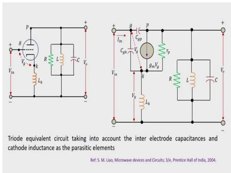
So, we will try to understand these two effects with an example considering a conventional triode. So here we consider a triode which has a cathode which emits an electron and this anode which is maintained at a higher potential this potential difference between this cathode and anode accelerates the electrons, and finally they are collected at the anode, and this constitutes a current.
