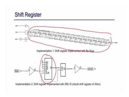
So, if you just do this so what is happening the implementation one is going to be mapped into the normal flip flops which is in the CLV's and that will be connected right it is a big chain of registers where as the implementation two because it has does not have any reset pin it can be mapped to the dedicated shift register right.
