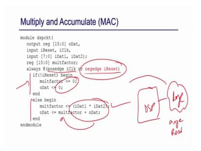
For example in this multiplier I have to do this multiply and add this is MAC, multiply and then you just add it right that is what I am doing here, but I have a asynchronous reset right. So, this is posedge of clock or negative edge of ireset. So, this is asynchronous right.
