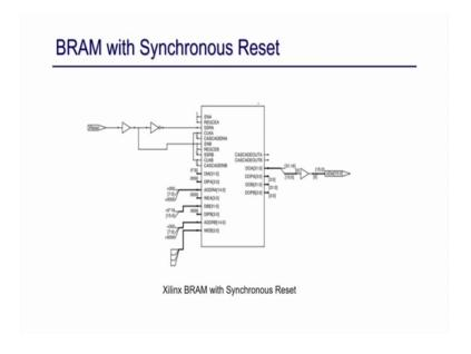
Because this is nothing, but a memory just I am adding memory operation I just storing some memory reading memory and writing memory right. So, so I have just inferred a b RAM Whereas if it is asynchronous reset I cannot infer a b RAM and everything map into to LUT's right the memory and this slices and CLV's and you can see the kind of
