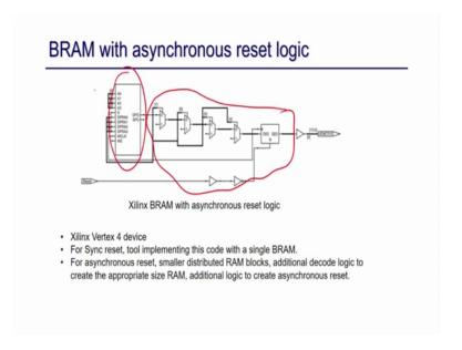
So, here is that extra logic is showing just us to do the asynchronous reset part. So, this is that small RAM and this is the asynchronous reset part which actually resetting that particular output ok. So, this is something give you a very fare idea how that asynchronous in reset impact in BRAM inference ok.
