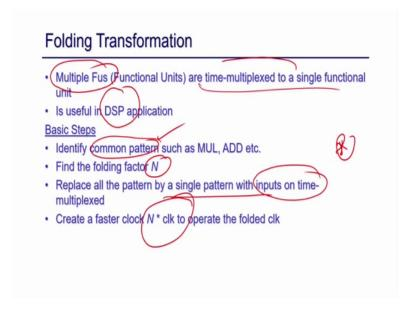
And this fold folding transformation usually apply for this complex operations like multiplier and is basically time multiplex. So, the inputs are time multiplex and it is very useful for DSP application where actually you try to input maximum DSP, DSP in the sense DSP is a specific component in FGPA how which actually can do multiplication very first and it also have some adder and accumulation option pre adder as well as accumulation option.
