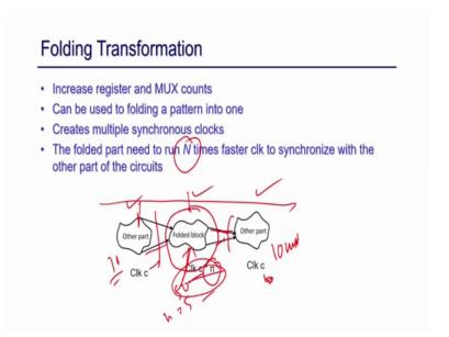
So, the important factor is that here. So, suppose this is the your folded structure right, but this is not the only component of your design. So, this is just a part of your design and it is synchronous with the other part of the design ok. So, now, earlier what is happening? Since this all running in parallel or in the series there is no delay 1 clock you going to get the results right.
