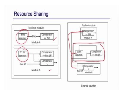
But it is little bit different in the sense that that the structure may not be exactly same. But I can reuse that component it is specifically applicable for counter if you just take this example suppose I have 2 module, where I have 2 counter right 11 bit counter and 8 bit counter.
