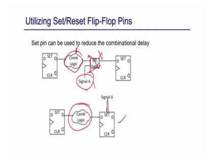
So for example in this particular design so I have this some combinational logic and then there is or gate here and then I have a signal so or with this right. So, if this signal is 1 and this signal is 1 right and it does not matter what is computing here.
