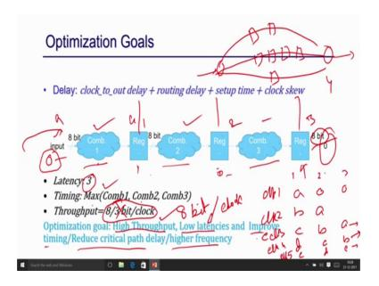
So, let us take an example to understand this fact. So, suppose this is my circuit right. So, there is a computational unit here, the input is coming some computational circuits are here then there is a registers, then there is a another computational circuit and which process this data and output stored in this registers and again this computational unit and then this final results is stored in the register right.
