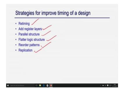
So, there are several techniques and very widely used techniques one of them is retiming, the next technique is add register layers then we can also do the paralyze some structures, flatter logic structures, reorder paths or replication right. So, these are the all kind of techniques that is are applying to your timing. So, we are going to discuss them separately ok.
