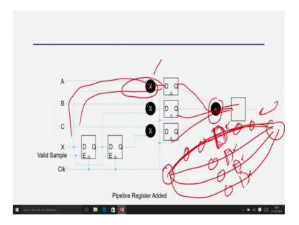
Extra layer here. So, that is what I have done here. So, that the critical path is now the layd of the maximum of one multiplier right. So, this has one this path has only one register adder, but this paths have one multiplier and usually multiplier is more complex than adder. So, the critical path will be determined by the delay of this multiplier.
