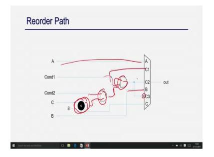
So, if you just see the hardware. So, if condition 1 is true I am going to choose A. If condition 1 is false and condition 2 is true plus C less than 8, this is C less than and this through output and then this will then I am going to choose B right.
