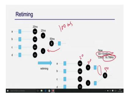
The maximum delay of the circuit is 100 nanosecond here what I did? I just moved this register here right. So, I just moved this register to here. So, now, what will be the maximum delay? So, this is something 20, this is 20, this is 50 and there are other delay. So, maximum will be 60 right 50 plus some other factor. So, there are 60 right. So, you are going to achieve more clock right 16.7 megahertz.
