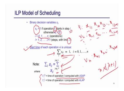
So, for our ILP modelling of scheduling we are going to use a variable x i l ok. So, what does it mean x i l is one means variable operations V i start at time step l right. So, x i l is equal to 1, if that particular operations talk time of that particular operation V i is l otherwise it is 0 right. So, if we just assume you have a operation it is a V l to V n the operations are V l to o V n and say time limit is lambda then your lambda can be 1, 2 lambda plus 1.
