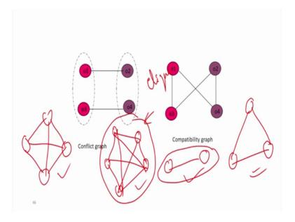
Similarly I can construct a compatibility graph what does it means which operations are compatible to each other level they can be shared a same resource ok. So, to draw the
