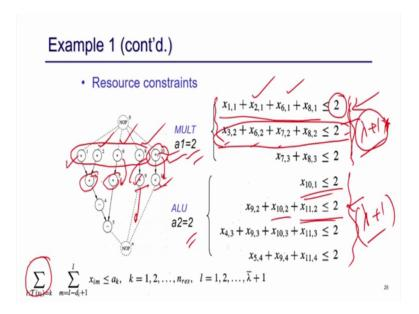
So, this is the set of constant for precedence now, if I assume that I have multiplier two multiply on to ALU I have to put constant for multiplier and as also constant for this ALU right. So, and the constant is given by this so this is what the type. So, for multiple types since these are all single cycle I do not have that consider a multiple step I have just consider to present state.
