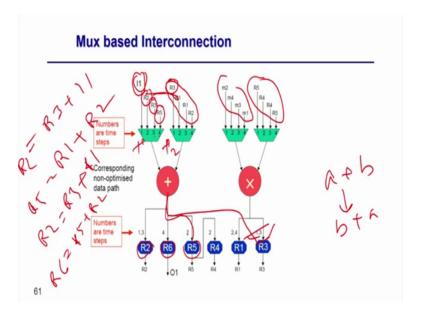
And here what kind of optimization is possible although actually that commutative operations can be applied here to improve that for this mux size. So, if you just see here so for example, say time step 1 this I 1 is coming time step 2 r 2 is coming, and time step 3 r 3 is coming, and time step 4 r 5 is coming and similarly here r 3, r 1, and r 2 right.
