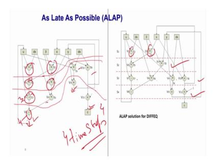
So, here the algorithm is I mean similar to that ASAP algorithm what it does it try to schedule the operation as late as possible. So, if you go into this we try start from the output so those operations are generating output right this, this, these operation. So, they are generating so they has to schedule in the last step right after that you do not schedule in the last step you need one more time step it.
