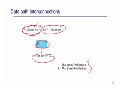
So, here as I mentioned that after this register allocation binding and function you need reminding I know this operation is map to this and these are the set of inputs possible here, now these are the set of input possible here and I have to make some connection here interconnections so that this kind of operations can be executed.
