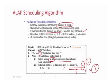
So, similarly we have this as late as possible is just the opposite person of this s and as soon as possible algorithm over here we are going to try to delay the operation as late as possible right. So, here we will have a given a latency bound; that means, I want to schedule this particular thing in say k time step, or say 4 time step and whether this is a feasible or not. So, if the latency is given too small then they exist solution that we are going to get may not feasible right.
