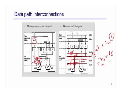
So, in bus based architecture what happened for each register there is a output bus right for register 1 there is a bus, for register 2 there is a output bus, for register 3 is output bus and if this r 1 is connected to this I will just added connection here and added switch here.
