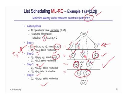
So, in this example you can see suppose this is my that differential equation solver again and I assume that my d 1 equal to 1 that is all are single cycle operations and I have 2 multiplier, and 2 adder so I have 2 multiplier, and 2 adder.
