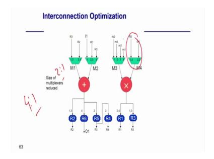
Because I am now actually to only two possible input here also I mean one of the input readings. So, similarly I can do the same thing for this this mux which I am not going to need to discuss detail and just reduce the size. So, this is the kind of optimization we can do in the data path generation using this commutative operations and all we can actually reduce the mux size which will also give you the what are area requirement of the whole design will be less.
