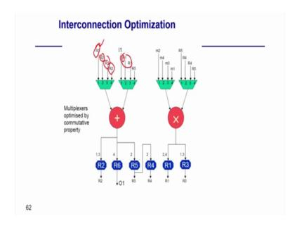
So, now you can see initially I have this r 1, r 2, r 3, r 5 and if I just move in this swap this r 2 and r 1 what will happen you can see r 2 comes here, and r 1 comes here, and now I have 2 r 1 right. So, I can select this r 1, and r 1, r 2, r 1 so, I can reduce the mux size, so I am only 2 possibly, 3 possibly input r so there r 2, r 3 also.
