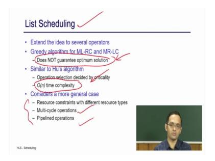
So, now we will move into this list scheduling algorithm which is nothing, but then this that is another person of this Hu's algorithm. Here this is also this ah, but here you can have multiple type of resource instead of only multiplier or on only adder you can a multiplier adder subtract all kind of resource can be available and your operations can be pipeline, multi cycle, or other various is also possible so and we have some resource constant right.
