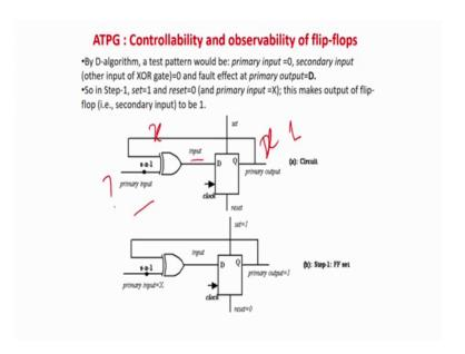
So, you can do that so, the same thing they have shown, I am just taking as a simple example to see if we have a set reset what will be the advantage. Like in this case, it is a stuck at one problem fault. So, you will require a 0 over here. So, if you have a 0 over here, basically, then maybe I assume that it is a xor gate. So, if I assume that I want I
