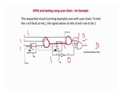
So now what now basically we are going to see with an example how scan has to be done. So, we are taking a very simple circuit, and we are taking a stuck at 0 point over
