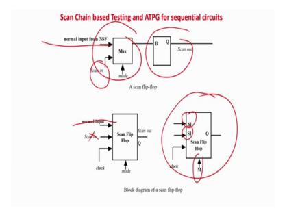
So now let us look at the typical architecture of this scan. So, what is happens basically we have a d flip flop we have a multiplexer. This is the normal input, and if this scanning, scan it can be a primary input or it can be the input from the other flip flop which is previous to that in the chain.
