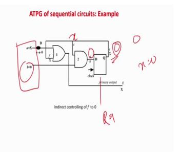
Now, how do you do it? So, of course, I require a 0 over here, that is my primary requirement I think where a 0 on the output of the few. So, how can I do? So, obviously, in sequential circuits, you cannot test by one test pattern. Like in combinational circuit, it was very obvious and also you have seen by example, that for a given stuck at fault you require maximum one test pattern to test it.
