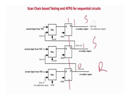
So, basically what I will have to do, either I have to make that set reset. So, in this case 6 lines will be output, but you can set I am resetting one mode. Because this is this is set, this is set, and this is the set. So, if they are 1 2 3 4 5 6 lines directly the output you can do it in one clock pulse. By making this set equal to 1, set equal to 1, and here reset equal to 1, your job will be done.
