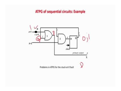
So, the idealized a stuck at 0 I put a 1 over here. Now I require a 0 over here, and the value will be propagated so, if it is 0. So, the value will be a d over here, normal one faulty 0, and this d will be propagated over it. That is what is the requirement. This is sensitized, the value is propagated over here, and the value of 0 here is the justification, that is done.
