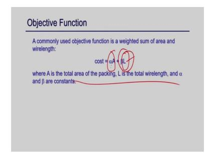
And also a; so, in general the objective function is the minimization area plus objective length right A is the area and B is the L is the length and alpha and fera beta is some constraint factor right this is overall objective of floorplanning ok. And this wire in the estimation is something because now I do not have the exact placement. So, how we can how can I estimate the wire length is basically just the distance between in this.
