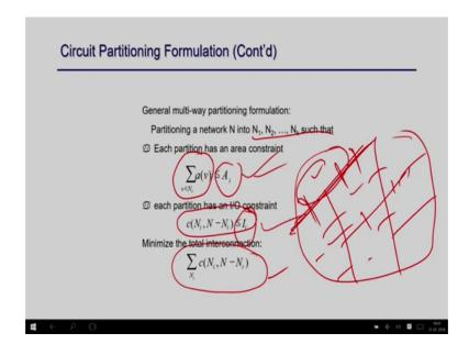
Such that each component area there may be some area requirement that each component area is within the permutable size and the number of edge crossing there the cut size is
