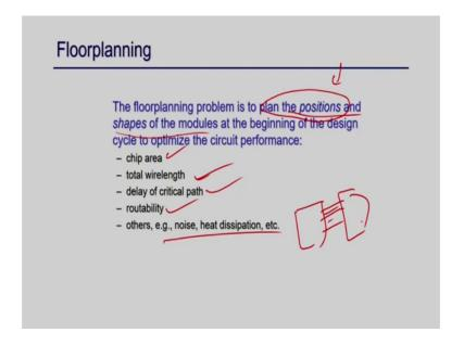
So, if you just move on so, floorplanning is the problem of positions; finding the plan the position not exact plan fixing the block that is important because I am just planning the positions right and then shape is finalized at the beginning of the design right, where your object will be optimize the area, total wire length also. Because you try to because I know that now what is the connection between two component based because that is given by the cut size.
