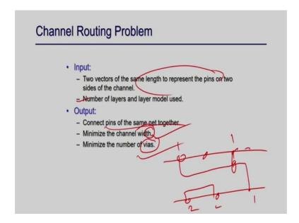
And your channel routing problem is as I mentioned there are two vector of same length pins are there the pins are given of two side of this channel. And there the number of layer is given whether is a VH model, HV model, HV H model and those that is also given and you actually and the pin number. So, this is 1, this is 1 and this is 1; that means, you have to make the connection like this right.
