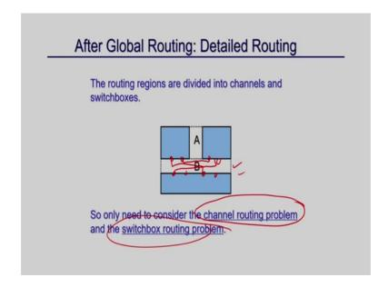
And then the finally after this is a pin assignment, pin assignment something you this then final as a mention here after that you actually make the pin assignment. Because what is happening here once you finalize one particular channel you know how many pin are there how many pins are there right.
