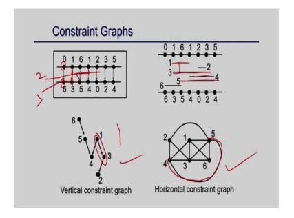
So, you can see here there can be various constraint right. So, if you have a this and this; that means, they cannot be put in the same track because they are overlapping. So, this is horizontal constraint we can construct a constraint graph like this for example, this 5 this
