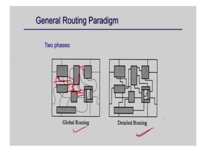
First is global routing the second is the detailed routing so; that means, what I just decide keep from this connection to this connection this will go through this part of the circuit and through this part of the circuit; this is I decide not
