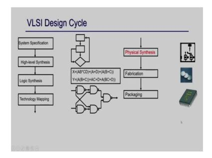
So, if you look into VLSI design cycles we have seen that we already discussed that it start from some specification, then it go through high level synthesis, logic synthesis, technology mapping and then physical synthesis fabrication and packaging right. And we already have discussed about high level synthesis, logic synthesis and technology mapping.
