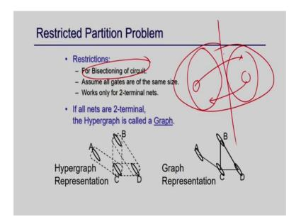
So, basically you try to make the circuit into by 2 right and the idea is that you start with the initial any arbitrary partitioning; you take a just any arbitrary partition, you try to bi partition the circuit and then in each iteration you try to take a node here and you try to (Refer Time: 24:20) here and you move it here and you try to move it here.
