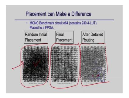
This is what is the objective or the placement step. So, we can see there is a some random initial placement what is generated by floorplan; effectively the placement looks like this right this is just the snapshot of the your layout. But you can make some modification you see the number of wire length become very less here right.
