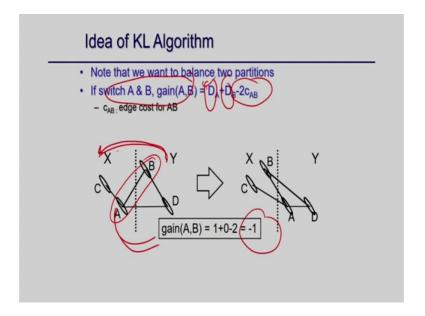
And then this cost of D B. So, that we are moving A from this side, B from this side cost of moving this plus this that will be your gain, minus the interconnection between these two node right there is a interconnection between this node. Because they are a actually counting two times here right; so, you have just remove it. So, they will be always remain the same. So, that is what is your actual switching between two nodes is the overall gain right.
