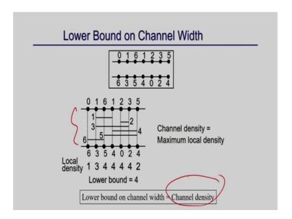
And using that actually you can solve your problem and you can actually identify the number of minimum track required using some logic also it is the channel density.
