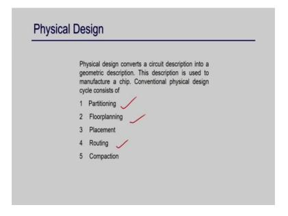
So, let us go into this physical design steps. So, in physical design the sub steps are partitioning, floor planning, placement, routing and final the compaction. So, we are going to talk about this partitioning, floorplanning, placement and routing what is then what is the objective of a sub steps right?.
