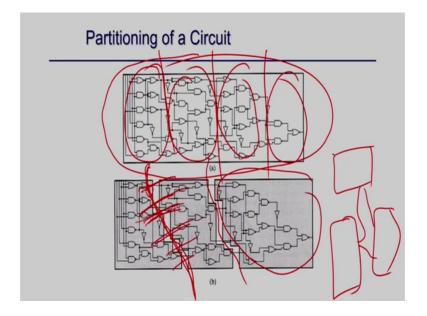
So, whenever you have big circuit or objective is finally, place all this for example, here this is a big circuit is given our objective is to place all this gates in a chip area in in minimum possible area. So, one approach is that you take one by one and you place them which is not physically possible that I have already discuss. So, basic idea is a process partition your design right.
