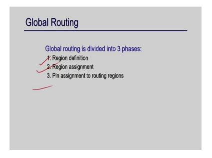
Basically the global routing has three phase that the region definition, region assignment and pin assignment ok.
