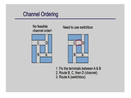
So, then in that sometime they basically you need a switch box. So, why you need a switch box? You can actually define some portion of the circuit which is basically switch box and that. So, that you can actually reduce a dependency and you can actually make it channel order ok.
