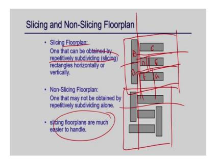
So, and also there is another concept here is sliceable non sliceable floorplan; what is that? Sliceable floorplan is something; so, you finalize your as per your aspect ratio and finalize your block height and width right and then you place them. So, after placing one is one is sliceable means what? You can actually can obtain the your floorplan can be
