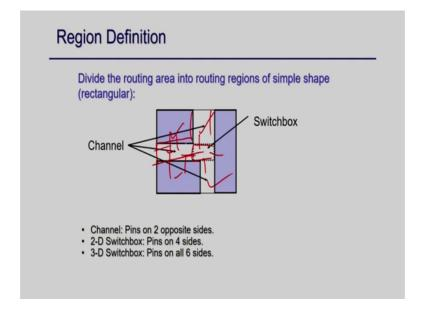
So, what is the region definition? So, basically when your channel between; So, there is a part of the circuit which is basically between two blocks which is called channel. So, this is also a channel and you have this is also a channel and this is a switchbox because this has a multiple (Refer Time: 55:19) data can come from this side, this side, this side as
