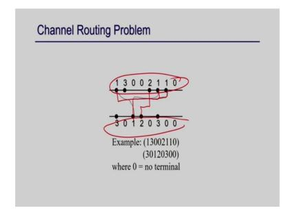
As I mention. an example; so, this is 1, this is 1, I want to make a connection like this right. Similarly this is 2, this is 2 means I have to make a connection like this. So, this is what is how the problem is given it is as given this set and this set right this is and you have given whether it is a VH; HV on this and you have to solve this right.
