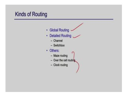
So, the routing has two types first is global routing, the second is detailed routing and the other kind of techniques are there like clock routing or cell routing maze routing which I will not cover here. So, primary; so, initially what is happening here; so, here is this things is there the routing is has two phase.
