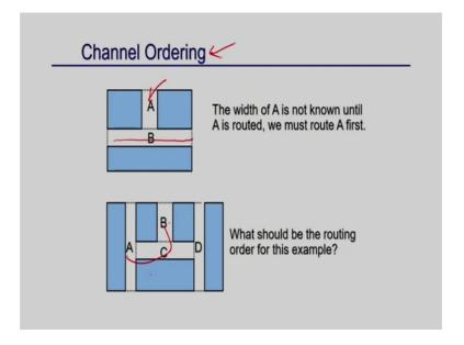
So, as I mention then again the one important concepts that is channel routing channel ordering. So, suppose; so, I have to decide the width of this; so, if you I do not know that width of A; I cannot decide the way that total width of this B right. So, I have to; so, I have to decide A first then B right so, but in some synergy may circular dependency would have to do B, then you have to do C if you are to do C A and something like this.
