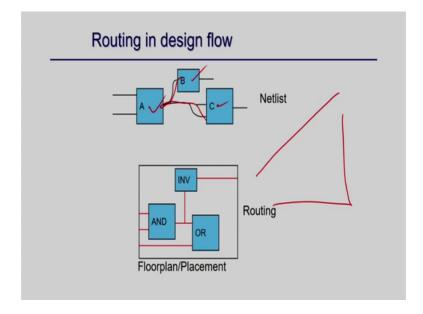
It has to be go vertically, or horizontally you have track vertical and horizontal track you have to make the connection through this right. So, ah; so, the routing problem is that is after floorplanning or placement.
