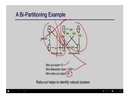
So, now here as I mentioned that formulation is that I want to make it find a cut such that between two partition either may have it will be minimum cut the number of crossing is less or the bisection have exactly bisections at the both component has equal number element with minimum number of cut here or I can have a minimum cut ratio.
