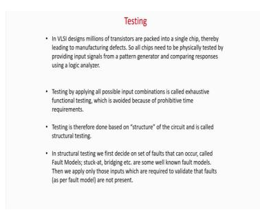
Now testing; so already I have told you in in VLSI design millions of transistors packed into a single chip. So, they have lot of manufacturing defects. So, as the yield is not very high, not like 99 percent plus, which is the generally case for traditional engineering devices like electric fan and iron. So, we all know how to design a fan and a iron. So, once you design it 99.9 present surety is they will do there functionality.
