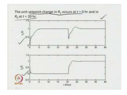
Then with the controllers in the loops, the performances of the TITO system are obtained as shown over here, the first loop has got a set point change, unit set point change at time T equal to 0 hour. And the second loop has got a unit set point change, at time T equal to 20 hours, then the responses of the two loops are shown over here, the upper loop response is given here, and the second loop is giving a time response of this form.
