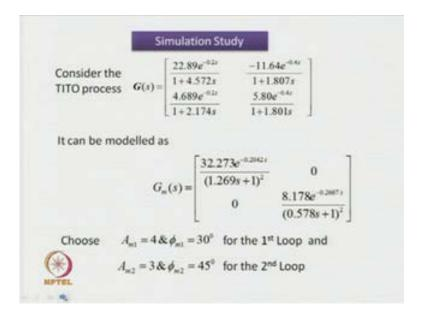
Let us consider a TITO process dynamics, given by this transfer function matrix G (s), which has got four elements and each four elements are nothing but, the first order plus dead time representation. So, we have got enough interaction in the TITO system, the two loops of the TITO systems have got significant interactions; now the dynamics of the TITO process, with the help of proper identification procedures, may be obtained in this form.
