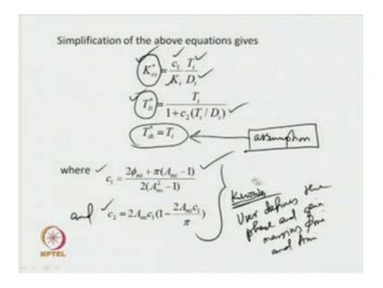
And those explicit expressions are obtained as K c i star is equal to c 1 upon K i T i upon D I, T I i star is equal to T i upon 1 plus c 2 times T i upon D I; and already we know that T d i star is equal to T I, this is the assumption we made at the beginning. So, with this assumption, we proceeded and we have been able to find explicit expressions for the two unknowns of the new PID controllers, K c i star, and T I i star. Now, in the expressions c
