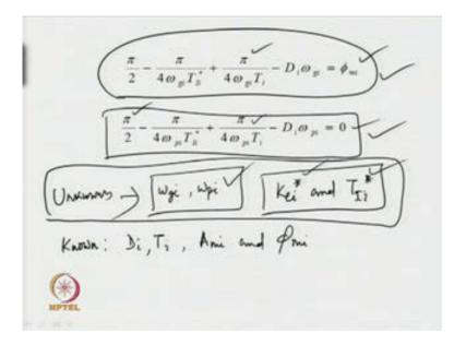
Now, one can substitute the tan inverse function over here, which will result in an expression of this form. So, tan inverse functions are substituted, which results in the expressions pi upon 2 minus pi upon 4 omega g i T I i star plus pi upon 4 omega g i T i minus D i omega g i equal to pi m I, where are we trying to substitute the tan inverse function because, it is very difficult to solve this non-linear equation (Refer Slide Time: 23:35).
