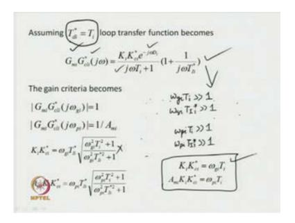
For that for each in analysis, let us assume that T d i star is equal to T i with that assumption, the loop transfer function becomes G m i G c l i star (j omega) is equal to K i K c i star e to the power minus j omega d i upon j omega T i plus 1 times (1 plus 1 upon
