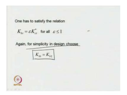
Next, using the same relation I can say K b i is equal to epsilon times K c i star, now epsilon has to be less than 1, and that guarantees that all the parameters of the PID controllers will be positive. So, simply designing the parameters of the new controllers, may not ensure desired control of the TITO system, in that case one must ensure this condition to get all the positive values, all the parameters to be positive.
