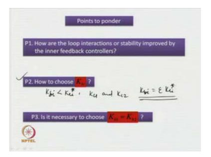
Now, certain points to ponder on this TITO system control are the first point could be how are the loop interactions or stability improved by the inner feedback controllers; inner feedback controllers, enable us to place the poles of the loops, at some desired locations. So, placing the poles of the loops, at some desired locations helps us not only in designing perfect controllers for the system rather that helps also in loop interactions.
