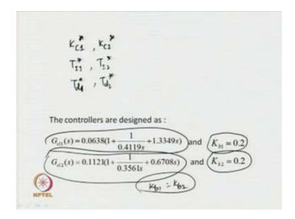
Controller has been designed initially, we get the designed values for K c 1 star, K c 2 star, next T i 1 star, T i 2 star and subsequently T d 1 star, and T d 2 star, then using the relations just, now we had discussed using these relations, the controller parameters of the original controllers are obtained as this, and this. Of course, with the choice of K b 1 is equal to 0.2 and K b 2 is equal to 0.2, as we have said K b 1 is equal to K b 2 enables us for each in design.
