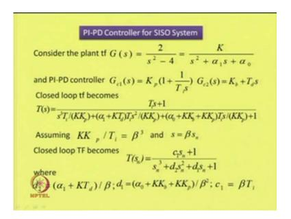
Initially, we shall consider a plant transfer function of the form shown over here, which is having a numerator K and denominator s square plus alpha 1 s plus alpha 0. This all pole transfer function, can assume different form depending on the values of alpha 1 and alpha 0. Now, when alpha 1 becomes 0, we get a second order integrating process, when alpha 1 equal to 0 and alpha 0 equal to 0, we get second order integrating process.
