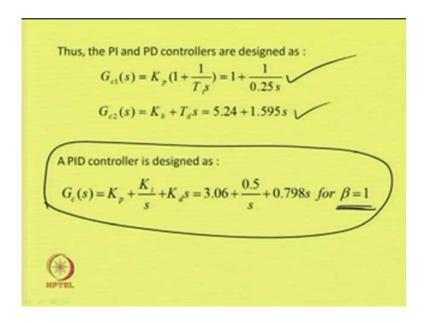
Now, with these values of the PI PD controller, let us see the performance we get from the closed loop system. Thus the PI controller is of this form and the PD controller of this form, for comparison we have also designed a PID controller for beta equal to o1. We can have the same beta, it does not matter respective of any value of beta, it is possible to design a PID controller using standard form.
