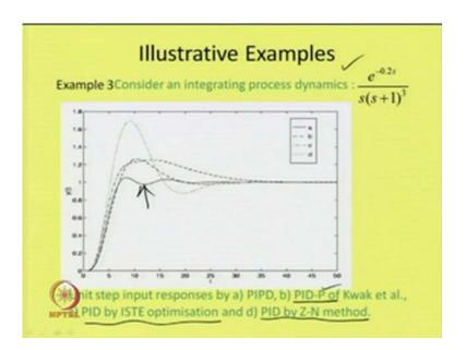
Now, there are some illustrative examples also. Consider an integrating process dynamics, a fourth order integrating process dynamics, for that also the PI PD controller responses given by the solid line is found to be improved one compared to the four parameter PID P control of Kwak et al, PID controller by ISTE optimization and PID controller designed by Ziegler Nichols method.
