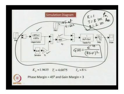
Before that let us see, how the control loop performs with the design values of the K p T i and T d, let us assume the process dynamics to have the form of G s equal to e to the power minus 2 s upon 8 s plus 1 square. So, we have got a process, second order process with repeated poles located at minus 1 upon 8 and with the delay of 2 seconds.
