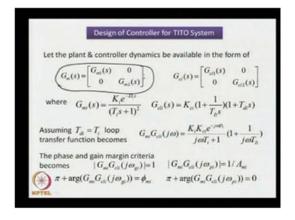
Now, the dynamics of the TITO process is assume to have the form G m s equal 2 G m 1 s and G m 2 s in diagonal of this transfer metrics. So, the TITO process dynamics is given by a transfer function metrics often known as transfer metrics given as G m s equal to G m 1 s 0 0 G m 2 s, we, thus we get a diagonal transfer function metrics for the TITO system. This form of transfer function representation helps us to design conveniently controllers for the system.
