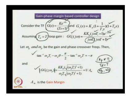
So, attempt will be made first to design a controller series PID controller based on gain and phase margins. The transfer function shown over here G c s shows us a series form of PID controller, where we have got the proportional gain given as K p, and integral time constant given as T i, and derivative time constant given as T d; this is a series form of PID controllers, unlike the parallel form of PID controller, which can be given in the
