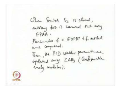
When switch when switch S 2 is closed, then auto tuning test auto tuning test is carried out using of course, FPAA. Then parameters of parameters of a first order plus dead time transfer function model are computed. Then the PID controller parameters parameters
