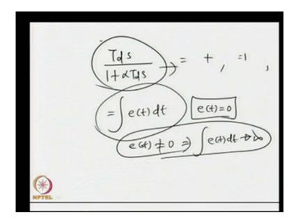
When the error gets integrated over time, but if error is not exactly equal to 0 over time, then this value goes on growing with time and blows up after certain time. So, that gives us a very large value over time. When e t is not equal to 0, integration of e t d t explores may give a very large unacceptable value after some time. This phenomenon is known as integral wind off.
