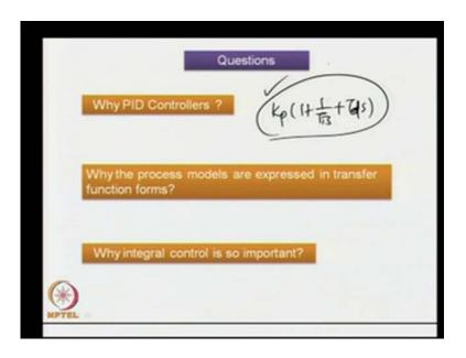
This analog form of controller can be is realized in software and in hardware. Writing a simple program, one can implement the PID controller algorithm. Similarly using analog gadgets, analog electronics or digital electronics, it is easy to implement a PID controller. That is why PID controllers are famous in process industries.
