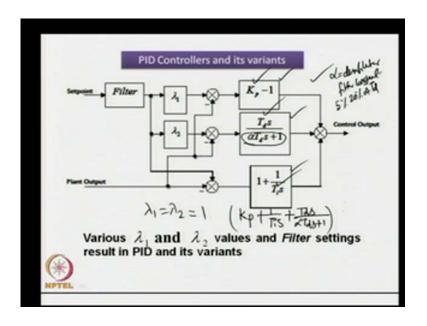
Before that, let us consider the block diagram of a PID controller, which can be given in this form. Here this block gives us the proportional controller, this one as the derivative controller with a derivative filter and this block gives us the integral controller. What is alpha over here? Alpha is often known as the derivative filter constant whose value is
