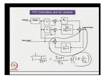
How to avoid that? To avoid that, we can realize that action with the help of a filter
