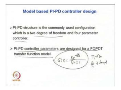
The benefit of using PI-PD controller has been described in one of our previous lectures, now PI-PD structure is the commonly used configuration, which is a two degree of
