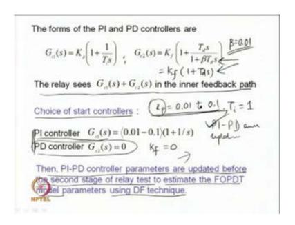
Let, the forms of the PI and PD controllers be G c 1Sis equal to K p times 1 plus 1 upon T i S, and G c 2 S is equal to K f times 1 plus T d S upon 1 plus beta T d S. Normally, beta is chosen a very small value, when beta is equal to 0.01, we can neglect the derivative filter term from mass of sequent analysis. So, G c 2 can be written as K f times 1 plus T d S for analysis for ease in analysis in our subsequent analytical - subsequent dealing of the analytical expressions.
