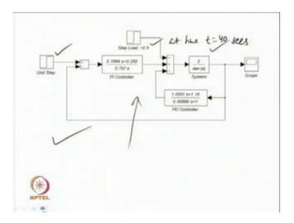
Now, we will we have simulated the PI-PD controller along with the plant in closed loop using unit step input as the reference input, and a static load disturbance of magnitude 0.5 occurring at time T is equal to 40 seconds.
