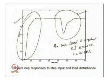
Now, the simulation results obtained from the PID, P PI-PD controller are shown here. The time response for the unit step input is shown in the initial part, whereas the load response is shown in the later part. Again the static load disturbance - static load of magnitude 0.1, please keep in mind of magnitude of magnitude 0.1 occurs at time t equal to 40 seconds. So, the responses are found to be satisfactory.
