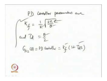
Let me rewrite again the PD controller parameters, so the PD controller parameters are K
