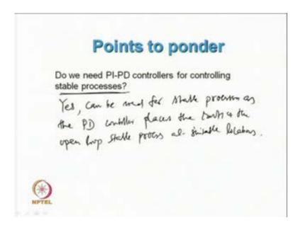
Coming to the points to ponder: Do we need PI-PD controllers for controlling stable processes, yes the PI-PD controllers can be used for stable processes, can be used for stable processes as the PD controller - PD controller basically places the roots of the open loop stable process process, at suitable locations. Also the PI-PD controllers find extensive use in controlling integrating, and unstable processes. It can also be used for controlling stable processes. Thanks.
