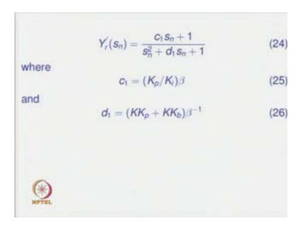
Now, dividing both numerators and denominators by K K i, we can get a second order standard transfer function. So, assuming beta equal to root of K K i further results in a second order standard second order transfer function or second order standard transfer function of the form Y r Y r dash S n is equal to C 1 S n plus 1 divided by S n
