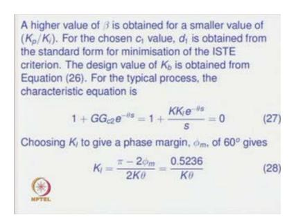
For the typical process now the characteristic equation becomes 1 plus G G c 2 e to the power minus theta s is equal to 1 plus KK l times e to the power minus theta S upon S is equal to 0. Now, choosing K l to give a phase margin of some specified value, suppose phi m phase margin is equal to 60 degree; that condition gives K l or gives an expression for the K l as K l is equal to pi minus two phi m upon two k theta upon substitution of phi m of 60 degree.
