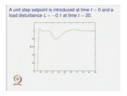
So, when this controller parameters are put, and simulation is carried out simulation of the modified smith predictor structure with the unstable first order plus dead time unstable process is carried out. We do get the response from a unit step set point input, that is introduced at time t equal to zero, and a load disturbance L of magnitude minus 0.1 at time t equal to 20. So, we do get responses corresponding to the set point and disturbance inputs, and the responses are shown over here.
