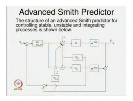
Now the structure has been reproduce, once more where the servo controller or servo tracking controller G c is also connected in parallel with a relay. The main objective of the relay is to identify the dynamics of the real time process. So, once the dynamics of the real time process is obtained, then that is now shown by the transfer function model G m e to the power minus theta m s.
