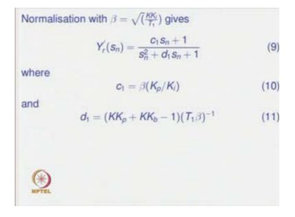
So, basically the dynamics of equation number 8, and equation number nine are not different from each other. Of course, there is a scaling factor, because you are getting a normalized frequency now in place of the normal frequency of operation. So, it will be nearly scaling of the responses, you will have corresponding to this normalized transfer function.
