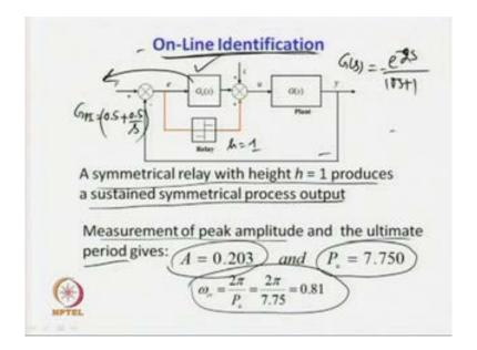
Only thing, you need to do is when you are stimulating this on-line identification scheme, the controller again I am saying use the controller, a PI controller; GPI of magnitude .5 plus 0.5 by s. Let me repeat, because this is very important and relay setting is height equal to 1. Relay height or parameter is set to 1 and the process is the same process, we have been considering in our earlier example; e to the power minus 2 s upon 10 s plus 1.
