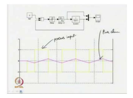
Now, with the use of a relay of course, I have been able to get this sustained oscillatory output shown by the pink color and the yellow one shows us, the output from the relay or process input process input during the auto tuning test now or identification test.
