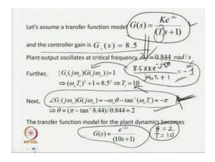
So, that way we have got the expression 8.5 times K e to the power minus theta s upon T1 s plus 1, as the loop gain and the loop gain has to be minus 1, to obtain sustained oscillatory output. So, using this expression when the magnitudes of these expressions are equated; magnitudes means, when the magnitudes of both sides of these expressions
