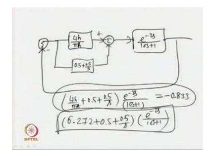
Now, when one uses the loop gain or when I write the loop gain equation for this as, this is equated to minus 0.833 8 3 3 and carry on with the analysis; that means, find explicit expressions for time delay and time constant associated with the transfer function model. Then, the the parameters can be estimated accurately. Let us see, how we can find those T. So, what will be done now in this analysis now?
