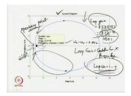
The controller gain is 8.5. The operating point is push to a point of minus 1 plus j 0 and the loop gain is equal to minus 1. What is that loop gain now? Loop gain is nothing but, the controller gain times the process dynamics.
