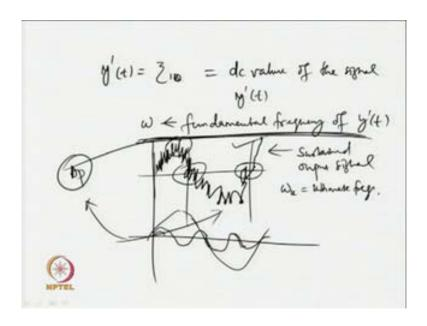
Now, when k equal to zero when k equal to zero what will happen, y prime t will be equal to simply your xi 1 k and k is 0. So, will get a constant of the form xi 1 0. So, this gives the d c value of the signal y prime t and rest of the components or terms will have will have certain frequency where the signal is assume to have a frequency of magnitude omega. So, omega is the fundamental frequency of y dash t.
