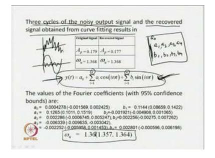
Now, what has been done, how we have obtain three cycles of the noisy output signal is plotted over here, if you see almost three cycles of noisy output signal is plotted along with that, the recoverd signal obtained from curve fitting also provided, how do you recover this one, it is all about simply data fitting. So, given a set of data, you try to feed it with the expression, we have obtained for the curve fitting.
