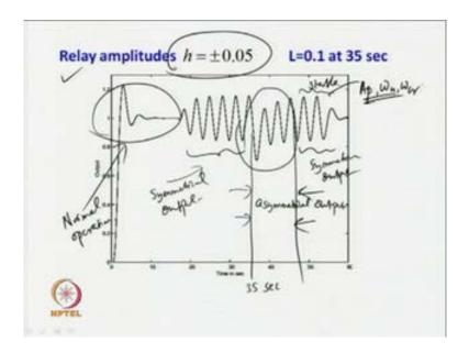
Now, for this unstable sorry for this integrating process, the static load is injected at time T equal to thirty five seconds and let us see the type of waveform will expect during the auto tuning test. So, when the static load disturbance occurs at thirty five seconds then the output is having asymmetrical output for a certain duration. So, this is the duration during which we have got asymmetrical output and apart from this duration, we do have symmetrical output from the process.
