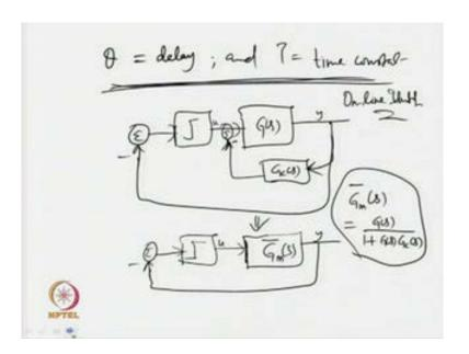
Those are the 2 remaining parameters known as theta, time delay and T, time constant. So, how to estimate the 2 parameters now? For that, we have to have analysis of the closed loop relay control system. So, the relay is connected to the plant and now, the plant is having some inner feedback controller. This is the controller, because we are considering online identification scheme. online identification. So, this is the equivalent representation of the online identification scheme.
