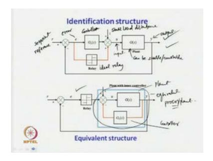
The scheme for the identification is given or shown as  $\frac{1}{1}$  shown over here. Now, R is the set point or reference input, G(c) is the controller connected in parallel with the relay; a relay is assumed to be an ideal relay. I is the static load disturbance and G(s) is the plant or process under relay control or during the relay feedback test. Now, the plant can be stable or unstable, and the remaining signal shown in this block diagram are y is the
