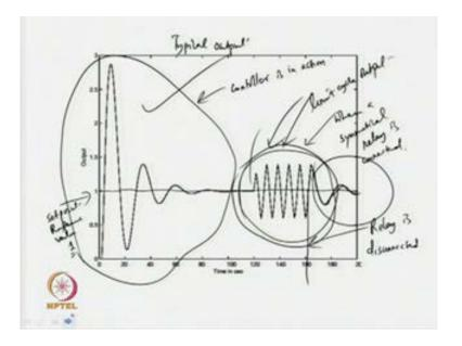
Now, some typical typical output from the plant is shown; where the plant, this part of the output shows that, the controller is in action is in action and normal operation of the controlled system is on or is going on. Now, when the relay is invoked or connected at time T equal to 120 seconds, then the output assumes this form. Now, when the output assumes this form as you can see. If you draw a line like this, the output is symmetrical
