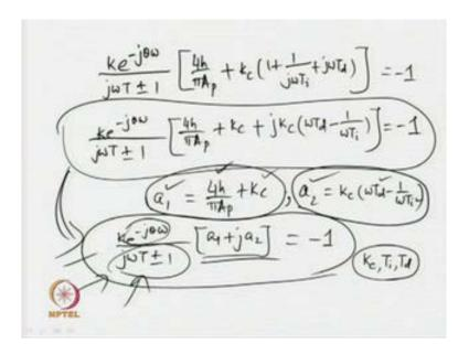
If you carefully look at the two constants a1, and a2; you see it contains not only the gain of the relay, it contains parameters of the controllers as well. So, Kc, Ti and Td, omega is measured; omega is obtained from the limit cycle output, but how to how to choose Kc, Ti, and Td during the relay experiment or test. That possesses a challenge.
