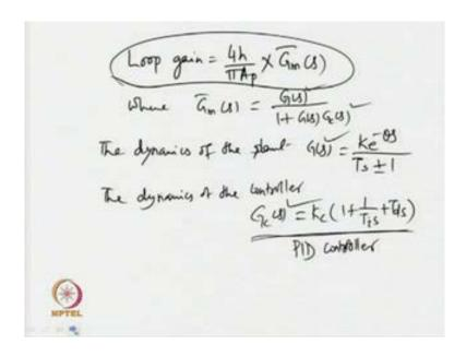
So, thus we have found that, the loop gain is equal to gain of the relay which is 4 h by pi Ap times Gm bar s, where Gm bar s is found to be G(s) upon 1 plus G(s) and Gc(s).
