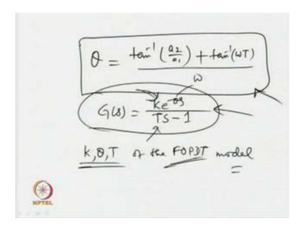
So, like the earlier case; now finally, I can have this minus pi minus pi of both sides cancelled out; giving me theta is equal to theta is equal to tan inverse a2 by a1 plus tan inverse omega T divided by omega. So, when the dynamics is having unstable pole, then at that time please make use of the two formula; we have derived the T this one and the
