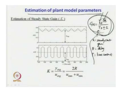
Now, how can we estimate the plant model parameters? Assuming some transfer function model of the form G(s) is equal to K e to the power minus theta s upon T s plus minus 1 for the dynamics of the plant. We find that, the transfer function model for the
