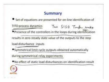
So, what we have studied here, set of analytical expressions are presented discussed for on-line identification of the TITO process dynamics. So, two SISO transfer function models, transfer matrix are obtained. Now, presence of the controllers in the loops
