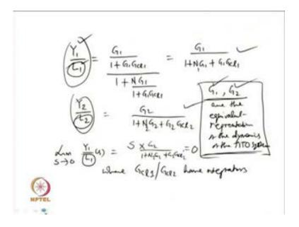
Now, also I can get the relation between the output to the static load disturbances in the form of Y 1 upon L 1 is equal to G 1 upon 1 plus G 1 G cl1 upon 1 plus N G 1 upon 1 plus G 1 G cl1. What I mean by that, let us find the transfer function between Y 1 to L 1. Then assuming R 1 to be 0 that time, R 2 to be 0 that time for the upper case, when the TITO process or dynamics is assumed to have decoupled dynamics, that that time the
