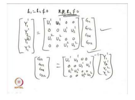
So, when I write this in the form of G 1 1, G 1 2, G 2 1, G 2 2 is equal to, take this to the left hand side. So, you will have the inversion now, matrix inversion U 1 1, U 2 1, 0, 0, 0, 0, U 1 1, U 2 1, then U 1 2, U 2 2, 0, 0, 0, 0, U 1 2, U 2 2 inverse times Y 1 1, Y 2 1, Y 1 2, Y 2 2. So, this is how get? You get. So, I find the matrix inversion which comes out to be of this form; times it will be your y 1 1, y 2 1, and y 1 2, y 2 2. So, this is how you get the expression for G now.
