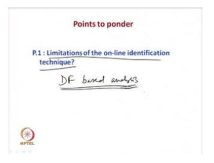
Now, what are the limitations of the on-line identification technique - one major limitation associated with this technique is that, we are using the describing function based analysis. Now, the describing function does not yield more number of inequalities, as far as analysis based on describing function is concerned. Therefore, one has to assume the transfer function models. The SISO transfer function models having less number of unknowns that is all, thank you.
