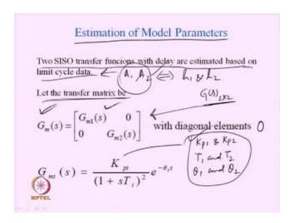
Now, the transfer functions have got the parameters steady state gains given by K P 1, and K P 2 for the two loops, and the time constants given by T 1 and T 2 for the two loops, and the delays given by theta 1, and theta 2 for the two loops.
