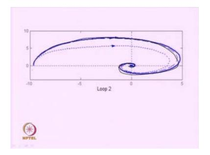
Similarly, for the loop 2 rather, we have seen that the nyquist plot for the original system dynamics, and the identified system dynamics are very much in agreement. And it shows that, the identified technique or the identification technique is quite efficient.
