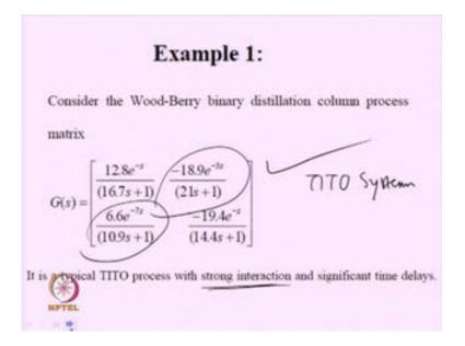
Now, I will go to one example. Consider this example, which has got a TITO transfer function matrix of this form. These two shows that, the TITO system has got enough loop interactions. So, the TITO system is subjected to significant or strong interaction between the loops.
