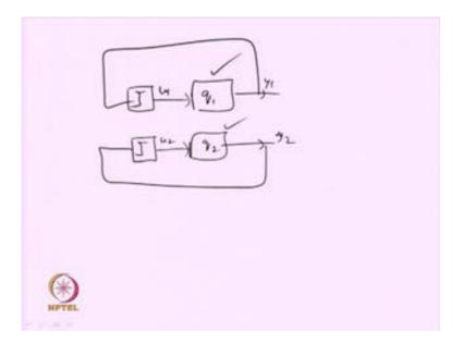
Given in the form of u 1, q 1, y 1, and u 2, q 2, y 2. So, whole dynamics - the dynamics the closed loop system, I have shown over here can equivalently be represented in this form. And if that is so, if that is possible in that case what happens. Now, one can easily employ a relay, here to identify the dynamics of the two sub systems.
