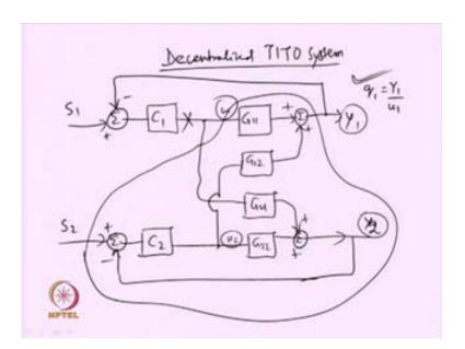
Now, allow me please to write down the T I decentralized control system once more, decentralized TITO system, where I shall describe the TITO system dynamics in the form of G 1 1, G 1 2, G 2 1, and G 2 2. Again we have got the output from the blocks
