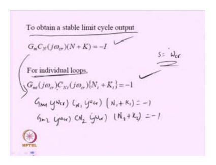
Now G mi of j omega c r times C Ni(j omega c r) times N i plus K i is equal to minus 1 or minus sorry, this will be minus for the individual loops it will be minus 1. That means, I can write this as G m1(j omega c r) C C N 1. Please keep in mind j omega c r times N 1 plus K 1 is equal to minus 1. Similarly, G m2(j omega c r) C N 2(j omega c r) N 2 plus K 2 will be equal to minus 1.
