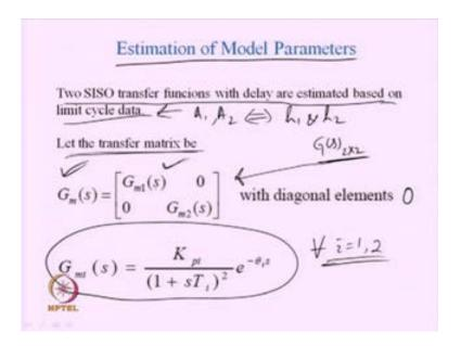
So, with the introduction of K C N, and N in diagonal form particularly, it becomes very easy to get the dynamic equation for the TITO system under relay control. So now, we shall describe in detail the estimation technique, when the relay test is performed. So,
