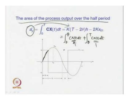
So, we can have expression for X t for different span of time. So, as you know I can find from wave form for this part of the wave form the corresponding output can be obtained using expression C X t, where X t can be given as you know, if the output is like this is the output half period of the output will consider, and relay switching takes place
