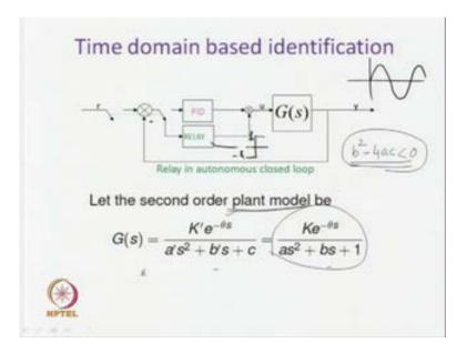
And when further assumption like b square minus four a c is less than 0 is made. Then only, this transfer function model or model plant model, transfer function is said to have underdamped characteristics, please keep in mind only when b square minus four a c is less than 0. Then only, the plant model becomes a plant model for an Underdamped system otherwise it is not.
