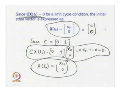
Now since c x t 0 has to be 0 for a limit cycle condition; that means, for to induce limit cycle for obtaining sustained oscillatory output this condition has to be made. So, when c X t 0 equal to 0, the initial state vector has to be given in some form as shown over here; then X t 0 has to be given as X 0 1 which is a non 0 value with zero element at the bottom, why that is so, since C is having the form 0 1; this vector having elements 0 and
