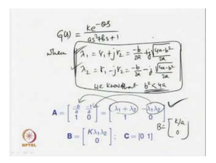
Let me, repeat how we have been able to find the state equations which has got constants A, B, and C, given G(s) in the form of k e to the power minus theta s a s square plus b s plus 1, when lambda 1 is equal to gamma 1 plus j gamma 2 is equal to minus b upon 2 a plus root of 4 a minus b square by 2 a, and lambda 2 is equal to gamma 1 minus j gamma 2 is equal to minus b upon 2 a minus j root of 4 a minus b square by 2 a. This is, you
