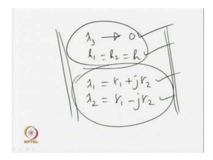
So, here what assumption you have to make lambda 3 tends to 0, and h 1 equal to h 2 equal to h, with those assumptions the peak time can be expressed as t p is equal to theta plus 1 upon gamma 2, where from gamma 2 came again. You need to substitute lambda 1 is equal to gamma 1 plus j gamma 2, and lambda 2 is equal to gamma 1 minus j gamma 2. So, with these substitutions the general expressions we have obtained.
