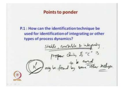
Now, how the identification technique can be used for identification of integrating or other type of process dynamics. They ask, I have already explained, now with proper choice C the parameter c associated with the underdamped second order plus dead time transfer function model with proper choice choices of C. It is possible to identify stable, unstable, and integrating process dynamics.
