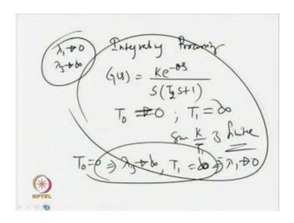
Similarly, the concept can be extended for integrating processes also integrating processes what are the integrating processes? We have got, I can say that this Transfer function model can be known as second order plus dead time Integrating process model.
