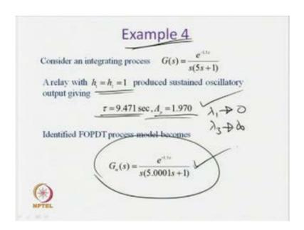
Now let us, consider this example: now, a symmetrical relay produced sustained oscillatory output giving half period as tau equal to 9.471 seconds, and A p as 1.970. Now with the substitution of again, I am the lambda 1 tends to 0, and lambda 3 tends to infinity, and using the analytical expressions. It is possible to find the Transfer function model for the integrating process as e to the power minus 1.5 s upon s times 5.0001 as
