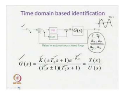
Earlier, we have seen also that the relay in autonomous closed loop yields are results in sustained oscillatory output. And let, the sustained oscillatory output be given by this wave form, and this is our y(t). Then, this is the arrangement that results in this type of
