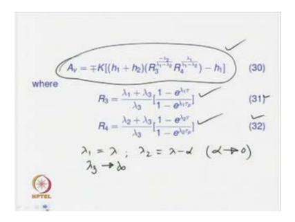
Now, how can we use those conditions to find simpler expressions for A v, when effort is made to identify second order plus dead time transfer function models with pole multiplicity. Now, I will go in that direction. Now, this R 3 and R 4 can be simplified further, when lambda 1 and lambda 2 are substituted by lambda 1 becomes lambda lambda 2 becomes lambda minus alpha with the condition alpha tends to 0. When this is used, then R 3 and R 4 can be obtained further in simpler form.
