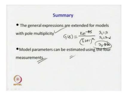
In which case, proper limiting values for different variables are to be used only. The beauty of this is that, the same set of powerful analytical expressions four analytical expansions and four measurements can be made use to identify a number of plant parameters or process model parameters where ,the processes can have pole multiplicity.
