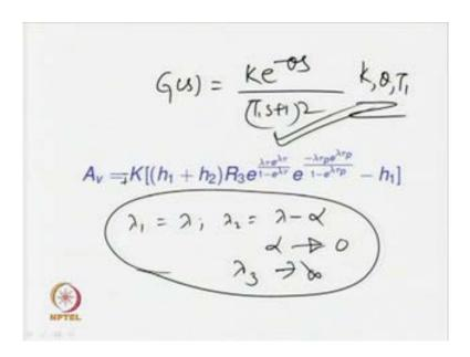
Let me summarize my lecture, the general expressions we have found earlier for identifying the transfer function model parameters of the general second order plus dead time transfer functions transfer functions can be extended for models with pole multiplicity. So, the model can have n number of poles also, it does not matter the same set of analytical expressions can be used with proper limiting values only. Where, I can have n number of poles located at the same point in the s plain.
