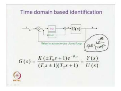
We shall say how we can identify a model transfer function of the form G(s) is equal to K e to the power minus theta s upon T 1 s plus 1 square. This type of model is known as models with pole multiplicity.
