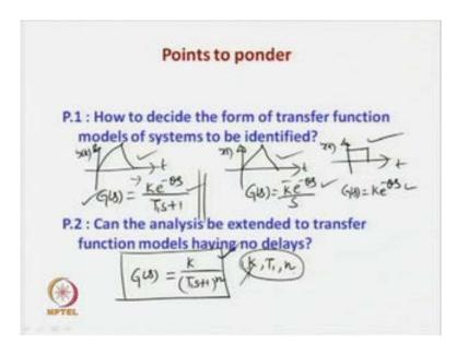
Now, some points to ponder. How to decide the form of transfer function models of systems to be identified? As I have already mentioned while I summarized the lecture, when the output of the relay test is of this form, go for the transfer function model G s is equal to k e to the power minus theta s upon T 1 s plus 1. And assume that one unknowns of this transfer function model is known a priori, then estimate the remaining two
