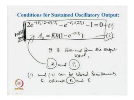
Then, the two analytical expressions. These two can be used to estimate k and T 1, instead of theta and t 1. Why I am mentioning? Suppose the theta time delay of the transfer function model theta is obtained from the output signal, then we are left with two more unknowns. Those are k and T 1. Then, k and T 1 can be estimated from the solution of the two non-linear equations.
