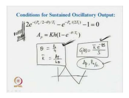
So, let me summarize these two things. Using these two expressions conditions for sustained oscillatory output, using two expressions both are obtained for a first order plus dead time stable system, it is possible to find the expression like theta is equal to P u by 4 and k bar is equal to A p by h theta, which can be used to estimate the unknown parameters k bar and theta, associated with our transfer function model G s is equal to k bar e to the power minus theta s upon S.
