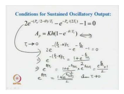
Now, we shall make use of the first expression now to estimate the time delay associated with the transfer function model. Now, when T 1 tends to 0, the expression 2 times e to the power minus P u by 2 minus theta upon T 1 minus e to the power minus P u by 2 T 1 minus 1 is equal to 0 can be written in the form of e to the power minus P u by 2 minus
