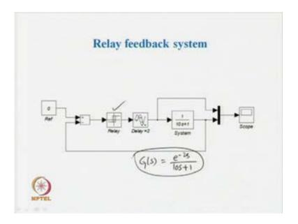
Now, let us consider the relay feedback system, where the relay induces sustained oscillatory output in the system. So, the system considered is G s is equal to e to the
