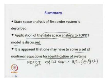
What we have learnt from this lecture? That state space analysis of first order system is described, where we have been able to derive simple expressions that can be solved simultaneously to estimate unknown parameters of a first order plus dead time model. Also, we have seen that application of the state space analysis can be extended to identify simplified models. How that can be done? That we shall discuss in the subsequent lecture.
