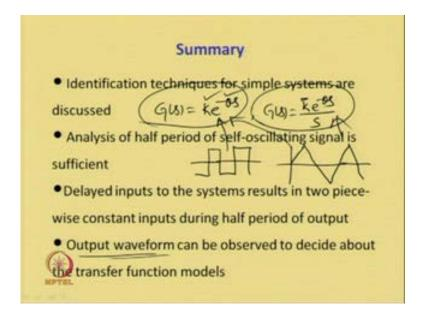
Now, what we have discussed in this lecture? Identification techniques for simple systems are discussed. For the system, dynamics are given by a gain with a delay or a velocity constant with delay and integrator. For these two simple systems, we have developed analytical expressions using state space; and, based on that, we have been able to establish relationship between the measurements of the output signal with that of the parameters of the transfer function model.
