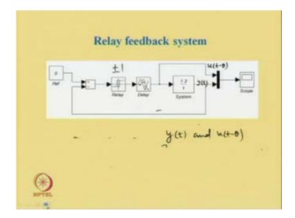
Then, when the relay test is conducted, what sort of output sustained oscillatory output we get from this system? That we shall see. Now, the scope has been connected to output of the system, which is denoted by y t and connected to delayed input. So, we get u t minus theta over here; that means the scope will be displaying the two signals: y t and u t minus theta.
