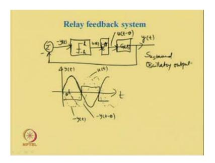
First, we shall discuss about the simple relay feedback system. We can draw a block diagram for that, where we have a summer, which is connected to a symmetrical relay of amplitudes h and minus h, which in turn is connected to a system; and, the system results in output y t. When this is simulated, the system generates sustained oscillatory output. The form of the output can be shown in this form, where we get periodic output of this form.
