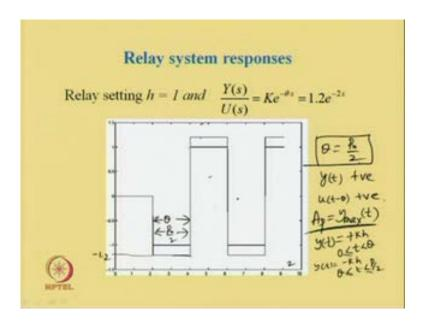
So, from the sustained oscillatory output signal, what we are getting? Interestingly, this theta is becoming p u by 2. So, theta is equal to p u by 2. This is a first one, why this is so? The main reason is that, whenever the output is going positive, y t is positive; during
