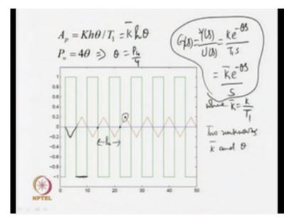
What unknowns we have now? G s; the transfer function model of the system is given by Y s upon U s is equal to K e to the power minus theta s upon T 1 s. This can further be written in the form of K bar e to the power minus theta s upon s; where, K bar is equal to
