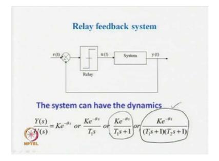
In today's lecture, basically, we shall see the output of a relay feedback system and the way one can obtain the output. Now, this simple relay-feedback system has got a relay, a symmetrical relay and system represented by the output and input ratio as Y s upon U s. So, the system input is u t and output is y t in time domain; whereas, in frequency domain, those are U s and Y s respectively.
