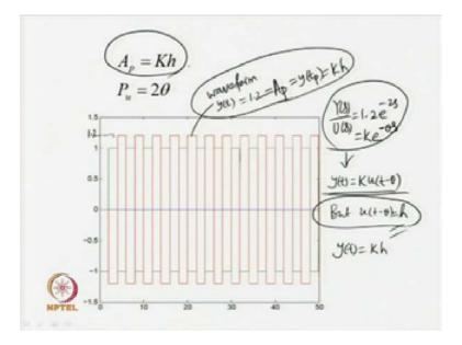
Using simulation, it has been found that the output will be of this form and the input will be of this form. So, the red one is the output signal, y t; and, the green one is the input signal u t minus 2. So, the input output signal will appear like this. Because of the time
