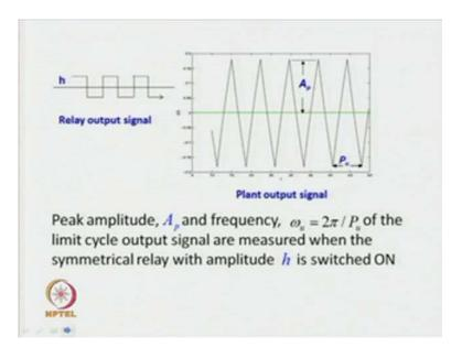
So, when we have the relay in the loop, the relay output signal will be like this, the relay output signal will be symmetrical, why that is so that we shall see in our subsequent analysis why do we get symmetrical relay output signal in spite of the presence of the controller in the loop.
