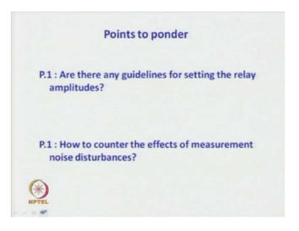
Some points to ponder. First point can be like this, are there any guidelines for setting the relay amplitudes? Generally relay amplitudes are decided based on the signal to noise ratio of the limit cycle output signal. When the limit cycle output is very much noisy, in that case, one has to judiciously choose the relay amplitudes. Minimum three cycles of stable limit cycle output must be obtained for making or before making measurements on the limit cycle output.
