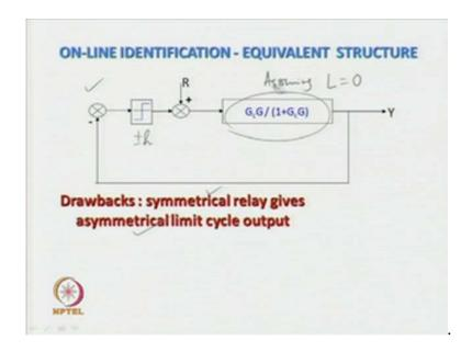
Now, what are the drawbacks of this scheme, why we are not happy with this one? If we look at carefully the equivalent structure of the online identification scheme, then the equivalent structure can be drawn in this fashion. Of course, assuming assuming the static load disturbance L to be zero, so when this L is equal to zero, at that time the online control structure can equivalently be represented by this structure. In this
