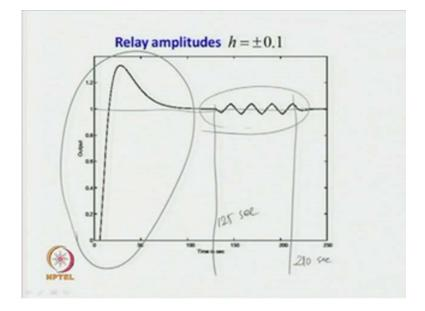
When the relay is switched on at about 125seconds, so when the relay is switched on at about 125 seconds, then limit cycle oscillation at the output takes place, so output becomes oscillatory. And when the relay is switched off at about 210 seconds, so when it is switched off at about two hundreds 210 seconds, then we go back to the steady state response.
