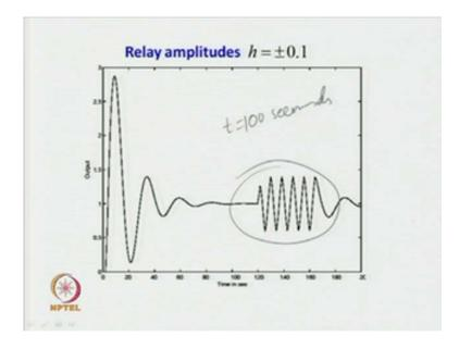
So, when the relay is switched on at time t equal to 100 seconds, then the limit cycle output takes place, the relay induces limit cycle output. And when the relay is switched off at about 160 seconds, so at time t equal to 160 seconds, at about 160 seconds, the relay is switched off. So, asked initially, switch on the relay at about time time t equal to 100 seconds and switch off the relay at time t equal to 160 seconds, in that case we get the output of this form.
