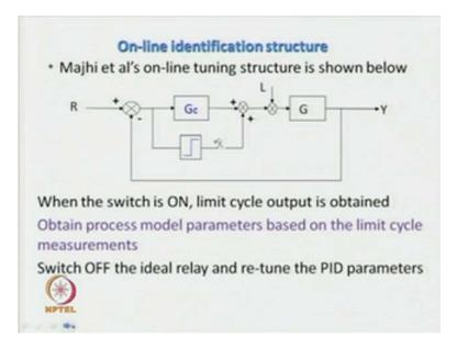
To overcome that we shall consider one more, online tuning structure proposed by majhi et al. Then, in that, in this structure, the relay is connected in parallel with the controller, so a relay is connected in parallel with the controller Gc and this is the simple control structure we have, where the relay is connected in parallel with the controller in the feed forward path and we have the closed loop system, relay control system.
