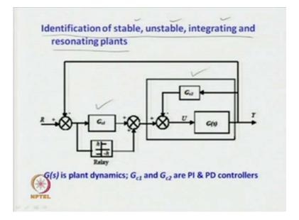
Next, we shall go to another scheme, the third scheme, online identification scheme, which is capable of controlling or tuning the parameters successfully for stable, unstable integrating and resonating plant. So, for a variety of, for a class of plant dynamics, this identification and control scheme can perform well, so what is there in this new online identification and control scheme? We got two controllers, we have got a controller G c1 here and we have got an inner feedback controller G c2.
