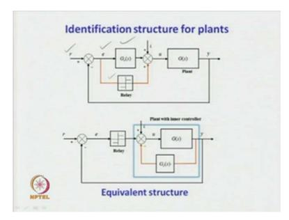
Identification structure; so, let us go back to the identification, why we are getting symmetrical limit cycle output from the new online identification scheme? To understand that let us consider the block diagram once more. R is the reference input, E is the any any error signal to the controller and also E is the error signal to the symmetric relay.
