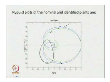
So, to ascertain the modeling accuracy to investigate the modeling accuracy, using the frequency response plots of both the actual and identified plant, we have obtained the Nyquist plot of the nominal and identified plants. So, the Nyquist plots of the original plant and the identified plants are plotted and shown over here; so there is no significant differences between the two plots then, one can conclude that the identified model truly represents the dynamics of the actual process.
