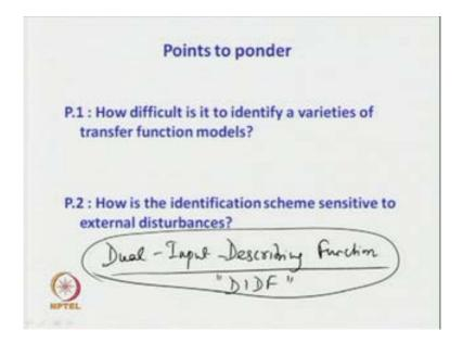
Some points to ponder, how difficult is it to identify a varieties of transfer function models, describing function based methods enables one to estimate two unknown parameters of a transfer function model. As we have seen the model can be of a general form or of any form, but only two unknowns of the transfer function model can be estimated using the describing function analysis.
