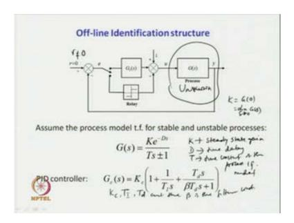
An off-line identification structure can be given like this, where r 0 equal to 0, when the relay is in action, whereas r 0 is not equal to 0, when the controller is in action. That means when the controller is in action, the process is in operation, then the relay test cannot be initiated, then when retuning of the controller is required, then we need to set
