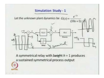
Now, this structure shows that when the relay is connected with the process unknown process, when some static load disturbance is presents present. In that case what will happen u the process input will be a symmetrical, as we know when L is equal to 0 what will be the form of the u; u will assume some symmetrical output waveform of the form some square or rectangular pulses.
