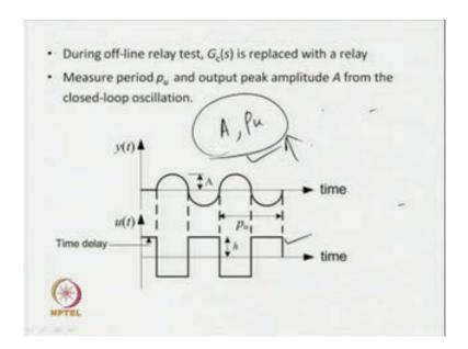
Now, for that during off-line relay test G c (s) is replaced with a relay, then we get limit cycle output, from the closed loop. So, the relay induces limit cycle output as shown here, where the output signal y (t), output signal has got some parameters; since we are getting sustained oscillatory output. Therefore, we can acquire or measure some information from the limit cycle output.
