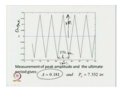
What we get we get a typical limit cycle output of this form, where this is x axis, this is the time axis, time in seconds and y axis is the output limit cycle output. Now we can make measurements the period of the limit cycle output, often measurement gives us P u to be of 7.332 seconds; similarly, the peak amplitude is found to be of magnitude 0.181. So, this is of value 0.181 and P u is of value 7.332 seconds.
