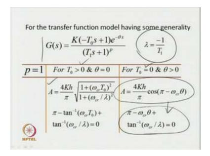
Now, for the transfer function model having some generality and given as G (s) is equal to K minus T 0 s plus 1 times e to the power minus theta s upon T 1 s plus 1 to the power P; also we can make use of the describing function analysis and estimate the unknown parameters of the transfer function model.
