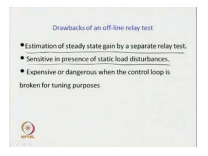
Now, drawbacks of an off-line relay test, what are the drawbacks an off-line relay test has, using the describing function the off-line relay test is found to give us only two analytical expressions; therefore, two unknowns of the transfer function model can be estimated.
