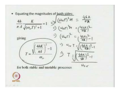
Equating the magnitude of both sides of the equation, we get 4 h upon pi A times K upon omega c r T square plus 1 root is equal to 1. So, for both the stable and unstable transfer function model, the magnitude of the analytical expression will be same. So, this can further be simplified as written in the form of omega c r T square plus 1 root is equal to 4 h K upon pi A implies omega c r T square plus 1 is equal to 4 h K upon pi A square.
