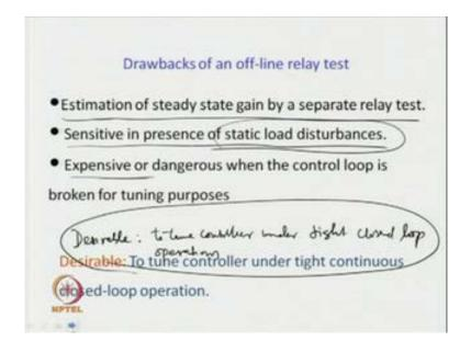
So desirable is to tune controller under tight closed loop operation and this is what we are not going to get from off-line tuning schemes.
