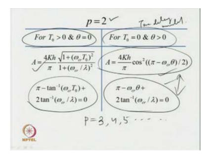
So, for higher values of P also we one can easily obtain similar expressions, when P is equal to 2, when the transfer function model is of second-order. In that case for the case of T 0 is greater than 0 and theta is equal to 0 the set of equations are obtained as A is this much and the phase condition gives us this equation. Now for T is equal to 0 and theta is not 0 for transfer function models, which are known as time delay models.
