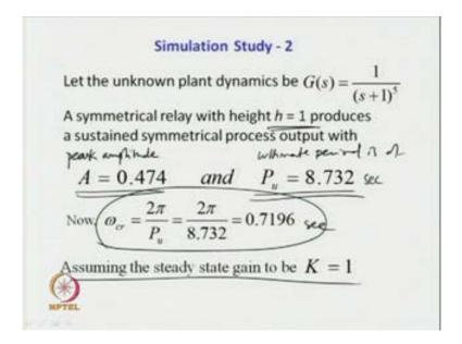
Let, us go to one more simulation study where the unknown plant dynamics is assume to be G (s) is equal to 1 upon s plus 1 to the power 5. So, in this case what we are going to do the actual plant is a plant all-pole plant with 5 repeated poles located at s equal to minus 1. So, the actual plant is something else. Whereas, we are going to estimate the plant dynamics by some first-order transfer function model.
