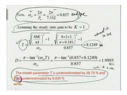
Then the critical frequency is calculated as omega c r is equal to 2 pi upon P u is equal to 2 pi upon 7.332 is equal to 0.857 second sorry radian per second. Now, the steady state
