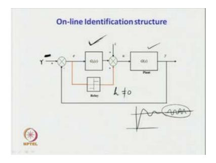
Next, we shall consider some on-line identification structure to overcome the limitations associated with off-line identification schemes; we shall consider an on-line identification structure. Where this r T is not necessarily has to be 0, so I can write it can be non 0 also this is your r T or reference input r simply. So, this gives us the structure of an on-line identification scheme.
