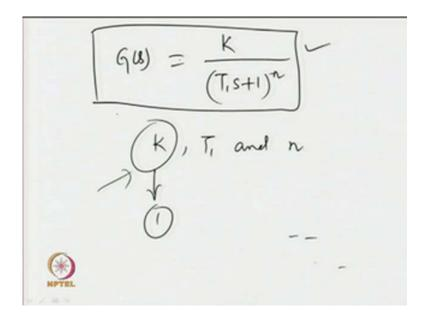
Now, one unknown has been estimated in this fashion, similarly this can be extended or we can go for some other technique to find the unknown parameters of model of transfer function model of a real time process. Let the real time process G s has the transfer function form K upon T 1 s plus 1 to the power n, before identification generally it is assumed that assumed that the transfer the process dynamics assume some specific transfer function form.
