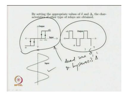
Now, a relay with dead zone can be shown like this, where delta is equal to the dead zone. Again we have got relay with dead zone and hysteresis, the input-output characteristics of a relay with dead zone and hysteresis can be shown like this. So, the relay has got dead zone and hysteresis. When the input to the relay is like this (Refer Slide Time: 47:50), the output will be of this form, when both dead zone and hysteresis in the relay are present.
