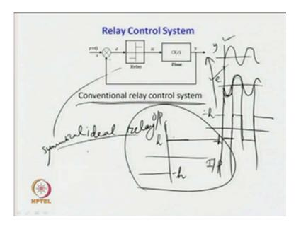
What a relay control system? The gain or proportional gain has been substituted by a relay, earlier we had some proportional controller here. Now, the gain of the proportional controller where changes gradually till some sustained oscillatory output is obtained from the closed loop system, but there some risk as we have discussed earlier; if the gain of the proportional controller is more than some then some specified value in that case, the output may blow out.
