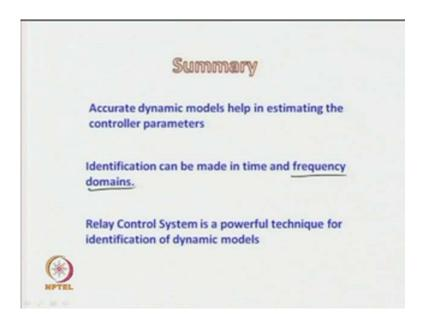
So in summary, accurate dynamic models help in estimating the controller parameters; therefore, effort should be made to estimate the parameters of transfer function models or time domain models as accurately as possible. Now, identification can be done in time and frequency domain; whereas, the frequency domain based identification techniques are found to be more convenient and useful.
