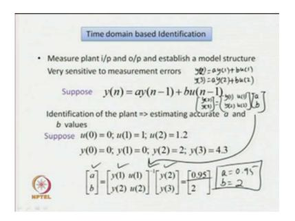
Now, we shall go to some identification technique, we shall study some time domain based identification of dynamics of a real time process. First one has to, let us consider we have some unknown process denoted by 1 upon denominator d n s, then we can apply some known input and we can measure the output from the process. So, from the measurement of input and output, a model structure can be established, but the model is found to be very sensitive to measurement errors.
