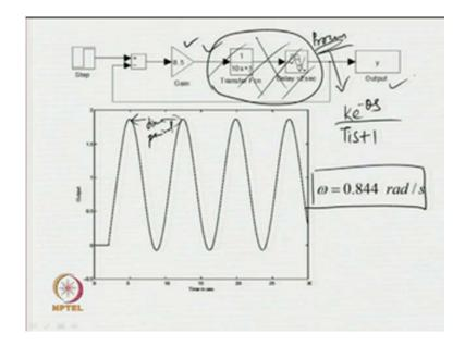
So, by read then trial, when we have the proportional gain of a value of 8.5, then we obtain a sustained oscillatory output for the closed loop system. When the proportional gain or proportional controller gain gain is equal to 8.5, then the closed loop system output becomes oscillatory a sustain oscillatory output. So, that is what we want, because these enable us to estimate two unknown parameters of a process model.
