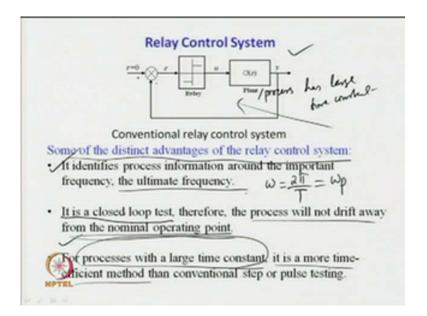
Let us see, what we have now some advantages of the relay control system are: it identifies process information around the input and frequency that is known as the ultimate frequency. The frequency at which we get the sustained oscillatory output signal is known as the ultimate frequency. The frequency of the sustained oscillatory output signal is known as the ultimate frequency.
