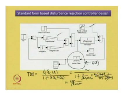
Now, the closed loop transfer function for the system for the closed loop system, for this system has to be given in the form of T s is equal to G G c s upon one plus G G c H s. Then here in the denominator, do not mind about the numerator; in the denominator, it can be written as G is your K upon s square plus alpha 1 s plus alpha 0, then G c is K p T is plus 1 upon T i s, then H s is this noise filter dynamics we give it by H s.
