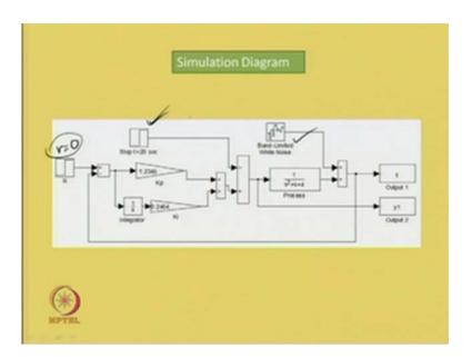
Now, when both the static load disturbance of magnitude minus 0.5 and band-limited white noise is present in the system, then the output of the system is obtained as shown over here.
