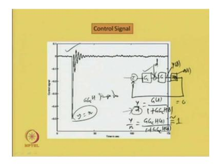
So, the noise filter has given us satisfactory load disturbance and noise measurement noise responses, the control signal is also quite satisfactory. So, with much less control effort, one is possible to obtain satisfactory closed loop performances from the closed loop system, of course with a noise filter in the loop.
