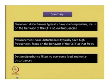
Now, in summary we can say, load disturbances are typically of low frequencies. Therefore, focus on the behavior of the closed loop system at low frequencies should be made to design suitable compensator for rejecting load disturbances whereas, measurement noise disturbances are typically of very high frequencies. Therefore, focus should be on to design controllers that would reject high frequency inputs or excursions in the closed loop system.
