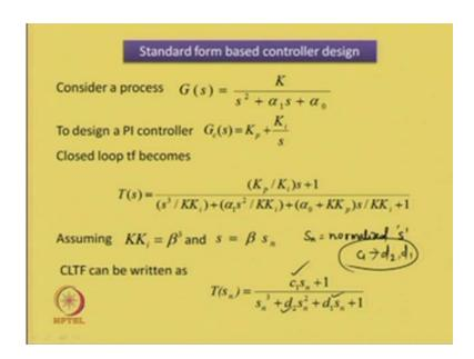
Consider a process, given as G s equal to K upon s square plus alpha 1 s plus alpha 0. So, this all-pole second-order process has got poles located at, suppose at far off from the left
