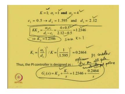
So, using K equal to 1, let us assume the process model is having the dynamics given by s square plus s plus 4. So, we consider an all-pole transfer function of the form G s is equal to 1 upon s square plus s plus 4 and the damping ratio for this one is equal to 1 upon 2 root of 2 root of 4 is equal to 1 upon 4 is 0.25. So, obviously, the damping ratio is 0.25 and we have got an under damped process for designing a PI controller for the system, for the second-order under damped system.
