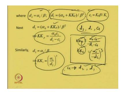
Now, we have got the d 2 expressed as alpha 1 upon beta, d 1 expressed as alpha 0 plus K Kp upon beta square and c 1 is equal to K Kp beta upon K Ki. These are the three variables we have in the standard transfer function, now manipulating this three variables, using the three variables, one can write d 1 is equal to alpha 0 plus K Kp upon beta square is equal to alpha 0 upon beta square plus K Kp upon beta square.
