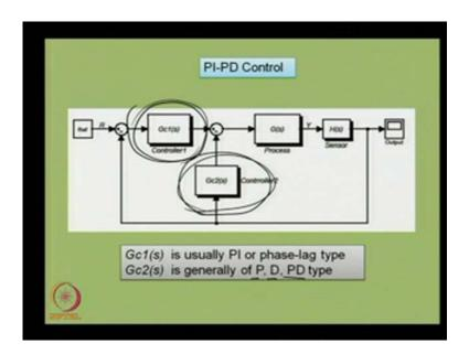
What is API-PD controller? The PI-PD controller can be depicted in this form, this block diagram represents a closed loop system where we have got a controller in the feed forward path and a controller in the feedback path.
