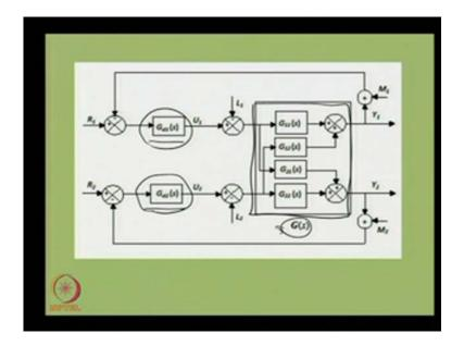
So, this block diagram represents the control system for a two input two output process. Now this G S represents G S represents the two input two output process or plant. So, if a plant is subjected to interactions from different internal loops that type of processor plant is known as two multi variable or two input two output plant. These two input two output plants can be extended to multivariable plants with the help of lots of interactions within the system.
