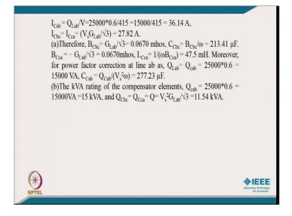
And that is 25000 into typically 0.6, that will be a reactive power divide by 415, [FL] it is a 15000 by 415 and equal to 36.14 Ampere. Similarly, I Cb will be again V s G Lab by root 3, [FL] again this current is 27.82. [FL] therefore, the B Cbc will be G Lab by 3, [FL] that is 0.067 mho and C bCbc by omega, it comes in 20, 201, 213.41 micro Farad and B Cca as G
