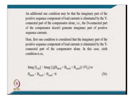
[FL], for this purpose, the sixth condition have to be added here, I mean like typically then only you can get the solution of this design. [FL] additional an additional an example I mean here we like to include couple of examples and but you may have a many such other conditions also.
