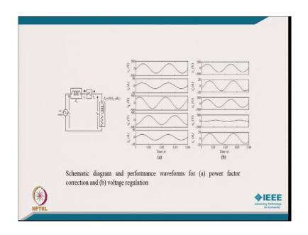
Well, in this case, we will be connecting compensator in series with the source impedance after which the load is connected and you can see the typically waveform for both the cases, for power factor correction and typically for voltage regulation both the cases I mean like. (Refer Slide Time: 34:57)
