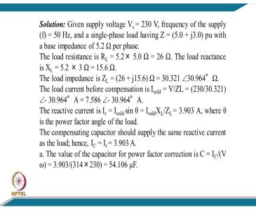
[FL] well, coming to the solution of this problem, I mean in the next slide, [FL] we can say the there is of course supply voltage given in the numerical problem 230 Volt and frequency is 50 Hertz and we have a single-phase load of again 5.0 and 3.0 per unit with the base impedance of 5.2 Ohm per phase.
