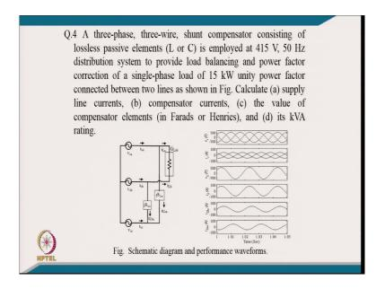
Coming to now the numerical problems on three-phase three-wire system, a three-phase three-wire shunt compensator consisting of lossless passive element is employed at 415 Volt, 50 Hertz distribution system to provide load balancing and power factor correction of a single-phase load of 15 kilo Watt unity power factor connected between two lines as shown in the figure. Calculate the supply line current, compensator current, the value of compensator element in Farad or Henry and its kVA rating.
