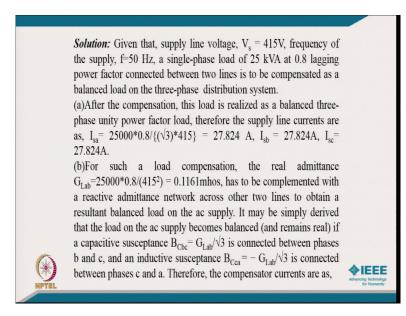
[FL] coming to the solution of is given that the supply line voltage is 415 Volt, frequency of supply 50 Hertz and single-phase load of 25 kVA at 0.8 lagging, power factor connected between the two line to be compensated as a balanced load on the three-phase distribution system.
