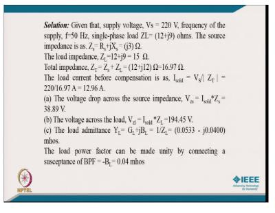
Now, coming to the numerical problems of this, I mean given the supply voltage of 220 Volt frequency of 50 Hertz and single-phase load of your 12 Ohm; 12 Ohm plus 9 Ohm and the source impedance here is your Z s equal to R s plus j X that is only R s is 0 and we took a only the inductive source impedance that is 3 Ohm for the case of simplicity to understand and the load impedance here is 12 plus I mean j 9 that comes the impedance as a 15 Ohm.
