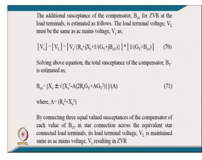
[FL] the additional susceptances of the compensator B cy for zero sequence zero voltage regulation at the load terminal is estimated as follow. The load terminal voltage must be the same as the ac terminal supply voltage, mains voltage. [FL] V s magnitude equal to V L and you can put the value of the typically here the V L.
