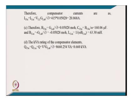
And putting the value of this, I mean we can get the value of I C compensator across the B c equal to I ca, I mean both are equal in magnitude V LL line voltage into G L divide by root 3 that is 415 into 0.0500, [FL] it comes like a current comes only 20.86 Ampere.
