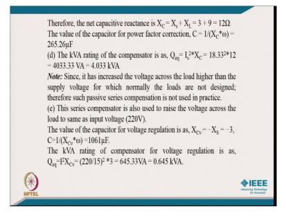
Therefore, the net capacitive reactance is X C equal to X L X s plus X L and that is typically, you can call it 3 plus 9 Ohm equal to 12 Ohm and the value of the capacitor for power factor
