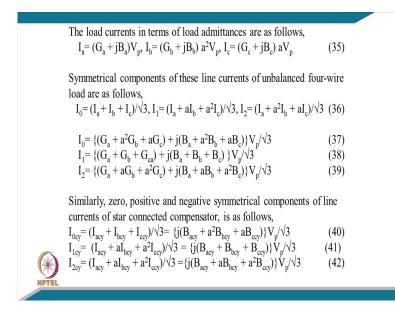
Well, now the load current in terms of load admittance can be expressed as follows. I mean a phase current I a can be written as a G a plus j a j B into V P that is a load, you can call it the admittance multiplied the phase voltage. Similarly, for b phase I mean G b plus j B b a square V P that is virtually for 240 degree phase shift of the voltage for b phase and c phase current can be represented again G c plus j B c and with the operator of 120 V a into V p.
