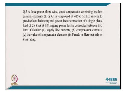
Coming to typically another three a three-phase three-wire shunt compensator consisting of lossless passive element is employed at 415 Volt, 50 Hertz system to provide load balancing and power factor correction of a single-phase load of 25 kVA at 0.8 lagging power factor connected between the two line. Calculate the supply line current, compensator current, the V A value of the compensator elements Farad and Henry and its kVA rating.
