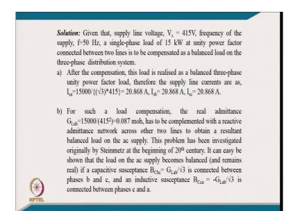
[FL] based on that, we have a now the solution to this problem given that the supply voltage V s equal to 415 Volt, frequency of supply 50 Hertz and single-phase load of 15 kilo Watt at unity power factor connected between two line to be compensated as a balanced load on the three-phase system.
