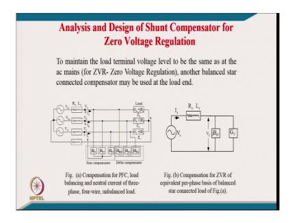
[FL] well, [FL] we have to extend this solution like analysis design of the shunt compensator for zero voltage regulation because in previous section, we consider it typically for unity power factor condition. [FL] for zero voltage regulation to maintain the load terminal voltage to be the same as the ac mains for zero voltage regulation, another balanced star connected compensator may be used at the load end.
