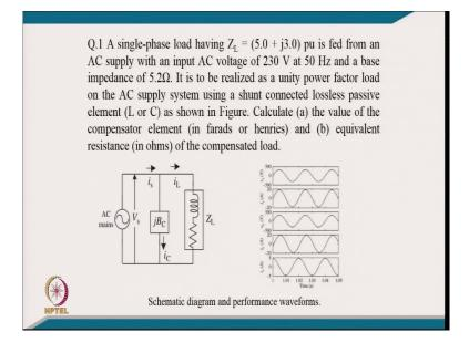
[FL], let us come to the typically the first numerical examples, I mean which is on the power factor correction of single-phase like I mean. [FL] the if you look into the problem, it is a single-phase having a load having a the load impedance of 5.0 plus j 3.0 per unit.
