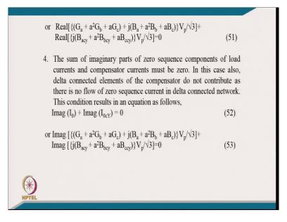
[FL] that is a another condition and you can keep the value of this and you can get the equation between load, you can call it the admittances and the star connected susceptances like. The fourth condition of course the sum of imaginary part of zero sequence current of load current and compensator current must be zero. In this case also, the delta connected elements of the compensator do not contribute and there is no flow of zero sequence current in delta connected network of the compensator.
