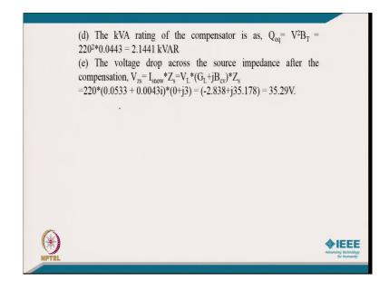
[FL] kVA rating, I have to find out for this compensator that will be V square B T and you can keep the value of V square 220 into your B 0.0443 and it comes 2.1441 kVAR. I mean that much capacitor if you connect it, then you will get a zero voltage regulation and the voltage drop across the source impedance after the compensation, we can find out I s new into Z s and that I s new will be is nothing but you can call it V L into your typically now G L plus j B v.
