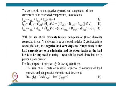
Well, similarly the zero sequence, positive sequence and negative sequence symmetrical component of the line current of delta connected compensator can be also written as follows. [FL] I 0 I 0cD means zero sequence current of the delta connected compensator can be written as I acD plus I bcD plus I cD divide by root 3 equal to 0 because there is no connection of delta connection to the neutral.
