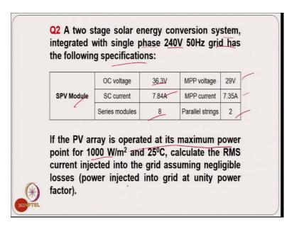
Coming to the  $2^{nd}$  numerical example. A two stage solar PV conversion system integrated with single phase supply of 240 V/50 Hz grid has the following specifications given in the table. If the PV array is operated at the maximum power point for 1000 W/m<sup>2</sup> and 25° C. Calculate the RMS current injected into a grid assuming negligible losses (power injected in the grid at unity power factor).
