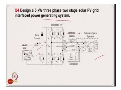
Now, coming to 4<sup>th</sup> example. Design a 5 kW 3 phase 2 stage solar PV grid interface system. So, we have a 2 state system solar PV generation, as shown in figure.
