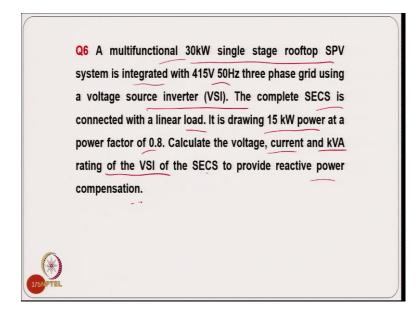
Coming to the 6<sup>th</sup> example. A multi functional 30 kW single stage rooftop solar PV photovoltaic system is integrated with the 415 V/50 Hz three phase grid using a voltage source inverter. The complete solar energy conversion system (SECS) is connected with a linear load. It is drawing 15 kW power at power factor of 0.8. Calculate the voltage current and KVA rating of the inverter of the solar energy conversation to provide reactive power compensation.
