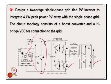
Starting with 1<sup>st</sup> example. Design a two stage single phase grid tied solar PV inverter to integrate 4 kW peak power of PV array with a single phase grid and circuit topology consist of a boost converter and H bridge voltage source converter.
