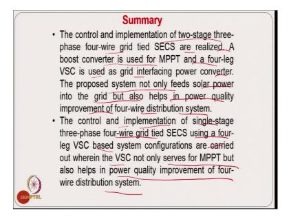
The control and implementation of two-stage three-phase four-wire grid tied system are realized. A boost converter is used for a maximum power tracking and four-leg VSC is used for grid interfacing power converter. This system not only feeds the solar power into the grid, but also helps in power quality improvement of four-wire distribution system.
