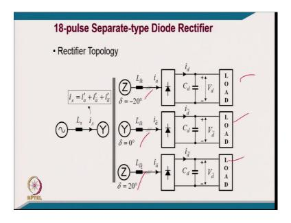
This is typically for 18-pulse. But, you have a separate load for every 6-pulse.
