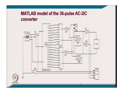
This is the model of the converter along with the transformer.
