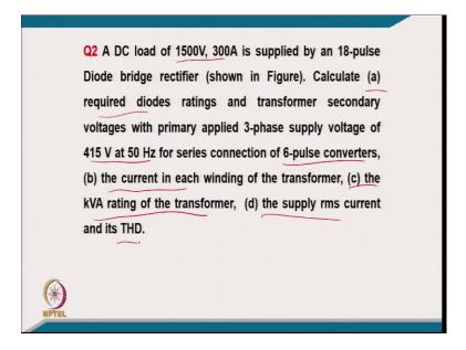
Coming to 2<sup>nd</sup> example, a DC load of 1500 V, 300 A is supplied by an 18-pulse diode bridge rectifier, as shown in figure. Calculate, the required diodes rating and transformer secondary voltages with primary applied 3-phase supply voltage of 415 V/50 Hz for series connection of 6-pulse converter, the current in each winding of the transformer, the kVA rating of the transformer, the supply RMS current and its THD.
