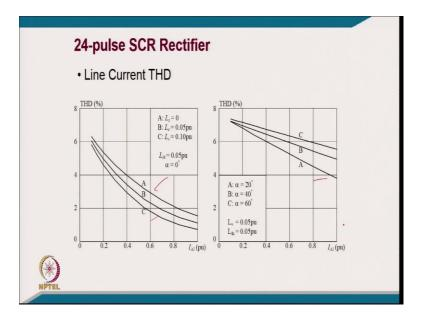
And here also you can see the effect of leakage reactance on THD.
