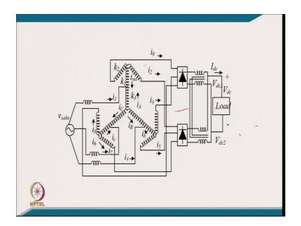
This is the typical connections, you can call it as an umbrella kind of connection, you are making like a tapping for giving input supply and then you are rising the voltage and then you are having a  $\pm 15$  degree phase shift for getting 12-pulse converter.
