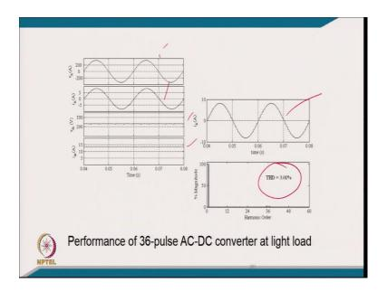
Current is in phase with the supply voltage and sinusoidal. And this is the harmonic spectrum and the THD around 3 percent of this 36-pulse converter.
