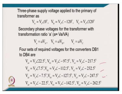
And that is the typically how we are going to have the design of that, I mean these are the voltage requirement.
