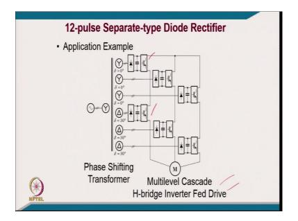
This is an interesting example; you can say multiple multi-level cascaded bridge inverters like Robicon drive system. Here, you can see, it is a kind of a like a 12-pulse connection, so, all these are 0 phase shift and these are 30-degree phase shift. So, for all 3-phases you need the separate secondary. And you can add the voltage there to get the
