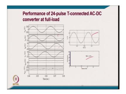
And these are of course, for 24-pulse with the pulse doubling, the THD reduces to order of 3.5 percent in place of 7.5 because again effect of the leakage reactance and the current goes very close to the sinusoidal.
