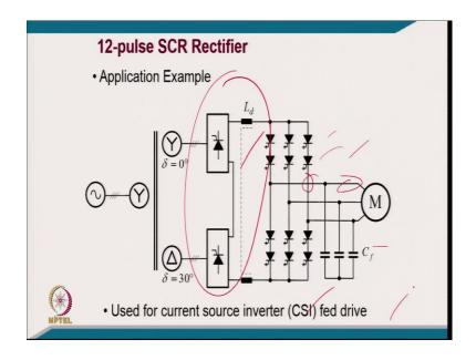
It has a low line current harmonic, and no SCR in series and that is why, it is used for variable frequency drive today. So, virtually, it is a driving a PWM current source inverter, where you are using GTO and you are using the capacitor for making this PWM current continuous.
