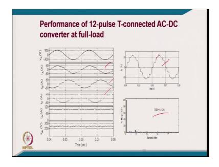
And these are the currents like typically in case of the your 12-pulse 3-phase currents drawn from the supply. And the THD of this, is in the order of 6.14% in place of 15 percent because of the effect of leakage reactance of the transformer.
