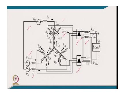
This is typically the connection for getting 12-pulse from 3-phase supply, with 2-phase shifted converter with the inter phase transformer, we are able to get phase shift like a  $\pm 15^{\circ}$ .
