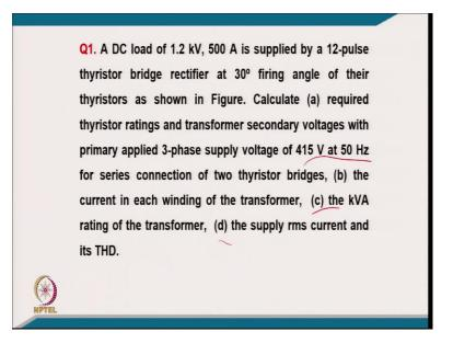
Starting with 1<sup>st</sup> example. A DC load of 1.2 kV, 500 A is supplied by a 12-pulse thyristors bridge rectifier at 30° fire angle of their thyristors, as shown in the figure. Calculate, required thyristors ratings and the transformer secondary voltages with a primary applied 3-phase supply voltage of 415 V/50 Hz for series connection of two thyristors bridge, the current in each winding of the transformer, the kVA rating of the transformer, the supply RMS current, and its THD.
