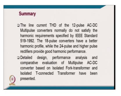
The line current THD of the 12-pulse converter, normally do not satisfy the harmonic requirement as specified by IEEE 519 standard, whereas, the 18-pulse converters have better harmonic. Further, the 24-pulse and higher number of pulses provide a good harmonic profile. Detailed design, performance analysis, and comparative evaluation of multi-pulse AC-DC converter based on isolated fork-transformer, and isolated T-connected transformer have been presented.
