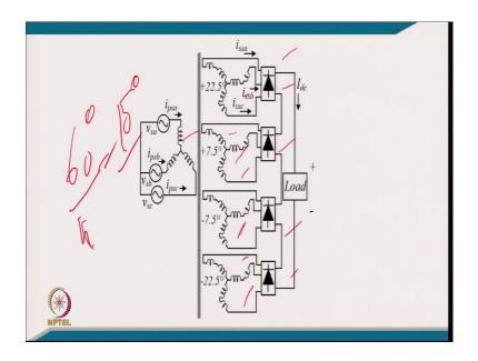
This is the 24-pulse converter, in this, the 4 bridges are connected in series. The phase shift should be like a 15 degree, i.e.,  $\pm 7.5^{\circ}$ , so, it is a 15° between two bridges. Because of 4 bridges, 60 by 4, it become your 15°.
