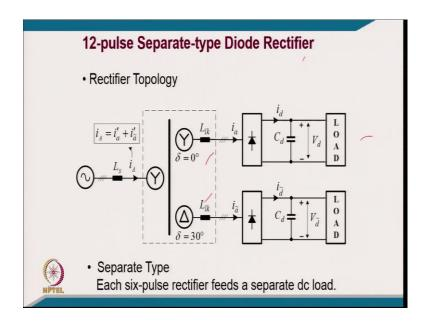
Further, you can have a 12-pulse separate diode bridge rectifier. Many applications we have a such thing. But if you have a phase shift here, then it gets reflected on this side.
