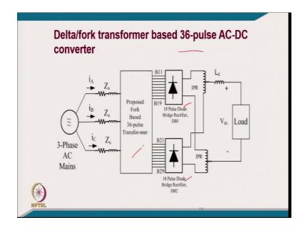
So, this is the power circuit diagram of delta/fork transformer based 36-pulse AC-DC converter.
