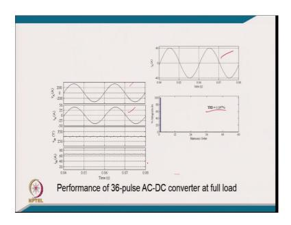
And this is the performance at full load. At full load, the THD is only 1.19 percent. You can see supply voltage supply current, and current waveform with the output voltage output current.
