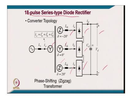
This is typically the you can call it an 18-pulse converter connected in series. You have 18-pulse converter where you require 3 converters, they are connected in series, and the
