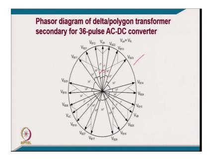
And this is the phasor diagram which all the points should be on same circle to make a same rms voltage on the secondary side.
