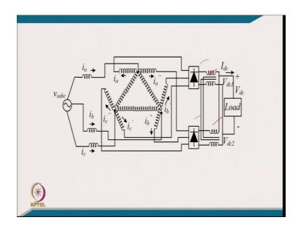
And this is the another connection for getting a 12-pulse of  $\pm 15^{\circ}$  which is called as extended delta.
