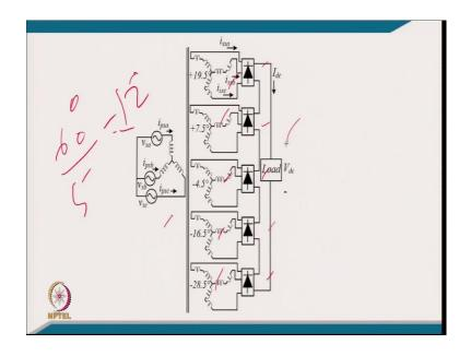
This is the system for 30 pulse. For 30-pulse, you have 5 converters each of 6-pulse.
