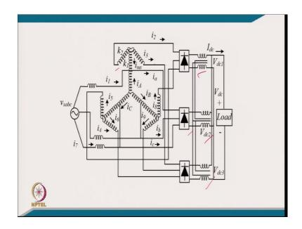
So, this is typically the connection for 18-pulse configuration with  $\pm 20^{\circ}$  phase shift with this fork kind or the umbrella kind of connections.
