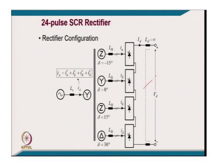
And this is for 24-pulse converter you are using 4 controlled bridges.
