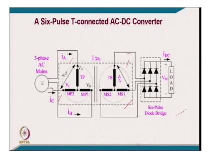
This is the circuit diagram for 6-pulse T-connected AC-DC converter.
