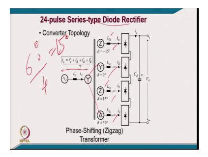
This is typically a 24-pulse series type of diode rectifier. So, here, you can have a 60degree phase shift divide by number of converter 4, it becomes 15-degrees phase shift. And this 15 degree you can find out here 0, +15, +30, and -15. There may be plenty of way, but that is the way how you can get with the zigzag and typically 30-degree phase shift.
