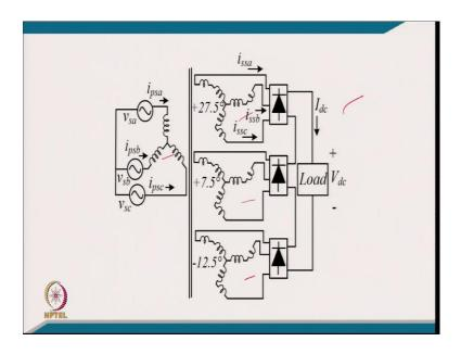
This is the typical connection. Because of zigzag connection, you are getting 18-pulses.
