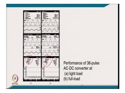
And these are the experimental results of the 36-pulse AC-DC converter under full load and light load conditions.
