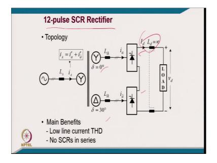
Now, this is the case of control by thyristors control converter or you can call it 12-pulse thyristors control rectifier, where you can control the firing angle for controlling the output power or the let us say if inductance, so, this current will be constant. Here, you will have again typically 30-degree phase shift for 12-pulses.
