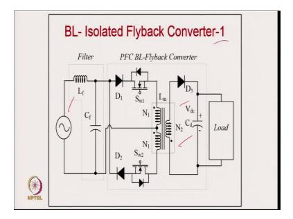
The bridgeless version of the flyback converter is shown here. In the bridgeless version the diode bridge is partially eliminated, of course, on the cost of couple of MOSFETs. The secondary circuit remains same, it may be multiple output also. The elimination of the diode bridge certainly enhances the efficiency up to some extent.
