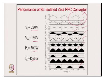
After, designing this converter for input voltage of 220 V, output voltage of 130 V, power of 500 W, and at 45 kHz, this is the simulated performance of isolated bridgeless zeta IPQC.
