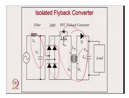
In conventional bridge-based flyback configuration, we will have an EMI filter, a diode bridge rectifier circuit, and of course, a power factor corrected flyback converter which can operate in discontinuous or continuous conduction mode. For discontinuous conduction mode we have to design flyback transformer's magnetizing inductance in discontinuous current mode. Otherwise, if you want typically CCM operation, then we need to design accordingly.
