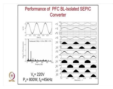
Well, after the design corresponding to 800 W, 220 V, 45 kHz; these are the typical waveforms, which includes supply voltage, supply current and DC link voltage. You can see, both pair of output inductor current remain in discontinuous mode operation. You can see, the THD even less than 2%, i.e., 1.95%.
