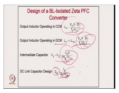
And, these are the design equations for the isolated bridgeless Zeta IPQCs under both CCM and DCM operation.
