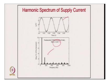
This is the supply current waveform and the THD. As per the harmonic's spectrum of supply current, the THD is 3.56 %.
