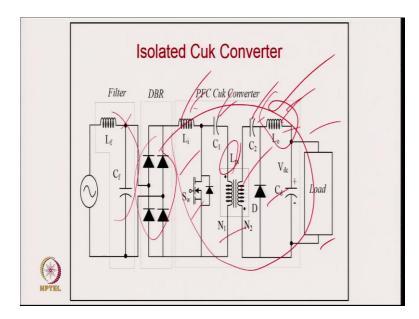
So, this is typically isolated PFC Cuk converter. This converter has an EMI filter, a diode bridge rectifier, and then an isolated Cuk converter. We can design this converter in many ways because there are 5 energy storage elements, i.e., input inductor, output inductor, energy transfer capacitors on primary side energy and secondary side, and the magnetizing inductance of isolation transformer.
