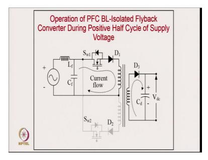
This is the operation of power factor corrected bridgeless isolated converter during positive half cycle.
