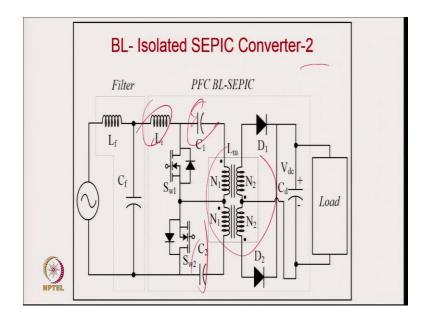
And this is the second bridgeless version of isolated SEPIC IPQC. In this, the diode bridge is completely eliminated.
