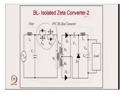
And this is another version of isolated bridgeless zeta IPQC. In this, the 2 switches conduct for positive and negative half cycle, alternatively.
