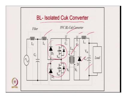
Well, this is the first version of the bridgeless isolated Cuk converter. In this, you have additional 1 diode, and 1 MOSFET, but you are able to get rid off with the diode bridge rectifier which reduces the losses in this converter.
