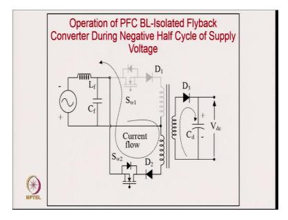
And this is the equivalent circuit for negative half cycle, the current flow path is shown by the dotted arrow. (Refer Slide Time: 08:41)
