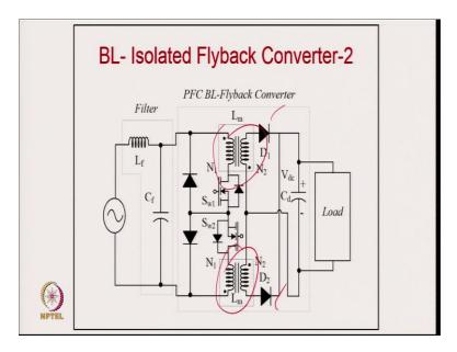
And this is the second circuit configuration which can be for little higher power. Because, this converter has two different circuits one for positive half cycle, another for negative half cycle with two separate transformers.
