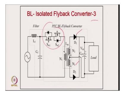
And this is the 3<sup>rd</sup> version of the bridgeless isolated flyback converter. Of course, we are using 2 devices in back-to-back manner, but we have completely eliminated the diode rectifier. In this, one MOSFET conduct for positive half cycle, and another conduct for negative half cycle. Then, in the secondary side, we have push-pull like configuration.
