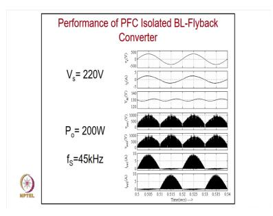
This is a typical example at 200 W and 45 kHz. You can clearly see, at supply voltage of 220, the supply current remains in phase with the supply voltage and the total harmonics distortion also remain negligible in this case. Further, the DC link voltage, switch voltage, and switch current are also given.
