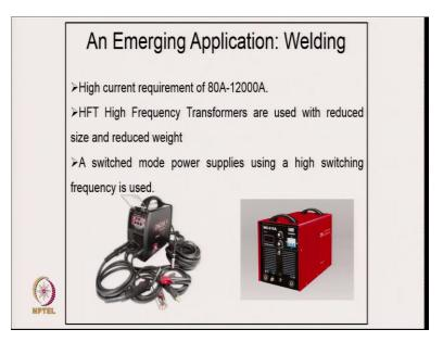
An emergent solution which is coming up is in welding machines. The high frequency welding machine require high current requirement (80 A - 12 kA) and utilizes high frequency transformer for the reduced size and reduced weight and reduced losses.
