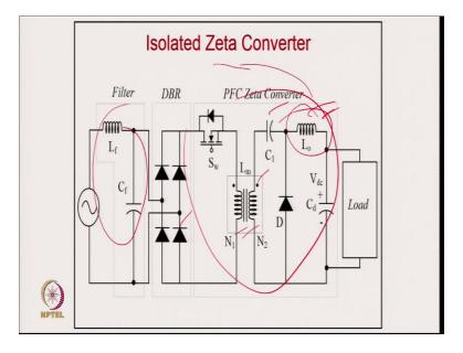
This is the typical isolated zeta IPQC, which have an EMI filter, the diode rectifier and isolated zeta converter. Here, the number of components is same as Cuk, SEPIC converter. Here, also you have a 3 element, output inductor, energy transfer capacitor, and magnetizing inductor, so, you have total 8 design choices.
