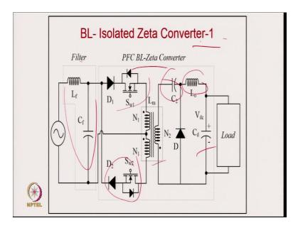
And this is the first bridgeless version of isolated zeta converter with power factor correction.
