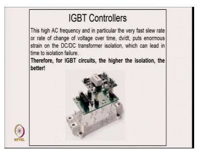
And another set is IGBT controllers. In such applications, very fast slew rate or rate of change of voltage over the time, i.e., dv/dt puts enormous strain on the DC-DC transformer isolation which can lead to isolation failure. Therefore, for IGBT circuits, the higher the isolation it is considered a better one.
