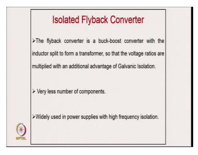
The flyback converter is a buck boost converter with the split inductor to form a transformer. So, the voltage ratio is maintained with the additional advantage of galvanic isolation and with very a smaller number of components. Such converters are widely used in power supply with the high frequency isolation over a wide range of power applications.
