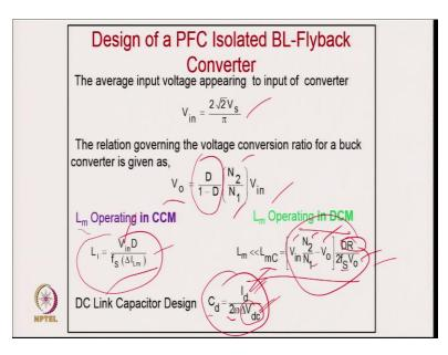
These are the design equations for the bridgeless isolated flyback converter topology under both continuous and discontinuous conduction mode.
