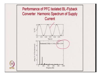
This is the harmonic spectrum of the supply current, as seen, the THD remains quite good, i.e., 3.3% for this power factor corrected isolated bridgeless flyback converter.
