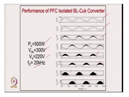
Now, coming to the case study, for 500 W with the output DC voltage of 300 V and the supply voltage of 220 V and at 20 kHz, these are the typical waveforms. Where, the output inductors are designed for discontinuous mode operation. The supply voltage and supply current remain in phase. The input inductor currents and capacitor voltages
