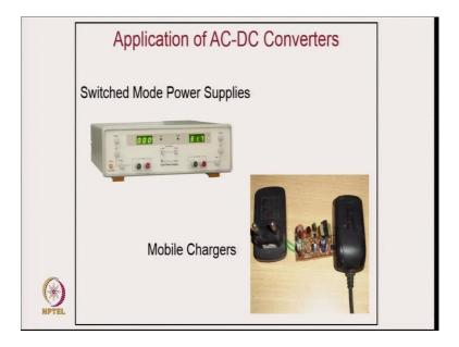
Now coming to the application of conventional AC-DC converters, in many applications, they cause the power quality problems, if not designed properly. The typical examples of such applications are switch mode power supplies, the mobile chargers, electric vehicle chargers, (which are coming up in a big way due to government policies and support), and LED driver circuits (for the lighting purpose may be in different power level starting from few watts it goes to like a maybe even 12 to 18 watts).
