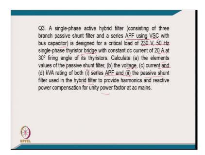
Coming to example 3, a single-phase active hybrid filter consisting of three branch passive shunt filter and a series active filter using a voltage source converter with the dc bus, designed for a critical load of 230 volt 50 hertz. Single-phase thyristor bridge with constant dc current of twenty ampere with 30 degree fire angle of its thyristor.
