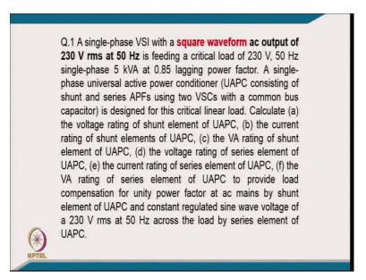
Coming to the first numerical example, a single phase voltage source inverter with a square wave ac output of 230 volt, 50 hertz is feeding the critical load of 230 volt, 50 hertz single-phase 5 kVA at 0.8 lagging, 0.85 lagging power factor and single-phase universal active power conditioner UAPC consisting of shunt and series active power filter using two VSC with common dc bus capacitor is design for this critical linear load.
