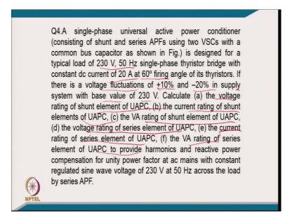
Coming to like a fourth numerical problem, a single-phase universal active power conditioner consisting of series and shunt active filters using two voltage source converter with common dc bus capacitor is designed for a typical load of 230 volt, 50 hertz single-phase thyristor bridge with the constant current of 20 ampere at 60 degree fire angle of its thyristor and if there is a voltage fluctuation of 10 percent plus and 20 percent minus in supply voltage with the base value of 230 volt.
