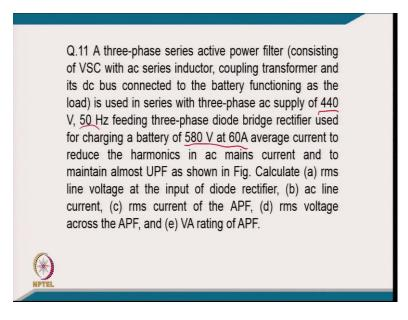
Coming to example number 11, a three-phase series active filter of voltage source converter with ac series inductor, coupling transformer and its dc bus connected to the battery functioning as a load is used in series with the three-phase ac supply of 440 volt, 50 hertz feeding a three-phase diode bridge rectifier used for charging a battery of 580 volt at 60 ampere average current to reduce the harmonics in ac mains current and to maintain almost unity power factor as shown in figure.
