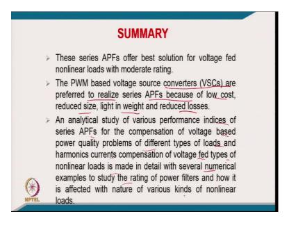
And this series active filter offered the best solution for voltage fed non-linear load with moderate rating. The PWM based voltage source inverters converters are used are preferred to realize the series active power filter because of low cost, reduce size, light in weight and reduce losses.
