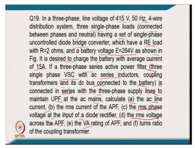
Coming to the 19 problem, in a three-phase line voltage of 415 volt, 50 hertz, 4-wire distribution system, three single-phase load connected between the phase and neutral having a set of single phase uncontrolled diode bridge converter which have a RE load equal to R equal to 2 ohm and battery voltage 264 as shown in the figure.
