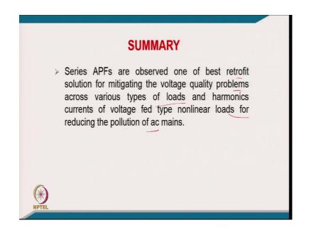
And series active filters are observed one of the best rate of it solution for mitigating voltage power quality problem across various type of load and harmonic currents of voltage fed kind of non-linear load for reducing the pollution of ac mains current.
