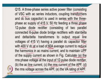
Coming to the numerical problem 15, a three-phase series active power filter consisting of voltage source converter with the ac series inductor, coupling transformer and dc bus capacitor is used to in series with the three-phase ac supply of 415 volt, 50 hertz feeding a three-phase 12 pulse diode rectifier consisting two parallel connected 6 pulse diode bridge rectifier with the star delta.
