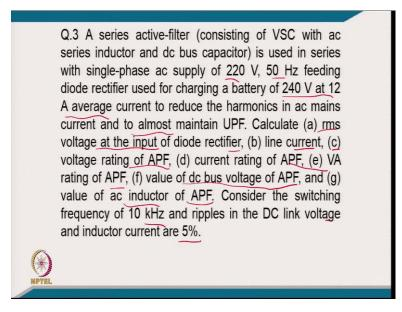
Coming to the numerical example 3. A series active filter constraints consisting of voltage source converter with ac series inductor and dc bus capacitor is used in series with the single-phase ac supply of 220 volt, 50 hertz feeding a diode rectifier used for charging a battery of 240 volt at 12 amp ampere average current to reduce the harmonics in ac mains current and to almost maintain unity power factor.
