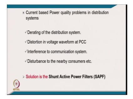
Then the current based power quality problems result in derating of the distribution system, distortion and voltage waveform at the point of common coupling, interference to communication system disturbance to nearby consumers.
