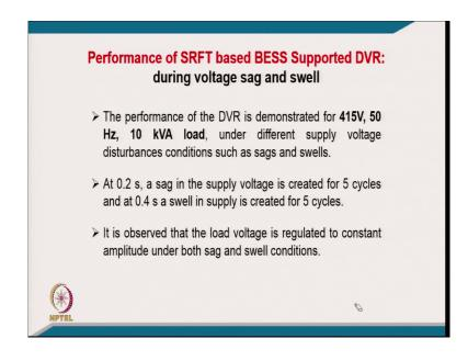
Ah The performance of synchronous loading reference frame BESS supported DVR we like to discuss first with that during voltage sag and swell. And the performance of the DVR is demonstrated here for 415 volt, 50 hertz, 10 kVA load under different supply voltage disturbances conditions such as voltage sag and voltage swell. At of course, we will discussed with the time domain a sag in the voltage is applied.
