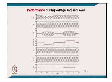
This is the typical result. I mean you can just see the first waveform. I mean like here it is the supply voltage or the voltage at the point of common coupling and there is a typically a voltage sag here 415 cycles. And then it was nominal voltage then sag 415 cycle then the nominal voltage then again swell for voltage 5 cycles in the PCC voltage.
