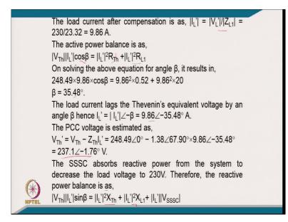
[FL] the typically calculating the current from this rated voltage divided by impedance it comes 9.86 and then putting a power balance I mean the power on the typically you can call it on grid side. I mean corresponding to voltage current and the angle between voltage and current and the loss in resistance of Thevenin and that is the load resistance.
