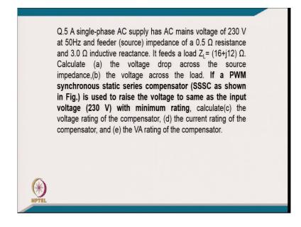
Coming to 5th example: A single phase AC supply has a AC mains voltage of 230 volt at 50 Hertz and feeder impedance of 0.45 ohm resistance and 3 ohm inductive reactance, it feeds a load of 16 point j 12 ohm. Calculate the voltage drop across the source impedance voltage across the load and if PWM a synchronous static series compensator is used to raise the voltage same as the typically the source voltage of 230 volt with the minimum rating.
