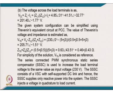
[FL] voltage across the load terminal is now Z L into I L and load is the parallel impedance of the both load multiplied I L. [FL] you can find out the load voltage now 201.4440 volt at the angle of minus 1.77. This voltage reduces I mean because both are the lagging power factor load and there is a kind of voltage sag is created here because of another heavy load connected at the point of common coupling.
