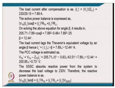
Coming to after compensation the typically the current, [FL] voltage is regulated to the source voltage of 230 volt divided by the impedance of load. [FL] it comes 7.889 ampere. And now we can have active power balance, the active power on the typically at the point of common coupling. It comes the power consumed in the Thevenin resistance plus the load power consuming the load.
