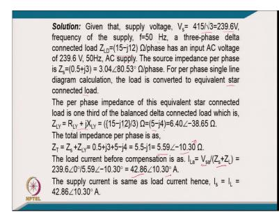
[FL] coming to the numerical part of this given that supply voltage equal to 415 by root 3 per phase that is 239.6 and we can say frequency supply 50 Hertz and 3 phase delta connected load of 15 minus j 12 ohm. Per phase have a AC voltage of 239 and the feeder source impedance is 0.5 plus j 3 ohm that comes 3.04 ohm at the angle of 80.53 degree.
