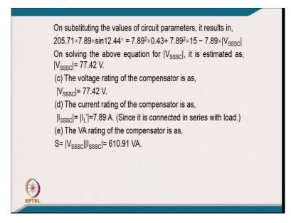
[FL] putting the value we get the typically the series compensator value of 77.42 volt and that is the same rating of the compensator. And current rating of compensator is says that load rate current rating that is 7.8 and multiplying these two with the VA rating of the compensator that is 610.91 VA like.
