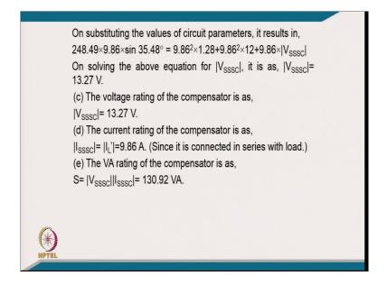
[FL] substituting the value we get here the series compensator value of 13.27 volt and the typically this is the same as the voltage rating of the compensator and current rating same as
