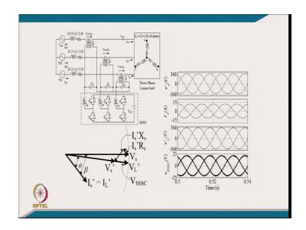
[FL] this is a typical circuit diagram. I mean we have a load here typically the balanced load. We have a source impedance. If compensator is not used this voltage will certainly go down because a lagging power factor load. And there is a source impedance which have a highly inductive part like.
