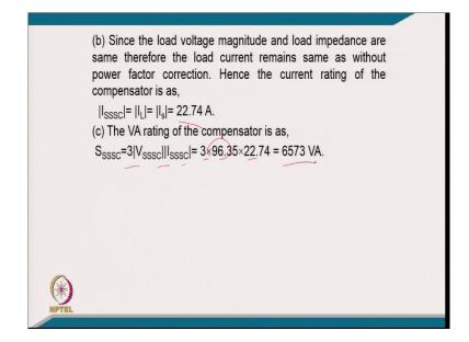
[FL], since the load voltage magnitude and source and load impedance are same, therefore, the load current remains the same without power factor correction hence the current rating of the compensator will be same 22.74 ampere. And VA rating will be 3 time V SC and I SC. [FL] this is 3 into the voltage 96.35 and current of its rating of 22.74 that comes 6573 volt ampere.
