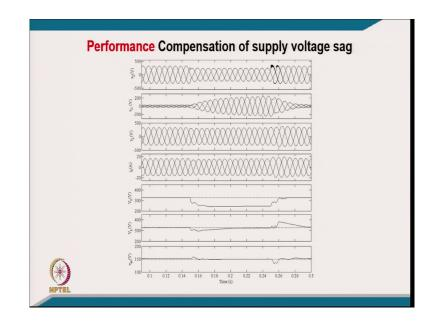
And in the typical case you can see here it is the sag is applied for 5 cycles and you have injected voltage here. So, that the load voltage is maintained sinusoidal balance and constant across the load. [FL] load is not getting affected by the sag and because of that your load current is also typically balanced and sinusoidal and you can see the how the source voltage is reduced. PCC voltage reviewed but load voltage is regulated and DC link voltage is regulated.
