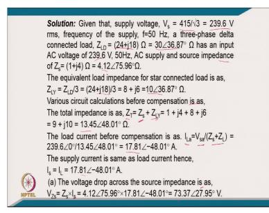
[FL] coming to the solution that given that supply voltage of phase voltage is 415 by root 3 that is 239.6 volt and frequency of 50 Hertz and we have a load impedance Z LD equal to 24 point j 18 that is 30 ohm at the angle of 36.87 has a input voltage of 239.6 volt at 50 Hertz and AC supply and source impedance is Z s equal to 1 plus j 4 ohm. It comes 4.1 2 ohm at the angle of 75.96 degree and the equivalent impedance of into the equivalent star is typically Z by Z L y equal to z ld by 3.
