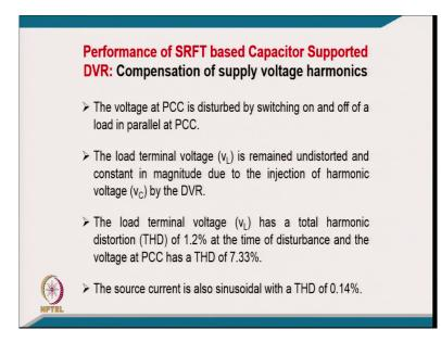
[FL] coming to like a performance of this SRFT based capacitor supported DVR with a compensation of supply voltage harmonic. [FL] voltage at PCC is disturbed by switching on and off the load in parallel to PCC. And the load terminal voltage will remain undistorted and constant in magnitude due to injection of harmonic voltage by DVR.
