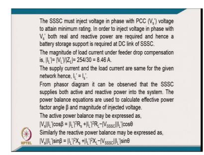
[FL] now series triple SC must inject the voltage in phase with the PCC voltage to attain minimum rating and in order to inject the voltage in phase with V s dash both real and reactive power are required and hence the battery energy storage support is required at the DC link of triple SC.
