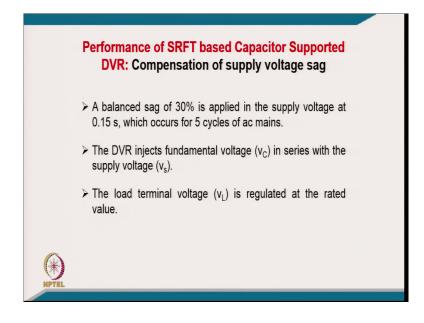
[FL] typically coming performance of the synchronous reference frame theory based capacitors supported DVR and here let us say for considering the consistent compensation of supply voltage sag, a balance sag of 30 percent is applied in the supply voltage at a time of point 0.15 second and which occurs for 5 cycles in of AC mains. And DVR inject the fundamental voltage in series with the supply voltage and load terminal voltage is regulated at the rated value.
