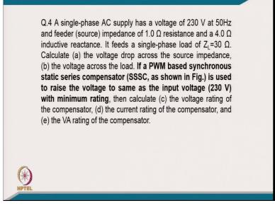
Coming to 4th example a single phase AC supply has a voltage of 230 volt at a 50 Hertz and feeder source impedance of one of 1 ohm resistance and 4 ohm the inductive reactance and you feed the single phase load of 30 ohm. And calculate the voltage rating across the source impedance, voltage rating across the load, a PWM based synchronous static series compensator is used shown this used to raise the voltage to the same as the input voltage with the minimum rating.
