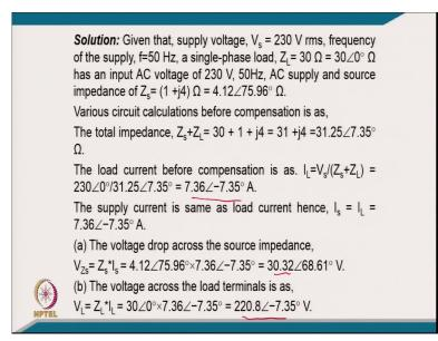
[FL] coming to numerical part of this given that the supply voltage V s equal to 230 RMS and frequency of 50 Hertz and single phase load up to 30 ohm and it has a AC voltage of 230 volt 50 Hertz and supply impedance of typically 1.1 plus j 4 ohm and that comes at 4.12 at the angle of 75.96 degree ohms and various circuit calculation before the compensation.
