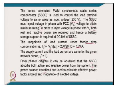
The series connected PWM synchronous static compensator is used to control the load terminal voltage to the same as the input voltage of 230 volt. [FL], SS triple SC must inject the voltage in phase with the PCC voltage to attain the minimum rating in order to inject the voltage in phase with the V s both real and reactive power required.
