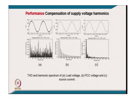
And this is the harmonic spectrum typically of your load voltage which have a THD of only 1.2 percent where the PCC voltage have a THD of 7 type 0.22 percent and the typically the load current or have only the THD of 0.14 percent like I mean. These are typical [FL] you can call it harmonic performance of this typically of DVR compensation system.
