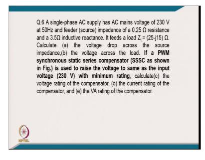
Now, coming to the sixth numerical a single phase AC supply has a AC mains voltage of 230 at 50 Hertz and feeder source impedance of 0.25 ohms resistance and 3.5 ohm inductive reactance. It feeds a load of Z L equal to 25 ohm minus j 15 ohm. And calculate the voltage drop across the source impedance, voltage drop across the load.
