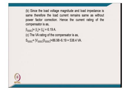
[FL], since the load voltage magnitude and load impedance are the therefore, the load current remains the same as without the power factor correction. Hence, the current rating of the compensator is your current or same, but voltage rating of compensator is we calculated. [FL] multiply this will be 538.4 VA rating like I mean.
