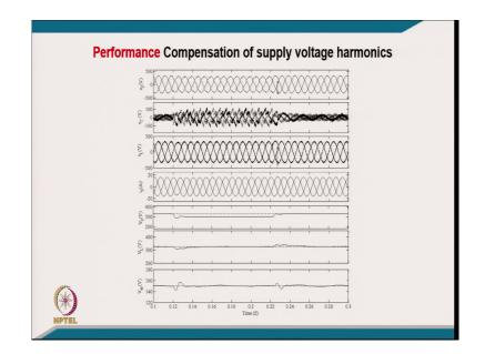
[FL] you can clearly see here you have a typically little sag with the harmonics in the voltage. These are the injected voltage and you will say in load voltage are balanced sinusoidal that is the reason the load current is also balanced and sinusoidal. And you can clearly see during this typically of injected harmonic the fundamental slightly reduced here, but the load voltage is not affected and the DC link is also not affected.
