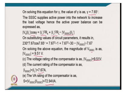
[FL] this angle at which at it to be injected 7.65 degree and thus triple SC supply the active power into the network to increase the load voltage hence the active power balance can be expressed. [FL] from this relation of active power on the typically grid side we put the loss in source impedance than loss in load.
