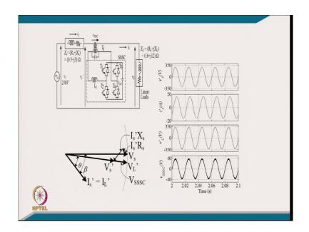
[FL] this is the typical case. I mean we have a load impedance. We have a source impedance if compensator is not put certainly load voltage will reduce because of lagging power factor and drop of source impedance. [FL] it is a worst voltage regulation, but we are injecting the voltage with the minimum radiating in the sense minimum voltage injection. [FL] that is corresponding to the phasor of this typically how it comes and we inject the voltage just to take care of the drop of this.
