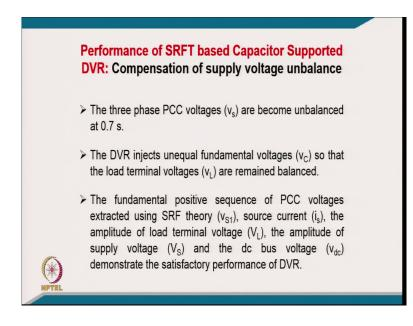
[FL] coming to the performance of this synchronous reference frame theory based capacitor supported DVR for the compensation of supply voltage unbalance and the three phase PCC voltages are have become unbalanced at typically 0.7 second. And DVR inject unequal fundamental voltage so that the load terminal voltage are remain balanced.
