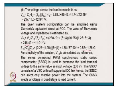
[FL] the voltage across the load terminal will be your Z L I L. [FL], keeping the value of this it comes typically 237.11 volt and the given system configuration can be simplified using Thevenin equivalent circuit at PCC. The value of Thevenin equivalent the voltage and impedance can be calculated
