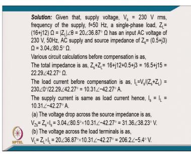
Coming to the typically numerical part of this, given that supply voltage V s equal to 230 volt RMS you can say of supply 50 Hertz and a single phase load of Z L equal to 16 point j 12 ohm Z L at the angle of 0 that comes 20 ohm at the angle of 36.87 ohm has an input AC voltage of 230 volt 50 Hertz, AC supply and source impedance of 0.5 ohm plus j 3 that comes 3.04 at the angle 80.5 degree ohm.
