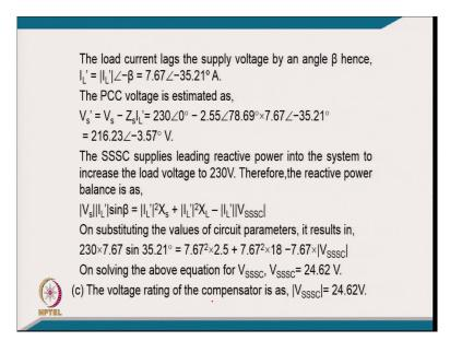
[FL] load current lags the supply voltage by an angle beta and that is the L delta c equal to 7.67 that minus 35.21 and PCC voltage is estimated that is V s dash equal to V s into Z s into I l. [FL] putting the value we get this is typically now the point of common coupling voltage 216.23 minus 3.57 degree volt and SSC applied during reactive power into the system to increase the load voltage to 230. Therefore, the reactive power balance is achieved.
