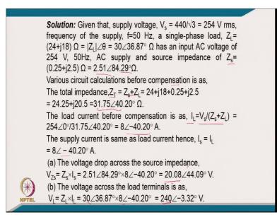
[FL] coming to numerical part of it given that the supply voltage V s equal to 440 by root 3 250 volt RMS, frequency of supply 50 Hertz and a single phase load Z L equal to 24 point plus j 18 that is typically 30 ohm at the angle of 36.87 with the input voltage of 254 that is 415 by root 3 50 Hertz so, AC supply and source impedance is typically 2.51 ohm at the angle of 84.29 degree.
