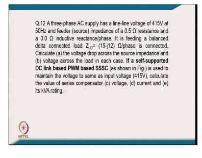
Coming to the 12th numerical problem: A three phase AC supply has a line voltage of 415 volt at 50 Hertz and feeder impedance of 0.5 ohm and resistance and 3 ohm reactant inductive reactance and it is feeding the balance delta connected load of 15 minus j 12 ohm per phase
