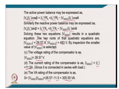
[FL] the active power balance may be expressed as typically the active power on the supply side then comes equal to the source loss in source impedance, loss in load and then the typically the active power injected minus the active power injected by the series compensator.
