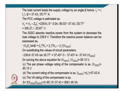
And the current will be there now at this angle of 37.43 ampere at the angle of typically of 30.77 and PCC voltage we can calculate. From here it comes like typically 300.27. [FL] this is much higher voltage and SSC absorb the reactive power to decrease the voltage to 239.6 from 300 and there therefore, reactive power can be expressed from reactive power balance.
