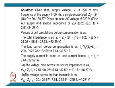
These are numerical part of the problems that given that supply voltage of 220 volt RMS frequency 50 Hertz and single phase load of 24 ohm minus j 18 and that comes 30 ohm at the angle of 36.87 ohm has a input voltage of 220 volt and a source impedance of 0.25 plus j 2.5 ohm which comes 2.51 at the angle of 84.28 ohm.
