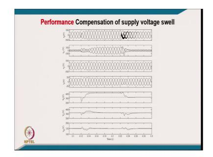
[FL] you can clearly see here in the PCC voltage there is a swell for 5 cycles and this is the typical injected voltage. And after injected this voltage I mean the load voltage is regulated sinusoidal balance across the load and thus the region the load is not affected I mean by this particular sag also.
