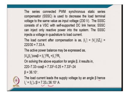
[FL] series compensator connected PWM synchronous static compensator is used to decrease the load terminal voltage to the same as.
