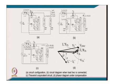
[FL], these are the typically you can call it the circuit diagram of typically of the configuration where I mean that is the original load this is series compensator and in for short period another load is connected that is Thevenin equivalent of this. And this is the typically the final along with the Thevenin equivalent the circuit diagram for from which calculation are to be made.
