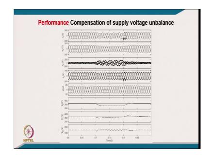
[FL] you can see here it is we have a unbalanced voltage I mean in the PCC, but the load voltage is regulated and this is the injected voltage. [FL] unbalanced voltage only to be injected there and typically the I mean like that is positive then this is load voltage and then the load current is not affected.
