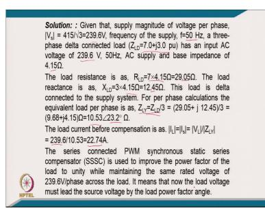
[FL], given supply voltage per phase is a 415 by root 3 239.6 and frequency of supply 50 Hertz and three phase delta connected load of Z LD equal to 7.0 plus 3 per unit has an input voltage of 239.6 and the base impedance of 4.15 ohm. [FL] the load resistance multiplying the per unit and this it comes 29.05 ohm and the load reactance comes same 12.45 ohm.
