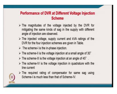
[FL] coming to now the performance of DVR at different voltage injection scheme, I mean [FL] we can call it the magnitude of voltage injected by the DVR for mitigating the same kinds of sag voltage sag in the supply with different angles of injection. The observed which we discussed last time in the different cases and the injected voltage supply current and kVA rating of the DVR for the 4 injection are given in the table like I mean.
