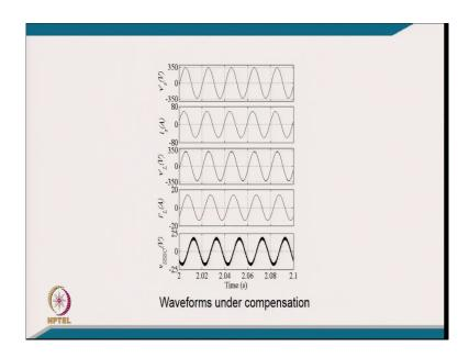
[FL] this is the phase diagram of the total like. And these are of course, the voltage you can call it the PCC voltage and the grid and load current and source current the load voltage and load current unlike and typically the your compensator voltage.
