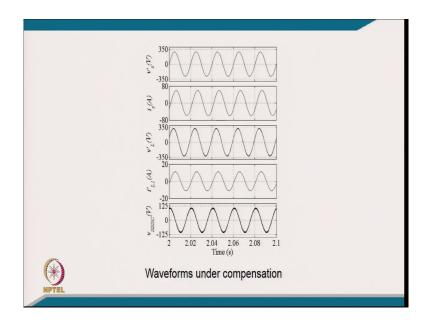
And after doing the all this I mean this is the typical waveform of the PCC voltage then the load current source current, load voltage modified load voltage, load current and series injected voltage which are in 90 degree from the current load current.
