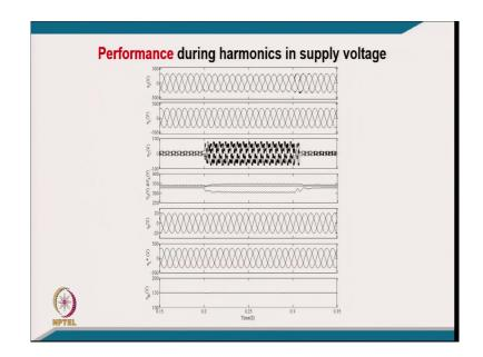
[FL] you can see here I mean here it is the nominal voltage and here it the voltage harmonics are injected at the point of common coupling and then nominally and, but you can see the load voltage is I mean sinusoidal and it is not I mean polluted from the harmonics.
