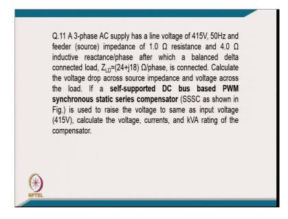
Coming to the numerical number 11: A three phase AC supply has a line voltage of 415 volt, 50 Hertz and a feeder impedance of 1 ohm resistance and 4 ohm resistance inductive reactance per phase after which a balanced delta connected load of Z LD equal to 24 point j 18 ohm per phase is connected.
