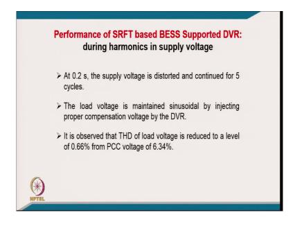
[FL] now, coming to performance sorry performance of synchronous reference frame theory with, but BESS supported during the harmonics in supply voltage. [FL] for the 3 cycle there is a supply voltage distorted, for 5 cycle and the load voltage maintained sinusoidal by sorry proper compensation of voltage by DVR and is observed that the total harmonic distortion in load voltage sorry is reduced to a level of 66 percent from PCC voltage of 6.34 percent.
