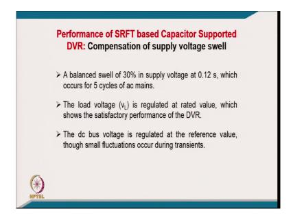
Coming to that typically the on another condition of performance of synchronous reference frame theory based capacitor supported DVR for the compensation of voltage swell. [FL] a balanced again swell of 30 percent in supply voltage is applied which occurs for 5 cycles of AC mains frequency.
