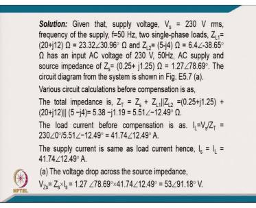
[FL] coming to numerical part of this given that the supply voltage V s 230 volt RMS, so, and frequency of supply 50 Hertz. And two single phase loads Z L1 equal to 20 plus j 12 that is 23.32 at the angle of 30.96 degree ohm and Z L2 5 minus 4 j 4 ohm which comes to like a 6.4 at the angle of minus 38.65 degree ohm. And has a input AC voltage of 230 volt AC supply impedance of 0.25 plus j 1 point ohm and the circuit diagram shown in figure.
