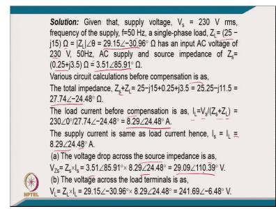
Coming to the solution part of this given that the supply voltage V s equal to 230 volt RMS, frequency of supply 50 Hertz and single phase load of Z L equal to 25 minus j 15 ohm and putting the value it comes 29.15 ohm at the angle of minus 30.96 degree. And has AC input voltage of 230 volt, 50 Hertz, AC supply and source impedance equal to that is equal to 0.25 plus j 3.5 ohm that comes 3.51 ohm at the angle of 85.91 degree and various circuit calculation before the compensation.
