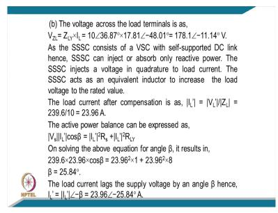
The voltage across the load terminal is now the load impedance multiplied the load current. [FL] we are putting the value it comes one 178.1 volt at the angle of minus 11.14. This is certainly much much lesser than typically through 229, the rated voltage because of lagging power factor and the source impedance is also of inductive nature.
