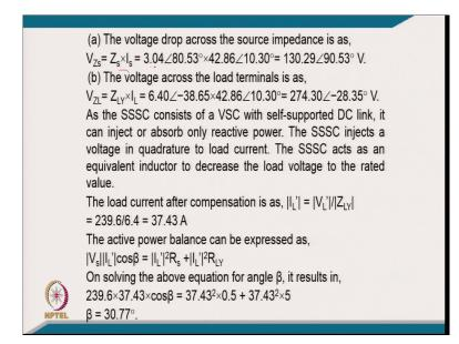
[FL] now the voltage drop across the source impedance will be impedance multiplied the current and it comes 30 130.29 volt at the angle of 90.53 degree and voltage drop across the load will be now load impedance multiplied the load current. It comes like a 274.30 volt and this voltage is much higher than the rated voltage because the load is inductive. [FL] we have negative voltage regulation.
