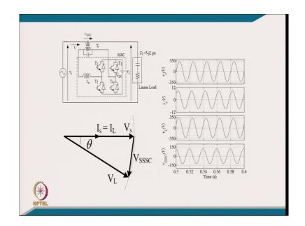
[FL] if you look into typically, I mean we have here the load and series compensator. I mean typically here and you can clearly see the I mean the we can say the source voltage is this much and load voltage also we want same. [FL] typically we have to inject the voltage typically of this nature so that it is on the same arc like. [FL] we modify the control in that manner.
