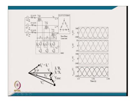
The typical circuit we have a here source impedance, we have a leading the power factor load which have a can have a lead typically the voltage more than the rated voltage. [FL] we have to bring the voltage equal to the rated by putting a series compensate consistent of the voltage. [FL] here you can see the source voltage is a load voltage which is regulated and this is the current and this is the series injected volt.
