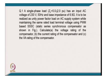
[FL] starting first numerical a single phase load of 5.0 minus 2.0 per unit has a input AC voltage up to 30 volt, 50 Hertz and a base impedance of 6.9 ohm and it is to be realized as a unity power factor load on AC supply system while maintaining the same rated terminal voltage using the PWM static series synchronous compensator as shown in figure.
