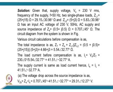
[FL] coming to the solution numerical part of it given that the supply voltage V s of 230 volt RMS frequency of supply 50 Hertz and two single phase load Z L1 equal to 25 plus j 15 ohm and Z L2 5 plus j 3 ohm and AC voltage of 230 volt and we can find out typically the Z s given here.
