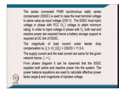
[FL] is then the series connected PWM synchronous static series compensator is used to raise the load terminal voltage to the same as the input voltage of 230 volt and SSSC must inject the voltage in phase with the PCC voltage to attain the minimum rating and in order to inject voltage in phase with the V s dash both real and reactive power are required. Hence, the battery supported storage support is required at the DC link of the SSC.
