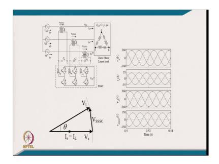
Typically you can call it here I mean we are keeping a here typically the compensator in series to regulate the voltage across this lagging power factor load and these are the typical waveform. [FL] what we have to do? By putting here by injecting the voltage we are maintaining same as the load voltage this is the same as source voltage. Even under the typically kind of voltage.
