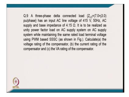
[FL] coming to 9th example: A three phase delta connected load of Z LD equal to 7.0 plus j 3 0 per phase has a input line voltage of 415 volt 50 Hertz AC supply and base impedance of 4.15 ohm. And it to be realized as a unity power factor load on the AC supply system on the while maintaining the same rated terminal voltage using a PWM series compensator. Calculate the voltage rating of the compensator, current rating of the compensator and VA rating of the compensator.
