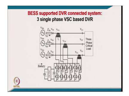
Or, or you can have a 3 single phase one. [FL], you can have a very independent control and this (Refer Time: 14:36) you can design at quite different voltage low voltage also. And accordingly you can select the battery voltage with dc-dc converter like I mean or so. [FL], this becomes very interesting configuration for practical application.
