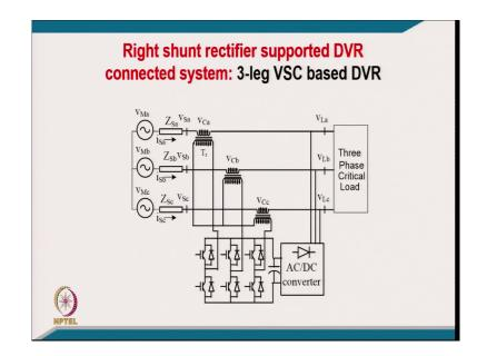
And then this is that if you put the rectifier on load side, I mean like you can have a I mean the rectifier support during this case. Well, this sometime the some of the topology get even the dc link can be of the load that we will talk a little later in some of the maybe series active filter or so, [FL] it can be the rectifier on the left side with the 3-leg, or it can be with the 2-leg rectifiers on the right side.
