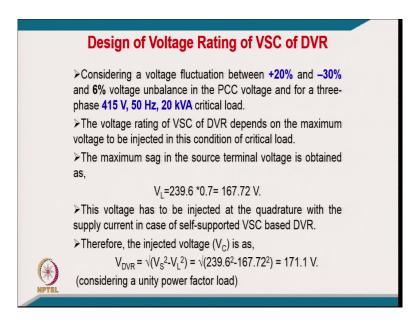
[FL], coming to the design of voltage rating of the voltage source converter. [FL], considering a voltage fluctuations between plus 20 percent and minus 30 percent, and a 6 percent voltage unbalance in the PCC voltage for a three-phase 415 volt 50 hertz to 2 kVA 20 kVA load for which we are designing critical load for which we are designing these DVR.
