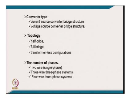
I mean we classified first on the converter types I mean [FL] we can use of course, in current source converter with the bridge structure or we can use the voltage source converter bridge structure that is about converter based classification. The another classification we give like a topology based classification like half-bridge, like a full bridge, the transformer-less configuration.
