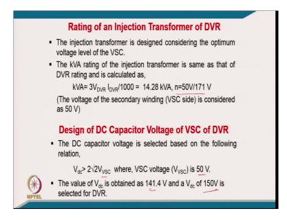
[FL], rating of injection transformer, I mean the injection transformer design considering the optimum voltage of the voltage source converter, and kVA rating of the injection transformer is same as that of DVR rating which is calculated earlier 3 V DVR by 1000 [FL] 14.28 kVA.
