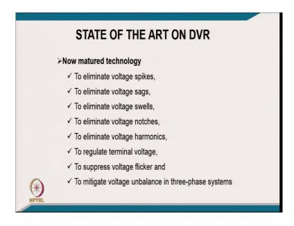
[FL], coming to that on a state of art on this DVR or series compensator active series compensator, now it is a matured technology to eliminate the voltage spike, to eliminate voltage sag, to eliminate the voltage swell, to eliminate voltage notches, to eliminate voltage harmonic, to regulate the thermal voltage, to suppress the voltage flicker, and to mitigate the voltage unbalance in three-phase system like.
