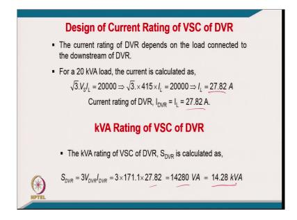
And the current rating of DVR depends on the load connected to downstream of the DVR or you can call it current rating of DVR is same as the load current rating. [FL], we have a 20 kVA load and current can be calculated from this relation root three V S I L.
