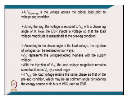
[FL], a pre sag is the voltage across a critical load prior to voltage sag condition. [FL], during the sag, the voltage is reduced to V S that is virtually you can call it like a typically this one, it reduced to this one. Earlier it was typically this, this one I mean we call it pre sag, this is the load voltage.
