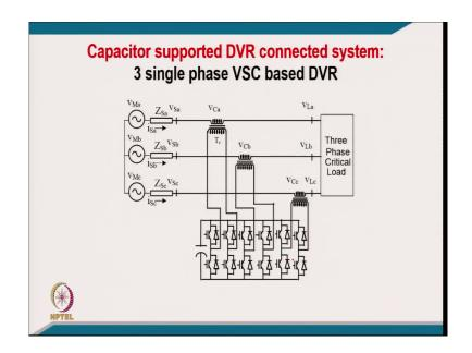
And then 3-leg VSC with the capacitor supported. [FL], this is quite versatile and can be a designed at low voltage. And you can inject it with the self supporting dc bus of this 3 single phase typically of DVR or series compensator.
