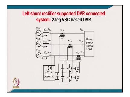
[FL], another one typically is with the 2-leg that was with the 3-leg with the rectifier supported. And this is really 3 single phase with rectifier supported.
