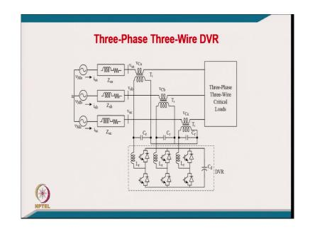
[FL], coming to again the another configuration is basically for three-phase four wire DVR, we have a supply and we have a source impedance. [FL] We have and the this is a three-phase critical load where we want a good quality of voltage with balance voltage sinusoidal voltage regulatory voltage.
