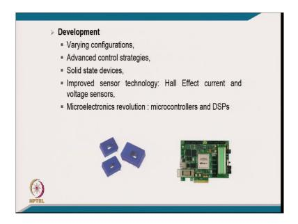
Well, development on this of series compensator have been in varying configuration with the advanced control technique and different solid state devices are used in that. And of course, responsible is improved sensor technology like Hall Effect current sensor, voltage sensor which are now at reasonable cost, but they are very fast and they does they do not distort the signal also.
