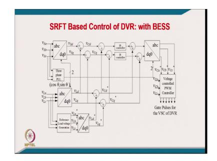
[FL], these typically the you can call it the synchronous reference frame theory based control algorithm of DVR with battery support with DVR. [FL], what I mean if we look into this algorithm, the very purpose of DVR to regulate the voltage across the load. [FL], here we have a source voltage we are sensing and from PLL of this, we are getting either PLL or we can take a template.
