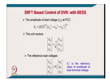
[FL], SRFT based theory typically I mean the equations for if you look into the amplitude, we have to find out the voltage which we like to regulate. We like to calculate the template which we discuss it. And from template and reference voltage, we can find out the reference load voltage like I mean your template required from load voltage only that should be typically the same voltage magnitude required.
