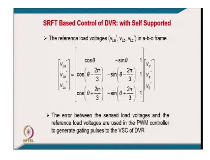
And now we transform this V d, V q, V 0 to directly the load voltage because these are the voltage across the load we require. [FL], we have a instantaneous sinusoidal balance regulated voltage reference voltage, and we sense the load voltage, and we put the load volt on this load voltage PWM current control.
