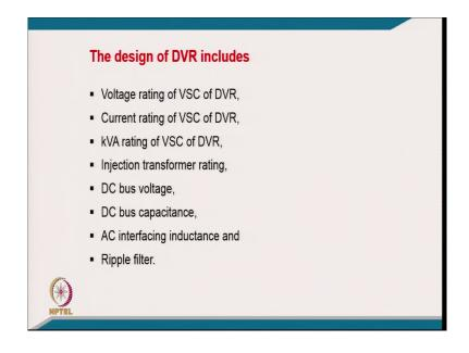
The design of DVR includes the voltage rating of voltage source converter of DVR, current rating of voltage source converter of DVR, and estimation of kVA rating of the voltage source converter of DVR, and the injection transformer rating, then DC bus voltage rating, DC bus capacitance rating, and AC inductor interfacing, and ripple filter rating.
