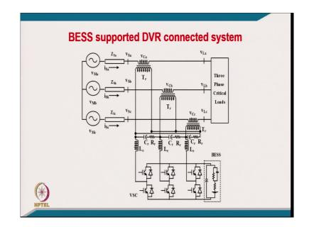
Or another is that you can support directly on the battery of the dc link like I mean BESS supported we can call it. And along with the capacitor here [FL] battery can be charged or can be discharged because for very short period you can take substantial energy also I mean during dynamics because we call it dynamic voltage restorer it means during dynamics also you might have a voltage typically kind of fluctuation sag, swell, or a transient phenomena.
