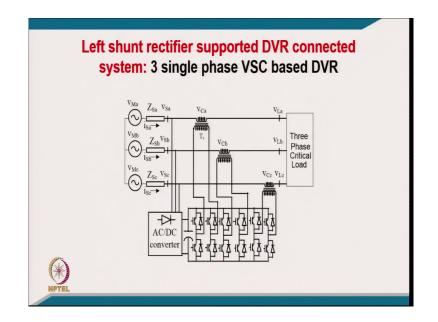
[FL], you have a rectifier supported with 3-leg independent control for all three phase for voltage injection because you may require the separate voltage injection for all three lines separately because the unequal voltage or unbalanced voltage maybe here we would like to balance the voltage across three-phase critical load.
