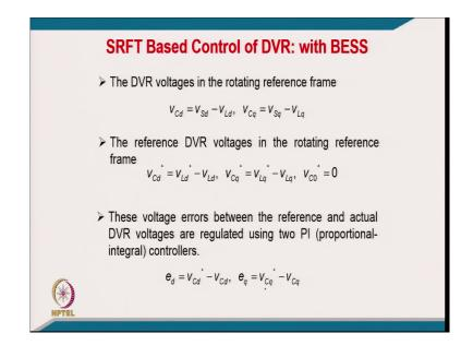
Both are in dq load as well as the source voltage, [FL] we can get a now the difference of this of this dq in compensating one. And from we can find out the even a compensating reference voltage also. [FL] These are actual compensating voltage, these are reference compensated voltage because we have a reference load voltage minus the actual load voltage.
