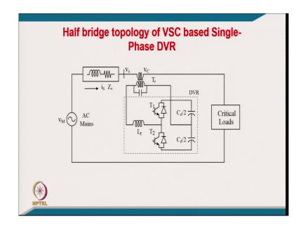
I mean you can just see here if we give a more detail like maybe like a source impedance, [FL] voltage source converter as we discussed that is better [FL], we can use the half bridge ok is a critical load we have to regulate the voltage across this. Whatever the power quality problem of voltage is there, it is supposed to be mitigated by series compensation provided by series voltage there.
