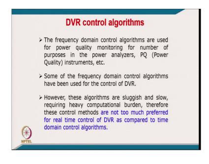
[FL], coming to like a DVR control algorithm. The frequency domain algorithms are used for power quality monitoring and number of purpose in the power analyzer, power quality instruments, etcetera. [FL], some of the frequency domain control algorithm have been used for the control of DVR.
