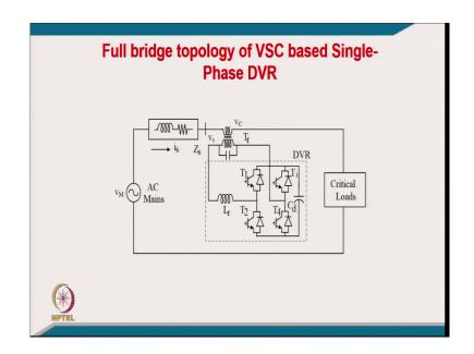
[FL], these are the typical drawback. And because of this reason we prefer to use the voltage source converter typically in a bridge configuration. This is bridge configuration here. And we have to maintain again a voltage here so that PWM operation is satisfactorily here.
