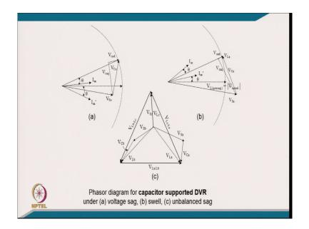
[FL], now coming to very purpose that how typically you can think about the different cases I mean here is the phasor diagram of capacitor supported DVR. [FL], for voltage sag condition I mean this is the typically voltage sag we consider this is the rated voltage, but there have been a sag.
