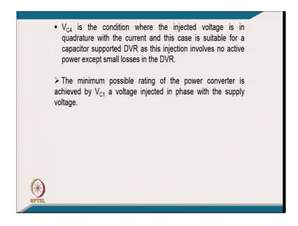
And the V C4 is the condition where the injected voltage is in quadrature with the current and this case is suitable for capacitor supported for a DVR, and this injection involved no active power losses in the DVR. [FL], this is the condition I mean you look into if it is a typically this condition.
