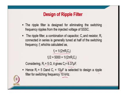
Coming to the design of ripple filter. The ripple filter design for eliminating the switching frequency ripple from the injected voltage of this DVR or series synchronous steady compensator. [FL], ripple filter is a combination of C r and resistance R r connected in series generally tuned at half the switching frequency, f r.
