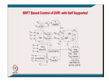
This is of course, typically the again synchronous reference frame theory based control with self-supported dc bus. Of course, we discussed already the self supporting dc bus it means we have to put it. We have to maintain the dc link voltage. Apart from that, the injections should be of voltage preferably at 90 degree because it should need the reactive power only.
