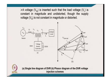
I mean a voltage we injected is inserted such that the load voltage is constant in a magnitude and undistorted, though the supply voltage is not constant and magnitude or maybe distorted. [FL], the very principally we have a source voltage, we have source impedance. This voltage may not be regulated voltage ok.
