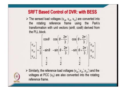
And then from this same way form load voltage using this again the Parks transformation, we can find out even the dq voltage of the load also. And similarly the load voltage reference also from PCC also converted into dq reference frame I mean [FL].
