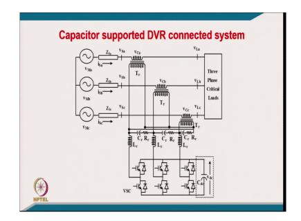
Well, this is like a capacitor supported I mean typically example with the proper component value that you have interfering inductor you have ripple filter. Of course, I told you that if you are using leakage reactance, then this capacitor ripple filter goes across the other secondary side I mean because we cannot put otherwise I mean like on that [FL] that capacitor supported a DVR like I mean.
