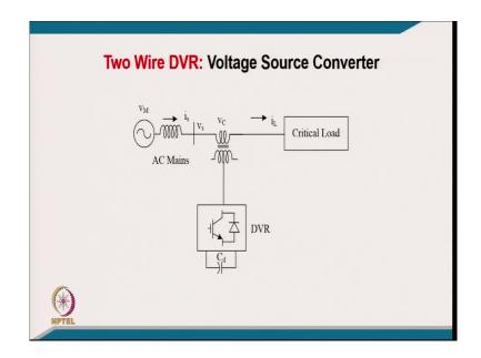
Like it is a single phase I mean two wire DVR with the current source converter we already discussed it across the load. And this is single phase with a voltage source converter I mean DVR.
