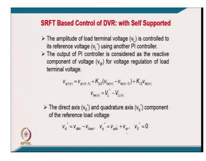
And similarly for regulating the voltage for perform to reactive power for regulation of voltage, we have a load voltage, reference load voltage, we have a reference load voltage amplitude. And we put the PI controller for that that give you the typically the injection of voltage at 90 degree from the current and corresponding reference we get from there.
