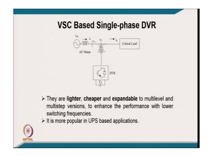
[FL], another structure is like a voltage source converter because here it is shown in brief because we will discuss many structure of this voltage source converter little later. So, we have a supply, and we have a source impedance. And we have a critical load across this we want to keep the voltage even this load may not be drawing a good quality current, but we still need the voltage of good quality across the load regulator voltage.
