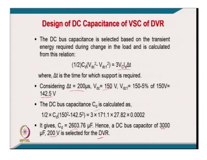
Coming to dc link capacitor of this voltage source converter of DVR with the transformer. [FL], dc link voltage is selected based on the transient energy required during change in the load and is calculated as a half C v half C d in bracket V dc square minus V dc1. And this is the minimum voltage. This is a nominal voltage. And then the energy have to come certainly from 3V c I s into delta t. [FL], delta t is the time for which you require the support required.
