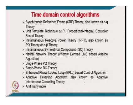
I mean the we already discussed the controlling DSTATCOM, [FL] we can classify the control algorithm on the same basis like time domain control algorithm, like a synchronous reference frame theory, also known as d-q theory, Unit Template Technique or PI Controller based Theory, or Instantaneous Reactive Power Theory also known as PQ theory or alpha beta theory.
