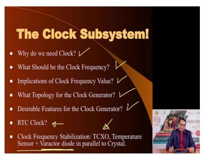
Let us go back to presentation to see what we are talking of. You can stabilized the clock using technique cord TCXO meaning temperature compensated crystal oscillator, this is basically a small enclosure where the temperature of that enclosure is maintained to a fixed value irrespective of the outside ambient temperature and this ensures that the crystal does not drift.
