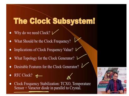
They change the bias voltage on this varactor diode which has been place in parallel to one of the capacitor of the crystals so as to maintain fixed clock frequency. So, these are various methods of having higher accuracy clock frequency signals in application where you require more precise measurement than what would be available with just the cords crystals or with the RC oscillator.
