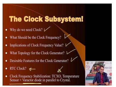
So let's start with the first element of this ecosystem, the clock subsystem. Why do we need a clock? Can we design microcontroller systems without a clock? Most of the time you would have seen that an analogue circuit does not require a clock but a microcontroller is different because it is an example of a digital circuit now digital circuits can be design in two ways what is called as asynchronous sequential circuits and the other type is synchronous sequential circuits.
