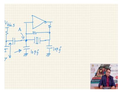
Another method uses a unfortunately this method consumes a lot of power to maintain that temperature, another method uses a temperature sensor and a varactor diode and the way these crystal works the circuit diagram of crystal oscillator is like this that you would have an inverter and you would have big large value of resistor another resistor here and you would have a crystal between these pins and you would have couple of capacitors as I mentioned low value capacitors.
