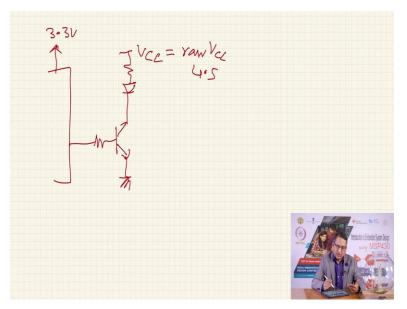
We took the MSP output here and we could have a low side driver as we have already, understand that term and then we could have a LED like this. So, this is the raw voltage raw
