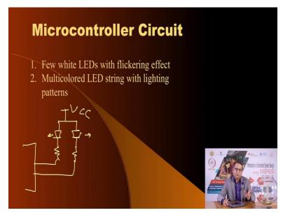
So, it could be something like this one LED here one more LED and then limiting resistor. This is your VCC and this goes to 2 pins of the microcontroller and they were control together with random bits being thrown at both these LEDs. And so what you end up getting is a flickering effect, and once we tested that we were confident that we would be able to control these candles.
