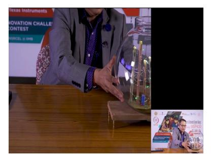
I can remove it and it stops working by because there is no source of power. Let me also take it out of the fishbone to show you the circuit here. Now, I could put it back on top of it and it starts working again why because here is the the receiving coil and in this there is the transmitting coil, I put it on top of it it starts working.
