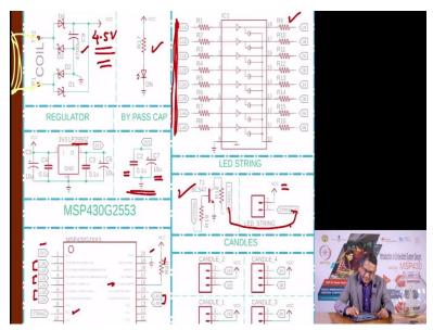
Now we are left with only the mechanism to drive the string of LED's and for that we took another transistor and connected the string here. So, this is the raw supply VCC here is raw supply voltage and the string was connected between this point and this point like this. And a connector has been provided so that you can remove it if you like.
