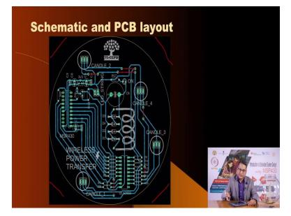
This was implemented like on a single sided PCB. The blue wires indicate tracks and the red bars indicate jumpers. Because the signals have to cross so you bring them up on jumper wires and then put them bring them back in. So, as you see it only uses about 1, 2, 3, 4, 5, 6 jumpers.
