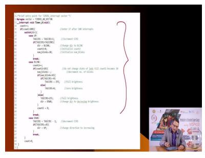
This is the whenever the timer interrupt happens. It goes into it. And in this at some point, it will blink the LED and at some point after sometime it will do PWM on on those LEDs. So, this is the timer code which control that string of LEDs.
