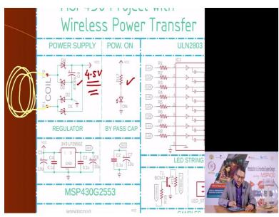
And so let me show you the schematic. So, this is the schematic diagram for this MSP430 based wireless power transfer project. Let us go through all the parts of this schematic. This is the power supply part. So, on this on these two terminals you would be able to collect a coil. Like this here, and then this would generate AC. It would receive the voltage in AC form. And so you are going to have rectifiers. This is the bridge rectifier.
