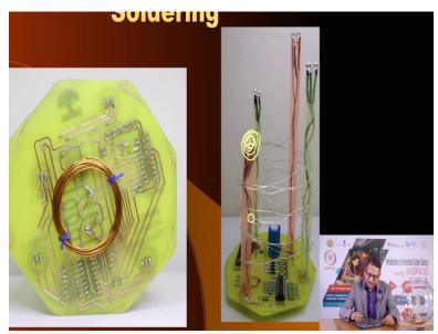
Here is the coil at the bottom. And on the top you would see here is the, this is the top side as you see the top side has been printed with the what what is called as identification layer. So, this PCB actually went through two processes of transferring the layout. The bottom layer was the tracks and the top layer was the the identification layer. So, that we know where each of these components are going to be put and this can be easily done.
