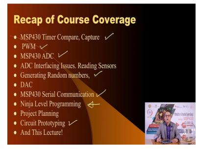
Then we looked at another important feature of a microcontroller and embedded system, which is the mechanism to count time and count events. And for that we looked at the MSP430 timer in the compare and capture mode. Also how we could use the timer for PWM pulse width modulation. Although we also looked at the mechanism to generate pulse width modulation signal using a software code only without the requirement without the implication or without the intervention of a timer.
