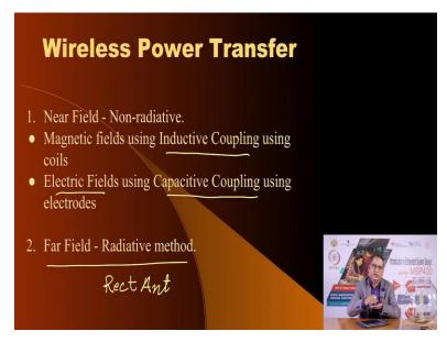
It turns out that wireless power transfers are largely of two categories one is called near field non-radiative. And the second is far field in the near field non radiative method again there are two sub methods one is one uses magnetic field and uses inductive coupling using coils. And the second one is uses electric fields and uses capacitive coupling and for capacity coupling it uses plate's electrodes.
