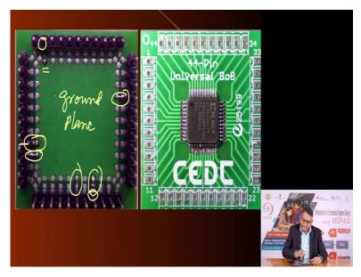
This is the break-out broad, this was fabricated using outside fabrications facilities and on that this is actually a 44 pin Universal BoB which means any 44 pin IC can be sold it onto this and at the bottom appropriate grounds planes this is going to be ground plane, this is ground plane.
