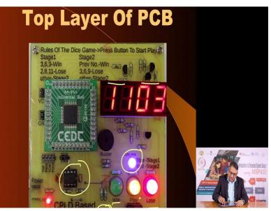
This is the actual implementation. This is the top layer, here are the win, play again, and lose LED, this indicates the stage you are in, this is old number, this is new number, this is the clock generator, this is reset switch, and this is the user switch which you press, these are the rules which the game are mentioned.
