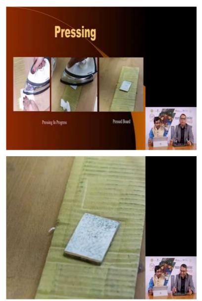
And then use a normal regular home iron for ironing clothes, we use a similar iron about 1000 watts and we firmly press the hot iron on the on the paper. So, that the idea is that the print which is there the laser print gets stuck to the copper. So, you may need some practice but roughly five minutes of intense pressing is required so that the entire paper gets stuck to the PCB.
