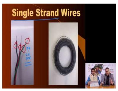
So, what we what you should have is access to single strand wires of such a dimension such gauge and with different insulations. On insulation let me also make a point that the typical insulation that you would get in the market is plastic insulation.
