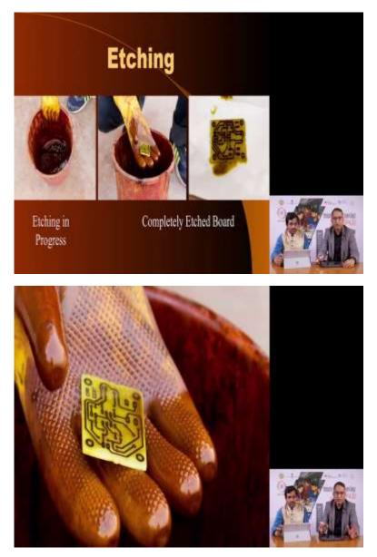
Once you have put it in the etching solution, you have to vigorously agitate the container and this basically will accelerate the reaction. Another method to accelerate the reaction is to increase the temperature of the etching solution and you could use a heater or something like that, but one has to be very careful not to melt the container.
