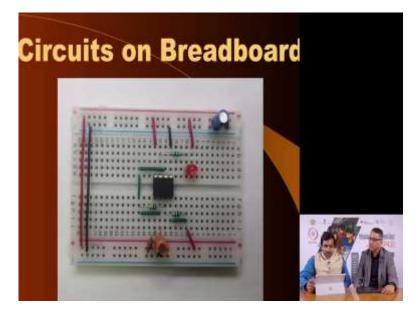
Professor Dr Badri Subudhi: So first method is circuit on breadboard. So you can see a breadboard where the horizontal line in the top are connected together. Similarly the vertical lines are connected together. So, this is a simple example of circuit when one IC is there, few single stranded wires are there, few registers are there, one LED is there and few capacitors are there.
