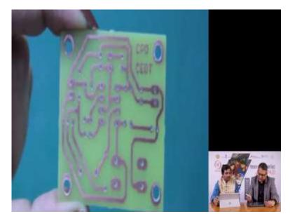
Once they are drilled, this is what the completed PCB looks like and as you can see the copper, the paper underneath the PCB. And you can see that they have been neatly drilled. Now you are ready to go to the next stage which is to refer to the layout, refer to a bill of material which will tell you what should be the value of various components that you must solder. And so you must bring all these things together.
