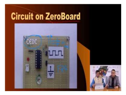
Here you see a PCB, a zero board that we ordered in bulk, which is why it also has a name of my lab, but you can get it in the market very easily of various dimensions. The material of the PCB is very important, this is called FR4 stands for fire resistant type 4 substrate that is the insulating material on which copper tracks or copper pads in this case are pasted.
