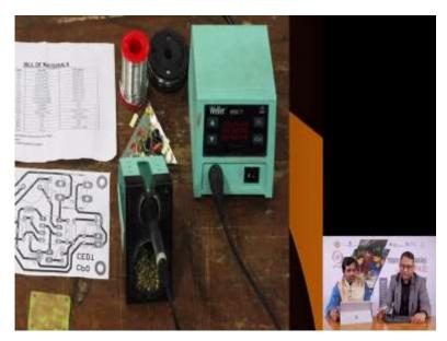
Here it is being shown in the soldering setup. So not only do I have the soldering iron with me, I have the other material which is very important while you are sorting because you do not want to insert the wrong component in some hole, only to have to de-solder it. So it is better to take preventive measures, make sure that you are sure that this is the component to be soldered in given holes.
