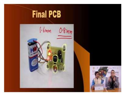
And once you do that, you are left with a beautiful PCB where all the components have been inserted rightly as you see here, the resistors have been nicely bent at 90 degrees so that they are easily inserted in the given holes. Here is a LED, it is powered with a battery, here is a
