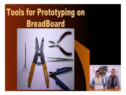
Professor Dr. Badri Subudhi: So you may need a few tools for prototyping on breadboard. So you can see few examples of prototyping breadboard tools. So first one is you can see on the screen is a couple of single stranded wires, the second one you can see is a wire clipper, the third one you can see is a nose plier.
