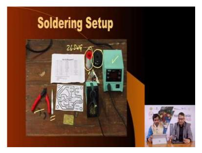
Here is a cutter, 3once we insert the component in the holes, we have soldered it we need to cut off the unwanted length of the wires for that we need this cutter. This tweezer will be used to bend the components nicely so that they go right into the holes where they are supposed to go so tweezer is meant for that.
