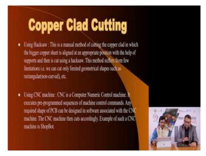
Now, to prepare for the process, you need a copper clad board and you had to cut that copper clad board to be slightly bigger or equal to the dimension, this is the dimension of my PCB that I wish to fabricate and therefore you must make a appropriately sized, you must cut a appropriately sized piece of copper clad board from a larger stock that you may have.
