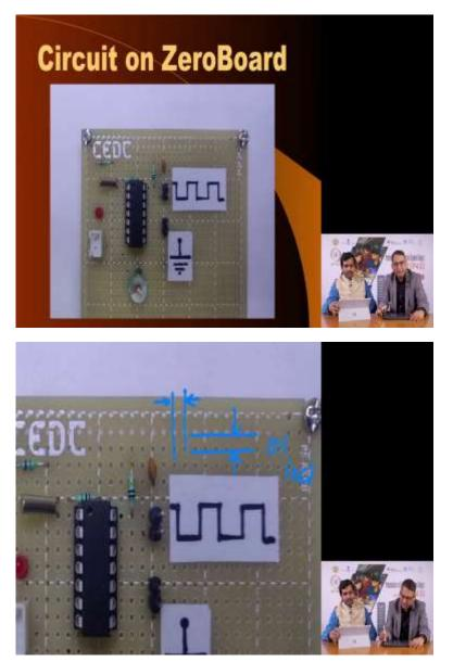
Here is a second example. So breadboard as we mentioned is a good way in fact you have seen the use of breadboard circuits in many of our experiments in the past. Here is a second example of how to prototype a board and that we call a zero board. This is a name we have chosen and it is commonly used.
