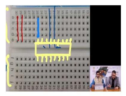
So you see this line is all connected together. Similarly, this line is connected together. And it is suggested that the red line should be plus and the blue line should be minus. It is again a suggestion you are free to utilize those interconnections in any which way you want. Similarly, the horizontal wires, horizontal holes on the bottom line are like that here you have these wires are all, these holes are all interconnected internally.
