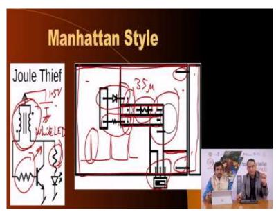
So the supply voltage for such a circuit is a single 1.5 volt battery, I am going to ground it to show 1.5 volt AA or AAA battery you can use, and this is a white LED, this LED is a white LED in this circuit. Now, as we have discussed it earlier white LED cannot be turned on or
