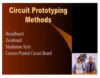
Professor Dr. Badri Subudhi: So there are 4 type of circuit prototyping methods are there, first one is breadboard, second one is zero board, third one is Manhattan style and fourth one is custom printed circuit boards.
