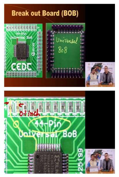
I will explain briefly why we call it universal BOB. The reason is, you see each IC would have its own characteristics, some pin would be connected, would be used for connecting the supply voltage, some maybe input pins, some maybe output pins, and if you have certain pins which are ground and on SMD IC oftentimes multiple pins are available for connecting to the ground.
