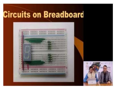
So, the second example you can see there is a 7-segment display is there, which is connected through some wires where the each register is connected with one wire and the LED 7-segment LED display is connected to these wires.
