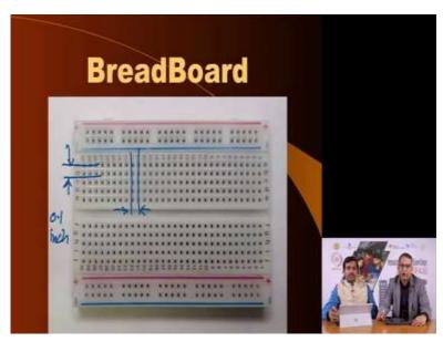
Here is an example of a breadboard, breadboard without any components. And as you see, it has a lot of holes, these holes have a certain pitch, pitch means the distance between two nearest holes. The distance between any two nearest holes here if I say this line and this line, this distance is 0.1 inch.
