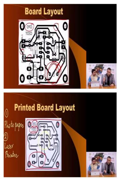
Because here, the references of the components and their names and where they are going to be placed they have been removed, while printing we make sure that we want to print only the layout as well as any text on the copper side of the board that you may want as you see here, I have the holes, the components, this is where IC will go, this is where a switch will go and so on.
