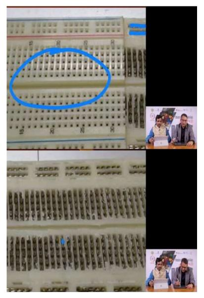
And as you see here, you see these are metal contacts. It is an entire column of contacts. Similarly, you see column of contacts here horizontally. So this is what lies underneath the holes in a plastic insulating form here underneath, this is nothing but rows of copper connections which make connections in the vertical as well as in the horizontal holes.
