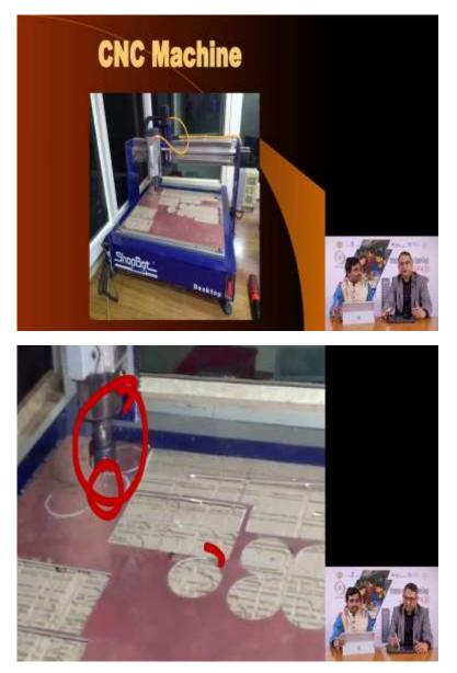
This is by the way, an example or view of a CNC machine that I have in my lab and we use it often to cut as you see here. This is the raw big size copper clad board that has been mounted on the table of the CNC machine and here is the spindle onto which a cutting bit has been installed and it can cut in whatever arbitrary shapes as you see, circular PCBs have been cut so on and so forth.
