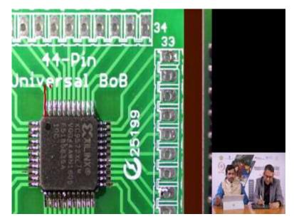
In this case, the distance between these two wires is relatively large for SMD. And there are other SMDs where the pitch of the pins is even narrower. And if that is the situation and in fact increasingly, the integrated circuits that are available these days are being fabricated are being made available only in SMD versions.
