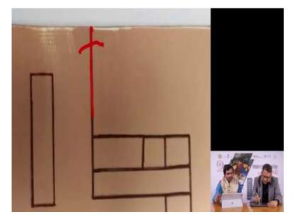
Once you have laid it out, you have to have some practice of laying out layout on piece of paper and then you cut a raw copper clad board of suitable dimension and then using a file, a thin file or you can even use the sharp edge of a knife or sharp edge of forceps to remove the copper. You see this, there is no copper here and so, islands have been created.
