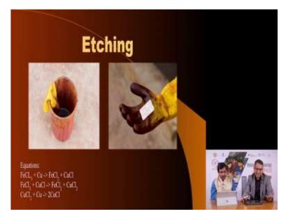
And the most common form of etching process is to use ferric chloride. Ferric chloride may be available in liquid form or you may by crystals and using distilled water, you can create ferric chloride solution. If you have access to a chemical laboratory in your college, they may offer you the best advice.
