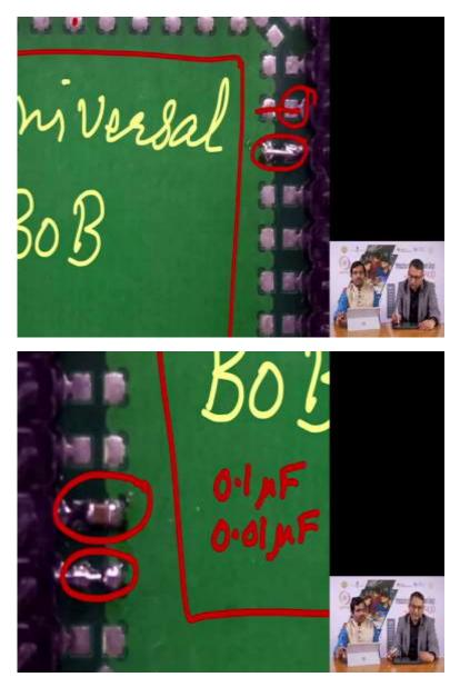
For that we must look underneath the other side of this PCB, you see all these pins have two pads, this is a pad here connected to this pin and here is a pad which is connected to an entire what we call as the ground plane that is this entire green portion is actually copper. Now, if we decide, if we know that this particular IC has say this pin to be grounded, then we will simply short it with a wire as you see here.
