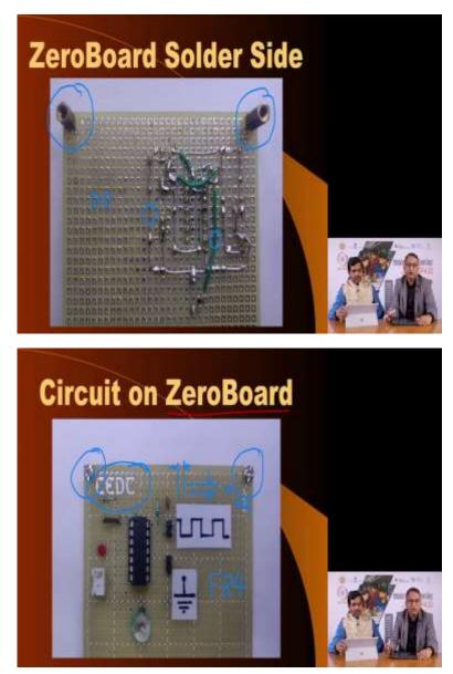
And here you see the circuit has been soldered. And you see this is very important, these are all mounting holes, because at the end of the day this PCB will rest on some surface and if the
