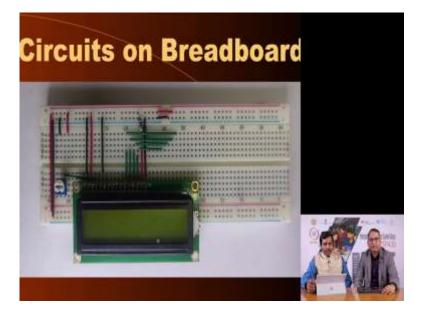
Professor Dhananjay Gadre: So, the third example of a breadboard circuit is as you can see, it has a liquid crystal display LCD. And since the size of the LCD is slightly bigger than the previous two examples as you see here, therefore a larger breadboard is being used. And because it probably uses more connections, you see more number of single strand wires to make connections.
