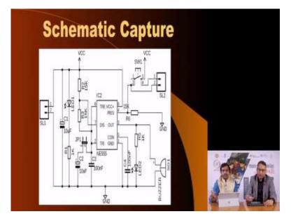
Professor Dhananjay Gadre: So, let us start with the first step. Now to be able to create a circuit board a custom circuit board you definitely need a schematic. Here is an example of a schematic, circuit schematic and as I mentioned in the very first lecture, that it would be helpful if you knew how to use some schematic capture and PCB layout software.
