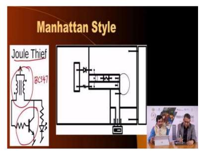
This next style as I mentioned earlier is called the Manhattan style of prototyping. Now, here is an example, here is a simple circuit that we want to prototype, this is popularly called Joule thief, because it is actually a sort of a DC to DC converter. This is basically an oscillator with these two inductors which are coupled with each other and general purpose NPN transistor such as BC547 and the supply voltage here is nothing but a simple (I am going to erase all this).
