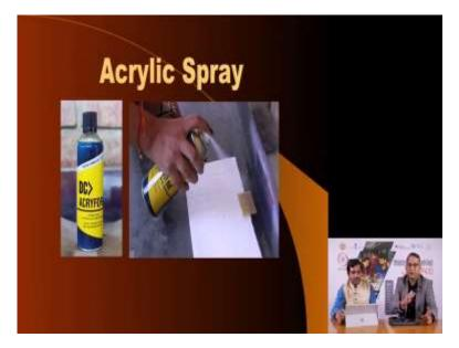
And so what we do is we use an acrylic spray. It is called conformal coating, this is available in many electronics markets, we spray a very thin layer of this acrylic material onto the PCB and in about half an hour's time it dries off and you are left with a beautiful PCB which has been coated with the acrylic material and it protects the copper tracks, now you are ready to drill holes.
