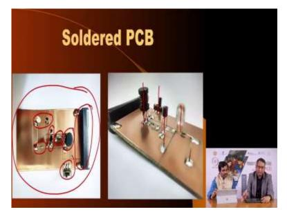
And ofcourse, you need a file what is called as a watchmaker's file, which is a very thin file for removing unwanted copper to create these islands, apart from that, you need a hacksaw to cut a PCB of appropriate dimension. Other than that, no specialized tools are required for prototyping a circuit using this Manhattan style PCB.
