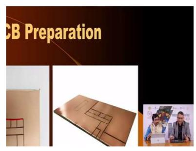
Now, in this particular case we used a single sided board meaning that copper was available only on one side of the PCB, the other side was blank. But use also get such PCBs of the type called double sided PCBs which means, you have copper on both sides. So, you could utilize
