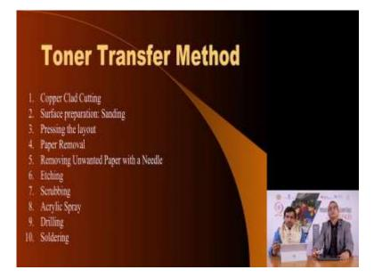
Professor Dr. Badri Subudhi: So first of them, you have to use a toner transfer method, so in toner transfer method, initially copper clad cutting will be there. So, after that sandpaper can be used for sanding the surface for surface preparation then a layout will be placed so it is called as placing the layout.
