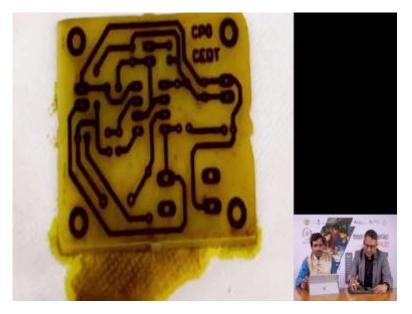
Here is the here is what it looks like. And it has just been placed on a tissue paper so that additional ferric chloride is absorbed.
