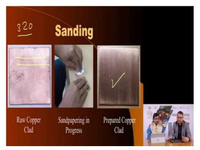
Once you have cut it, then you start scrubbing it, you start using a sandpaper, again sandpaper is available in various types. The grid that is the size of the sand particles which are stuck on the sandpaper is very important because we do not want to scratch the surface, we want to smoothen it.
