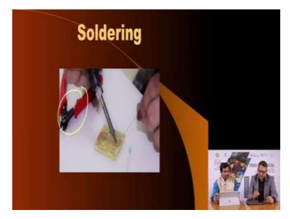
The way to insert soldering components is that you must hold our components with smallest or lower profile first, which means you solder registers and SMD components first, then you can solder IC bases or LEDs. And as the height of the components increase, you should solder them later. Once you have done that, you can snip off extra leads of the components with this cutter as you see here.
