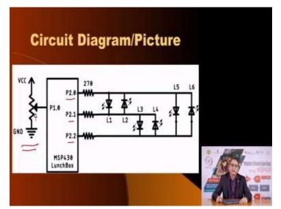
We are going to connect a potentiometer to P1.0 as earlier. But to P2.0, 2.1 and 2.2 we are going to connect 3 LEDs; 3 pins we are going to connect 6 LEDs in the Charlieplexed display fashion. And these displays, these LEDs will be handled in a interrupt subroutine. And we will see how that happens.
