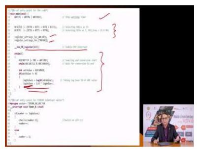
Here is the main code where we have disabled the watchdog timer. We have changed the frequency to about 16 megahertz and we have called the subroutines to program the ADC and the timer, and we also enable the interrupt. Now, why we have enabled the interrupt? Is that when the timer expired, it will generate an interrupt and go into the interrupt subroutine where it will refresh the LEDs and come back.
