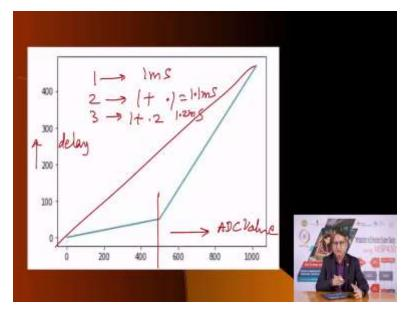
I would like to vary the refresh rate more gently by going from say 250 hertz to 220 hertz to 200 hertz and so on. So, one way would be to apply some non-linearity; some mapping of the ADC values in a non-linear fashion, so that I can have a different amount of delay. And one method could be as illustrated in this graph is that here is on this x-axis is the ADC value. And on the y-axis, you have the delay time.
