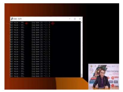
Now when you run this program, you would see that based on this it prints the ADC value, also the log and also the converted value. And you see, as long as whatever the number you can verify that using a calculator what should be the log 10 of this number into 2? Is it matching these numbers here?
