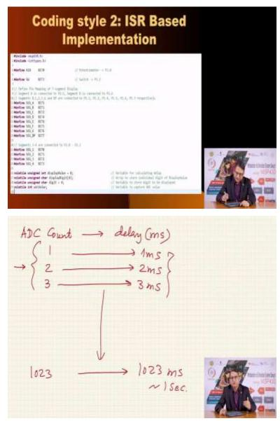
But before that, I want to also talk about that this whole mapping of ADC value directly to a delay value is not a very good idea. And let me explain what I mean by that. We said the ADC count is directly delay time in milliseconds. That means if the ADC count is 1, it means 1 millisecond. If the ADC count is 2, it means 2 milliseconds. If the ADC count is 3, it means 3 milliseconds.
