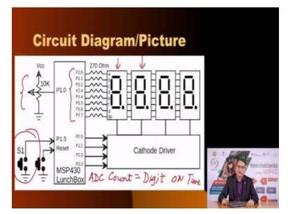
So, what is the objective of our exercise? The objective of our exercises is that we have created a 4-digit display. Now, how do you connect four 7 segment digits to a microcontroller with limited number of pins is that you employ what is called as multiplexing. And so in multiplexing instead of each digit having its own independent seven or eight pins, we are sharing the pins.
