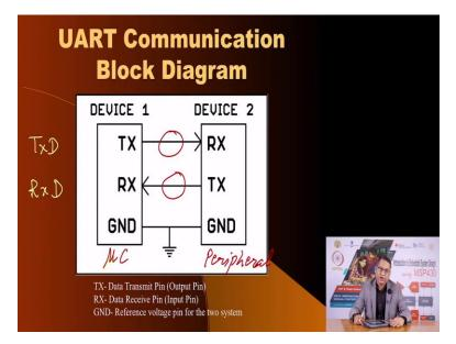
Now, the basic block diagram of communication between two devices is illustrated in this diagram, you have device one and your device two, the two pins of serial communication are called TX or oftentimes they are also called TxD. I could also call this TxD and the other pin for receiving is called RxD.
