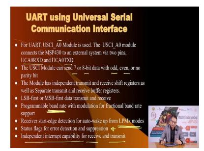
Now for UART, you had to use the A module, A0 module and it uses two pins those two pins will be listed on the microcontroller as RxD and DxD. Of course, these pins are mapped on available port pins, the module can send eight or seven or eight bits of data with odd even or no parity, it has independent transmit and receive shift registers, which is how it is able to communicate in a full duplex fashion.
