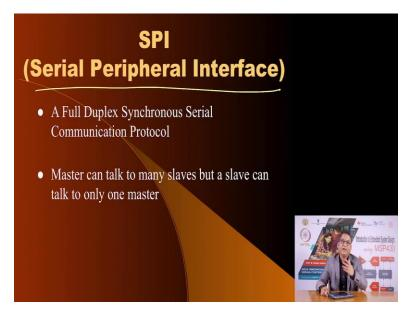
So, this is as far as the UART protocol is concerned. The second protocol that is available on MSP430 is this Serial Peripheral Interface. This is a full duplex synchronous, the previous protocol was asynchronous, which means there was no separate clock that was being sent. But here you have to send a separate clock and you it is a, you can create a network of devices using SPI and you have a master and you can have one slave or multiple slaves and you can have full duplex communication.
