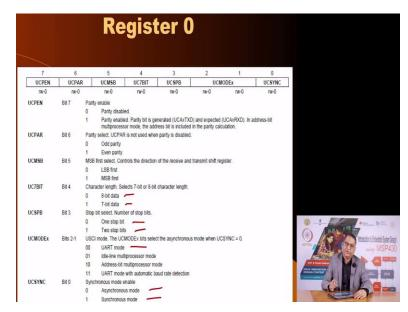
I strongly recommend that you go through these slides to understand the operation of the control register. For example, here you are selecting whether you want the parity to be enabled, do you want the MSB first or the LSB first, what is the size of the data transmission seven bits or eight bits, whether you want a one stop bit or to stop bits, whether you want to operate in the UART mode and so on and whether you are doing synchronous or asynchronous mode of communication.
