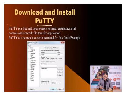
And what do you do, you install a software called PuTTY. PuTTY allows you to select the baud rate and the rest of the data bits and then when you have initialize it
