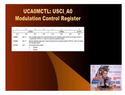
You have the modulation control register, the modulation control register is there, so that the bit rate which is generated by dividing the system clock or whatever clock source you have chosen.
