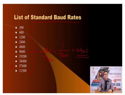
Here is a list of standard baud rates. Now the meaning of standard baud rates means that if you have a existing device, let us say a standard laptop or desktop, which would have offer certain serial communication protocols, it would offer the communication rates which can be from one of these numbers.
