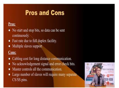
Now the advantages and disadvantages of this protocol are listed here. Since there is no start and stop bits the effective number of bits is, you know does not have that over it. So, your data rate will be higher. You can support multiple slaves. But you cannot use this for long distance communication between two devices and if you have multiple slaves, it will require multiple chip select pins from the master that is the only, you know disadvantage of this method.
