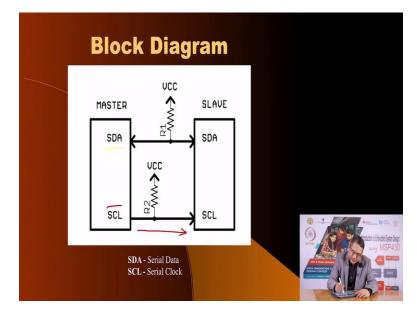
Here is what is required you only have two pins, one is called serial data and the second is called serial clock, The clock starts from the master goes to the slave and the data is bidirectional, you the master starts the communication the slave receives it, and then if required the slave can respond. Now, if you want to have multiple such devices, you can connect them to the same pins in the following way.
