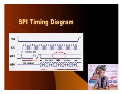
The timing diagram of the various signals that is chip select serial clock, MOSI, MISO is shown here. It starts from the master and then once the master has sent the data here, this is the data being sent by the master the MISO at that time will be in high impedance state and once the data has been transmitted, it may expect the slave to respond back and this is the data received from the slave.
