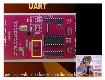
So, first of all this is the jumper settings for programming, for programming download the programming program from the desktop into the microcontroller the jumper settings there are three pins here in this, these two should be shorted. When you are downloading the program. Once the program is downloaded. You have to remove this shorting jumpers and you connect them on this side, on these two sides. Now, your microcontroller is ready to communicate with the PC using UART.
