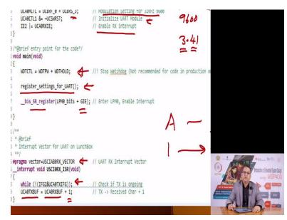
So once the, and then UART is programmed then it just sets the registers in the status registers to status register to enable the global interrupts and when a byte is received it will generate a interrupt vector. Here, we are going to go into the receive vector. In that receive vector, we are waiting, we have received the byte but since we want be increment and transmit it, we want to make sure that the transmit buffer is available.
