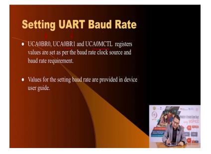
You have baud rate selector there are three register baud rate 0, register baud rate 1 and modulation control registers and the values that these registers must be initialized. The user manual has a useful guide which tells you, if this is your clock source and you want to communicate at certain baud rate what should be the values that you should load into the baud rate register 0, baud rate register 1 and the modulation control registers.
