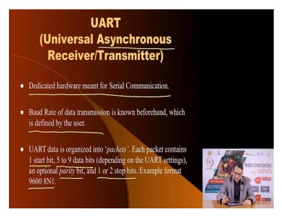
UART uses dedicated hardware and it is communicating in a serial fashion. When you are transmitting data serially, you had to decide what is the duration of each data because each bit. Because we are saying the communication type is asynchronous, which means there is no accompanying clock with the data that is being sent.
