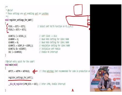
Let us go through that it is a just a single page of code, you have in the main program, all you have done is you have, reset the stop the watchdog timer as we always do and then we are calling a sub routine for setting the UART registers here is that register, in this the P cell 1 and P cell 2 bits are written appropriately, so that you can map the transmit and receive functions on P 1.1 and 1.2.
