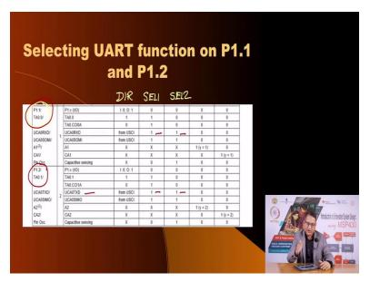
And here is now, as I mentioned, the transmit and receive pins are shared with port pins. In the case of MSP430G2553 the transmitting pin is on, receiving pin is on P1.1, here p1.1 and the transmittal pin here is on P1.2. So you have to, the direction is automatically determined when you write into the USCI register.
