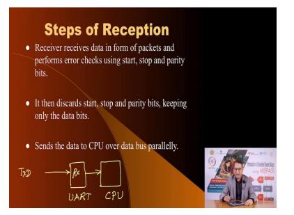
In the case of reception, you reverse the format now the UART is going to receive data from transmitter here, it is going to come in to the Rx pin, Rx pin and this will communicate to the CPU. This is your CPU, this is your UART. The UART will receive the start bit it will start receiving the data bits and then the parity and the stop bit, it will strip off the start bit, parity bet, and stop bit.
