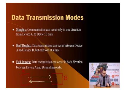
Now, when we communicate between two devices, let me draw them here. For example, if I want to communicate between device A and device B and this could be electronic devices, humans and so on and so forth. Let us say, this is A and B and you want to communicate between them.
