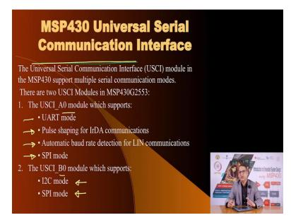
Now, let us look at the serial communication capabilities within MSP430 in the context of these three protocols and we will see how the peripheral, serial communication peripherals on MSP430 allows you to select one of these three protocols and so on. Now, there are two serial communication interface modules in MSP430G2553 that we are using and they are called
