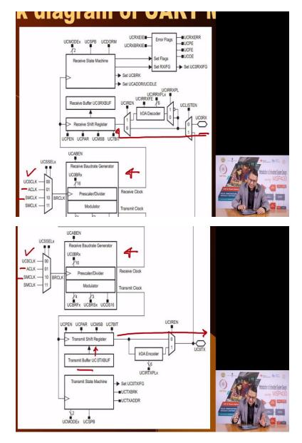
Here is a block diagram. Let this block diagram not intimidate you. I am going to go through that. So, you see the most important part is the part which is the baud rate generator here. It gets, it has a possibility of selecting a source of clock. There is a internal clock generator you could choose or you could choose the a clock, auxiliary clock or you could choose the SM clock, this with the help of certain registers will divide the clock frequency down to get the bit rate clock.
