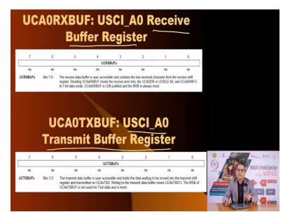
Then these are the receive buffers, here and the transmit buffer transmits so that you can receive and transmit data. These are the two registers in which you are going to write data for transmission and you are going to read that register whenever serial data is received.
