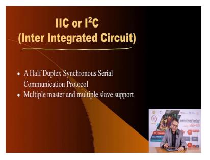
The third method of communication that MSB430 offers is called inter IC communication, as you see here, is called I square C. It is a half duplex communication protocol and you can connect multiple devices multiple slaves to the microcontroller and you can collect up to seven additional devices. That is the beauty of this protocol.
