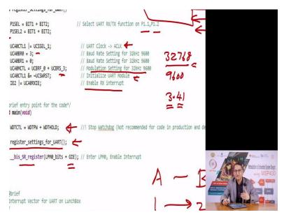
Then you have chosen to use the UART clock from ACLK, in our case ACLK is coming from the low frequency crystal oscillator that is 32768 the bit rate values are stored in these 2 registers value of 3. That is 32768 divided by, 9600. You will get a value of 3.41. So, this 3 you are writing into one of the registers. This 0.41 into 8. The resultant value you write into the modulation, register here.
