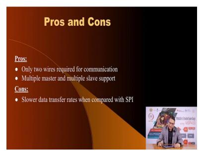
Only two devices to pin two wires are required, so it is a advantage and you can have a master and multiple slaves, but the rate of communication is much lower compared to what you can achieve with the SPI.
