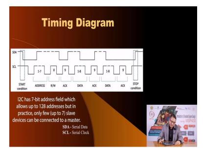
Here is the timing diagram of communication on the I square C bus, you have to initiate a start condition which is when the serial clock pin is high and there is a high to low transition on the SDA bus and then you have certain number of bits and then you end that transmission with a stop conditions in which the clock pin is high and you have a low to high transition on the SDA pin this will terminate that channel that packet of data and the slave can then respond.
