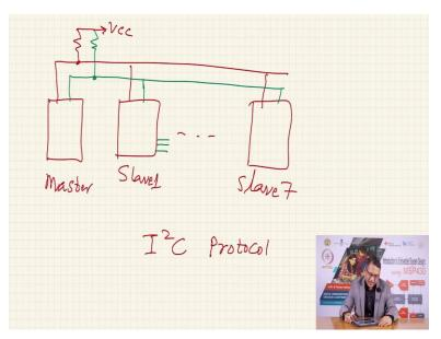
Here is your master, this is your master and we are talking of I square C protocol. You could have slave 1 and up to slaves 7 and using only two wires. Let me draw the second wire with a
