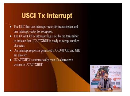
Then once you have, you want to transmit data, you can do that with the help of an interrupt, there is an interrupt vector for transmit which means the moment the output buffer is empty, it will generate an interrupt to the CPU and the CPU can then load a new value into the buffer and there is a flag interrupt flag which tells whether the transmitter is ready and you can also enable and disable this interrupt.
