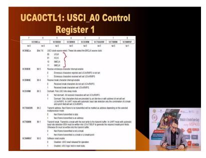
Then the control one register allows you to select what sort of clock source you would like to have and so on.
