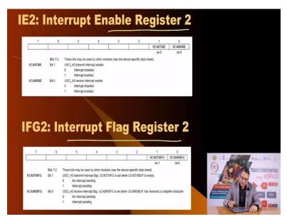
You have the Interrupt enable register 2, and interrupt flag register 2, you can disable or enable those interrupts through these registers.
