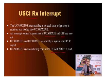
You also have a independent interrupt for the receiver receiving function and whenever the interrupt flag is set, that means a new character is available in the buffer and the CPU can read it.
