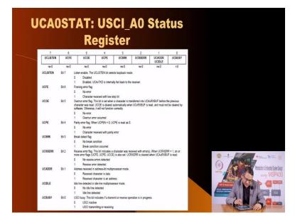
This is the status register. Status register which tells you whether data has been, whether there is a parity error, whether receive any other error on the receiving function and so on.
