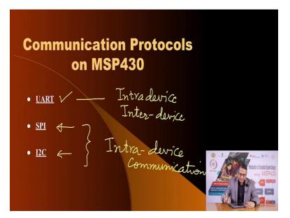
Now on our MSP430 we have several communication protocols, several serial communication protocols and the most common of them is the UART. It stands for universal asynchronous receiver and transmitter. Then we also have a mechanism for higher speed of communication this is called Serial Peripheral Interface and the third method is called I square C, which is inter IC communication.
