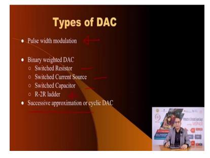
There are various methods, the first method we have already seen using a PWM then you can have DAC made out of resistors and current sources and switch capacitor and resistor using R-2R ladder as well as successive approximation type of DAC.
