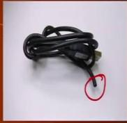
Step1: Cut the end (other than the USB Type A male end) of the cable.
